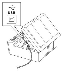
C Carefully guide the USB cable into the cable channel and out the back of the machine. Connect the cable to your Macintosh.
