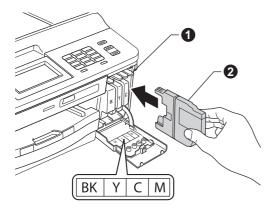
Gently push the back of the ink cartridge marked "PUSH" until it clicks. After all the ink cartridges are installed close the ink cartridge cover.
