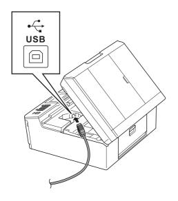
Carefully guide the USB cable into the cable channel and out the back of the machine. Connect the cable to your computer.
