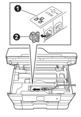
C Carefully guide the network cable into the cable channel and out the back of the machine. Connect the cable to your network.
