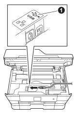
C Carefully guide the USB cable into the cable channel and out the back of the machine. Connect the cable to your computer.
