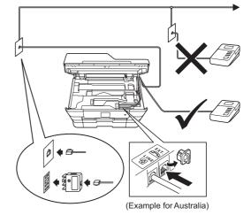
Set the receive mode to External TAD if you have an external answering machine. See Choose a Receive Mode on page 11. Detailed information ➤>Basic User's Guide: Connecting an external TAD (telephone answering device)
