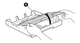
d Gently press and slide the paper length guide 1 to fit the paper size.
