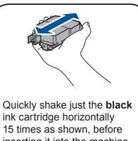
inserting it into the machine.
