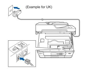
Connect the telephone line cord. Use the socket marked LINE and guide the cord out the back of the machine.
