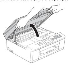
Connect the USB cable to the USB port marked with a etc. symbol. You will find the USB port inside the machine as shown below.
