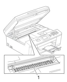
3 Using both hands, grasp the plastic tabs on both sides of the machine and gently close the scanner cover.
