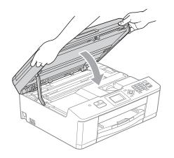
9 Wrap the ink cartridges in the bag, then tape the bag on to the paper tray.
