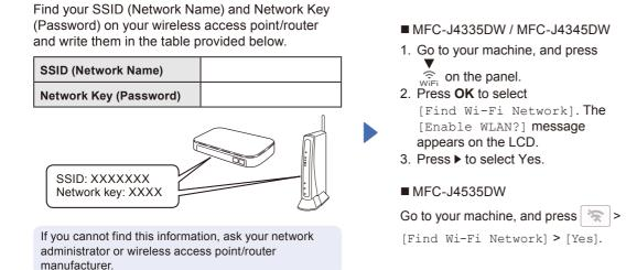
Select the SSID (Network Name) for your access point/ router and enter the Network Key (Password). When the wireless setup is successful, the LCD displays [Connected].
