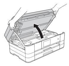
Connect the USB cable to the USB port marked with a symbol ①. You will find the USB port inside the machine on the right, as shown in the callout below.
