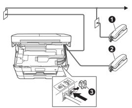
1. Extension telephone 2. External telephone Protective cap
