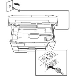
Connect the telephone line cord. Use the jack marked LINE and guide the cord out the back of the machine.
