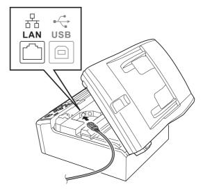
C Carefully route the network cable through the trench and out the back of the machine. Then, connect the cable to your network.
