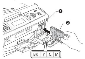
**9** Install each ink cartridge in the direction of the arrow on the label.
