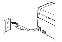
Connect the telephone line cord. Connect one end of the telephone line cord to the jack on the machine marked **LINE** and the other end to a modular wall jack.
