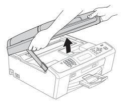
Connect the USB cable to the USB socket marked with a e symbol. You will find the USB socket inside the machine on the right as shown below.
