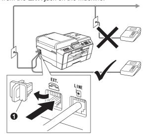
Set the receive mode to External TAD if you have an external answering machine. See Choose the correct Receive Mode on page 9. For additional details, see Connecting an external TAD (telephone answering device) in chapter 6 of the Basic User's Guide.
