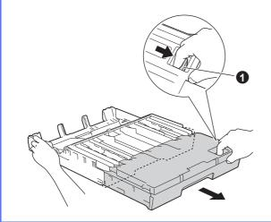
Gently adjust the paper side guides to fit the paper with both hands. Make sure that the paper side guides touch the sides of the paper.
