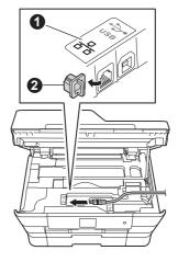
C Carefully guide the network cable into the cable channel and out the back of the machine. Connect the cable to your network.
