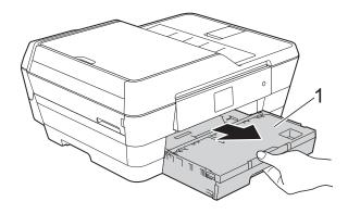
(MFC-J6720DW) Pull the paper tray #1 (1) and then tray #2 (2) completely out of the machine.
