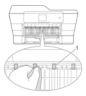
3 Lift the green Jam Clear Flap (2), and then clean the back side of the Paper Feed Rollers (1) with a soft lint-free cloth moistened with water.
