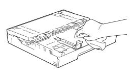
5 Close the output paper tray cover and put the paper tray firmly back in the machine.
