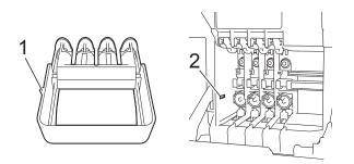
If you cannot find the orange protective part, ship the machine without it. DO NOT install the ink cartridges as an alternative before shipping. 9 Wrap the machine in the bag.
