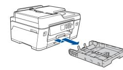
Pull the paper tray completely out of the machine as shown by the arrow.
