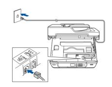
Connect the telephone line cord. Use the jack marked LINE and guide the cord out the back of the machine.
