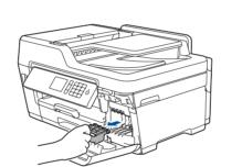
Follow the Touchscreen instructions to unpack and install the ink cartridges. The machine will prepare the ink tube system for printing.
