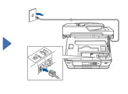
Connect the telephone line cord. Use the jack marked LINE and guide the cord out the back of the machine.
