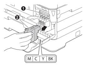
Gently push the back of the ink cartridge marked "PUSH" until it latches. After all the ink cartridges are installed, close the ink cartridge cover.
