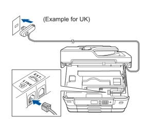
Connect the telephone line cord. Use the socket marked LINE and guide the cord out the back of the machine.
