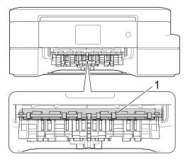
b. Squeeze both levers (1), and then open the Jam Clear Cover at the back of the machine.
