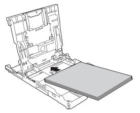
Make sure the paper is flat in the tray and the paper length guide (1) touches the edges of the paper.
