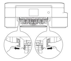
4. Place both hands under the plastic tabs on both sides of the machine to lift the scanner cover (1) into the open position.
