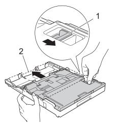
4. Load up to 20 sheets of Photo or Photo L paper in the photo bypass tray with the printing surface **face down**. Loading more than 20 sheets of photo paper may cause paper jams.
