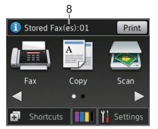
When [Fax Preview] is set to [Off], [Stored Fax(es)] displays how many received faxes are in the machine's memory.
