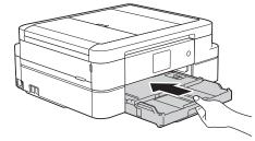
Do not open the paper support and the paper support flap when using the photo bypass tray. Otherwise it is difficult to take out the printouts.
