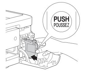
The machine will automatically reset the ink dot counter.
