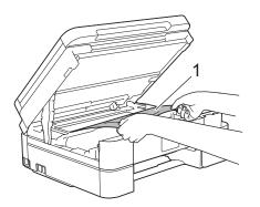
If your LCD error message was [Repeat Jam A Inside/Front], move the print head (if needed) to take out any paper remaining in this area. Make sure scraps of paper are not left in the corners of the machine (1) and (2).
