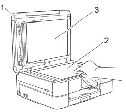
3. In the ADF unit, clean the white bar (1) and the glass strip (2) with a lint-free cloth moistened with a nonflammable glass cleaner. (ADF models only)
