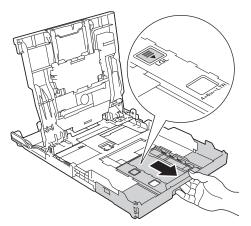
5. Gently press and slide the paper width guides (1) and the paper length guide (2) to fit the paper size.
