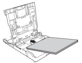
Make sure the paper is flat in the tray and the paper length guide (1) touches the edges of the paper.
