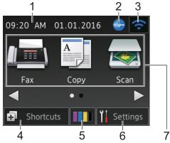
This screen shows the machine's status when the machine is idle. This Home screen is also called the Ready Mode screen. When displayed, this indicates that your machine is Ready for the next command.
