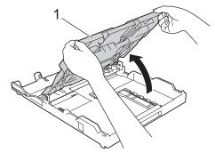
4. Gently press and slide the paper width guides (1) to fit the paper size, and then lift up the stopper (2).
