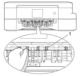
5. Lift the Jam Clear Flap (2), and then clean the back side of the Paper Feed Rollers (1) with a soft lint-free cloth moistened with water. After cleaning, wipe the rollers with a dry, soft lint-free cloth to remove all moisture.
