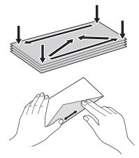
Fan the stack of envelopes well to avoid paper jams and misfeeds.
