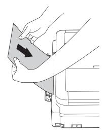
When loading an envelope, or a sheet of thick paper, push the envelope into the manual feed slot until you feel the paper feed rollers grab it.
