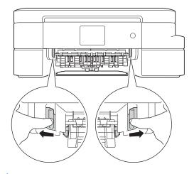
Depending on the paper size, it is easier to remove the jammed paper from the front of the machine rather than from the back of the machine.
