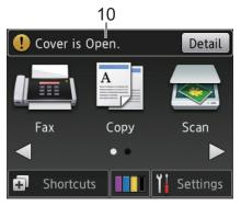
The warning icon (1) appears when there is an error or maintenance message; press [Detail] to view it, and then press X to return to Ready mode.
