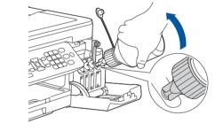
Remove the tip of the ink bottle. Insert the nozzle of the ink bottle firmly so that the ink does not spill. Fill the ink tank by gently squeezing the bottle as shown. Empty the entire bottle into the ink tank.
