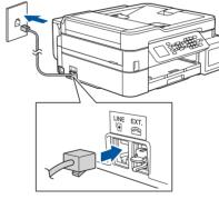
Connect the telephone line cord. Use the jack marked LINE.
