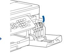
Push down on the cap of the ink tank to close it tightly. Repeat step 4 for the three other ink tanks.
