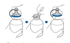
Remove the cap and protective film from the ink bottle, and then replace the cap.
