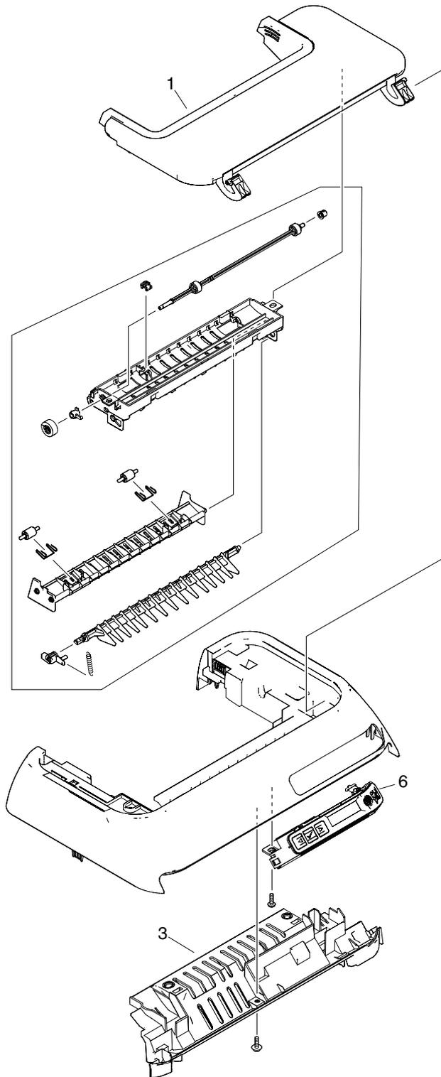
**Figure 7-5** Upper cover assembly - duplex models
