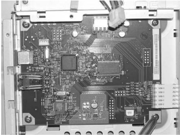
6. Lifting and remove the formatter.
