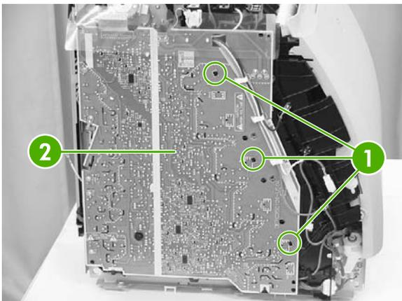
17. Remove two screws (1) and take out the metal plate (2).
