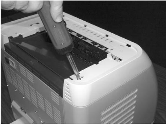
7. Remove one screw from the inside upper cover and then remove the black output guide.
