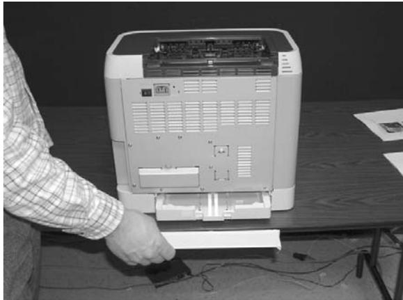
2. Remove nine screws from the rear plate (RC1-5227-020CN).
