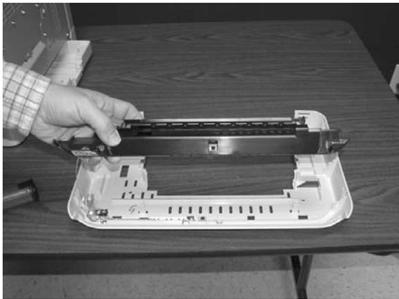
8. Remove two screws from the control panel.
