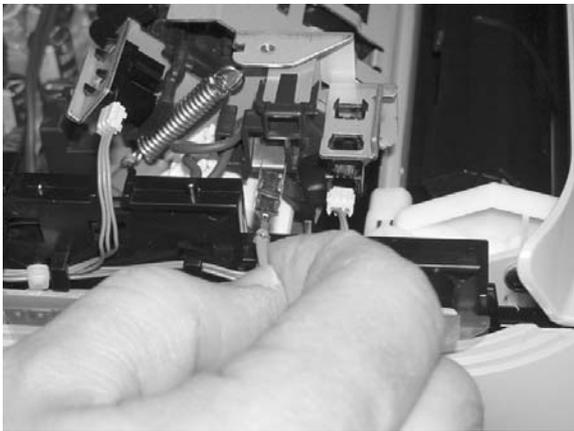
15. Remove the thermistor wire.
