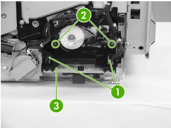
6. Remove two screws (1) and take out the duplexing-driver PCA (2).
