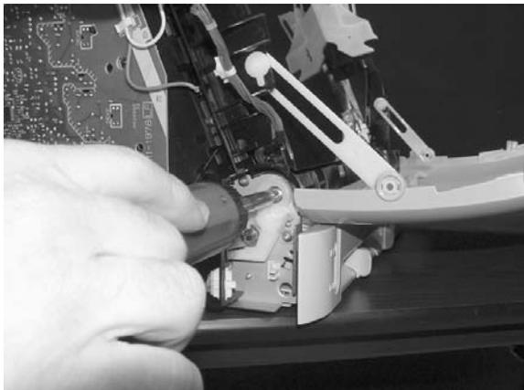
14. Using needle-nose pliers, remove the hinge left cam and the right hinge cam.
