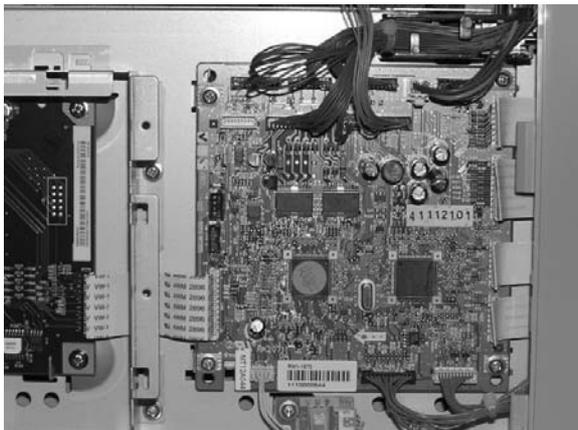
5. Remove four screws from the DC controller.
