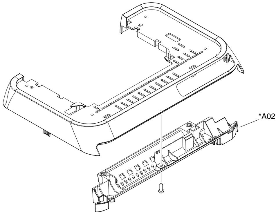
**Figure 7-4** Upper cover assembly - simplex model
