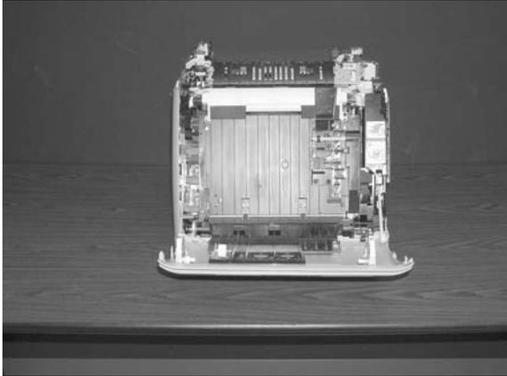
11. Remove the lower screw attaching the inside right cover to the printer.
