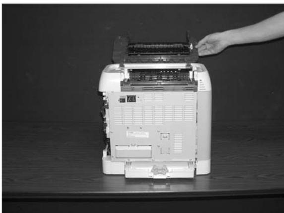
7. Remove the four screws that anchor the upper cover to the printer.
