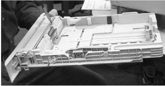
2. Remove two screws that attach the separation assembly.
