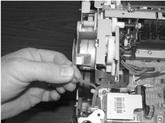
12. Open two clips and remove one clip to remove the fuser connector.
