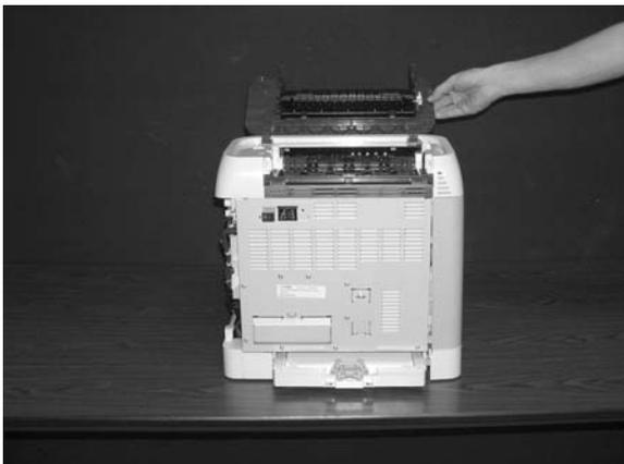
7. Remove the four screws anchoring the upper cover to the printer.
