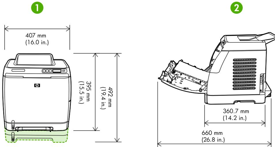
**Figure 2-1** Printer dimensions
