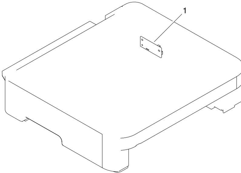
**Figure 7-22** PCA assembly location in optional Tray 3
