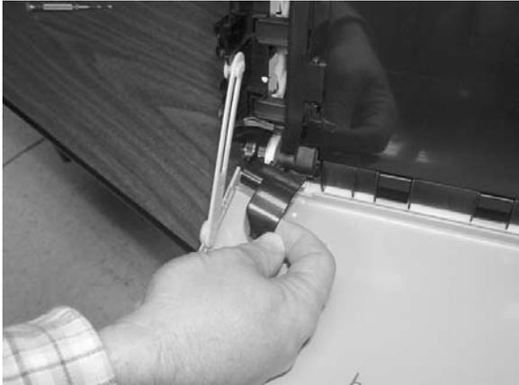
10. Remove one grounding screw from the ETB harness.
