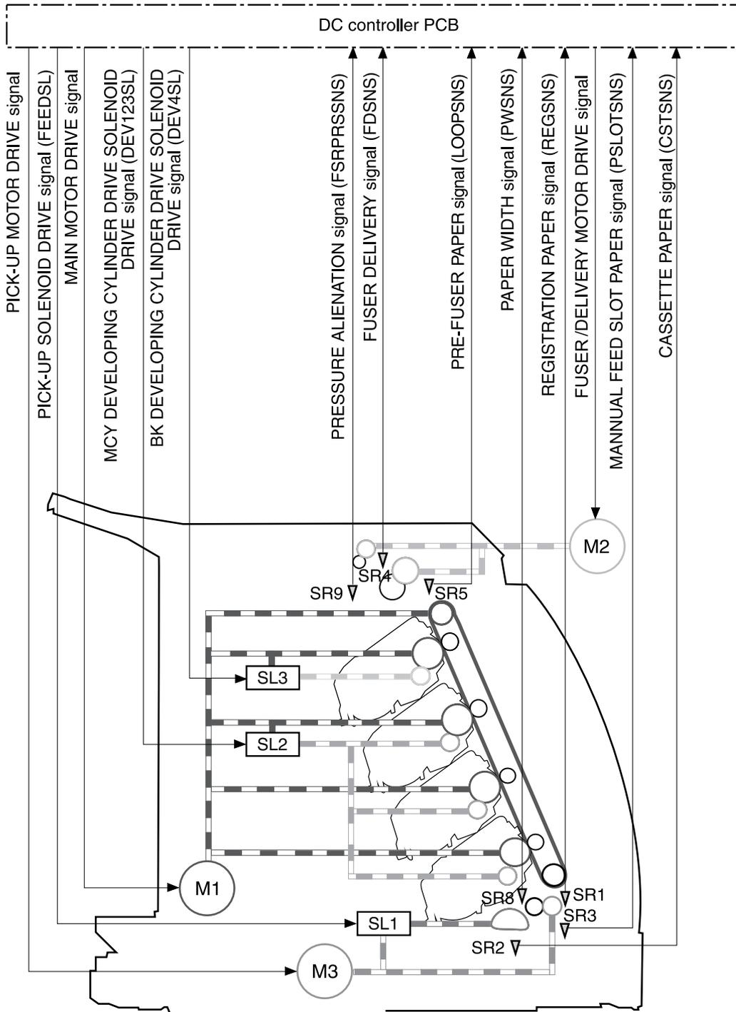
**Figure 4-12** Paper pickup and feed system
