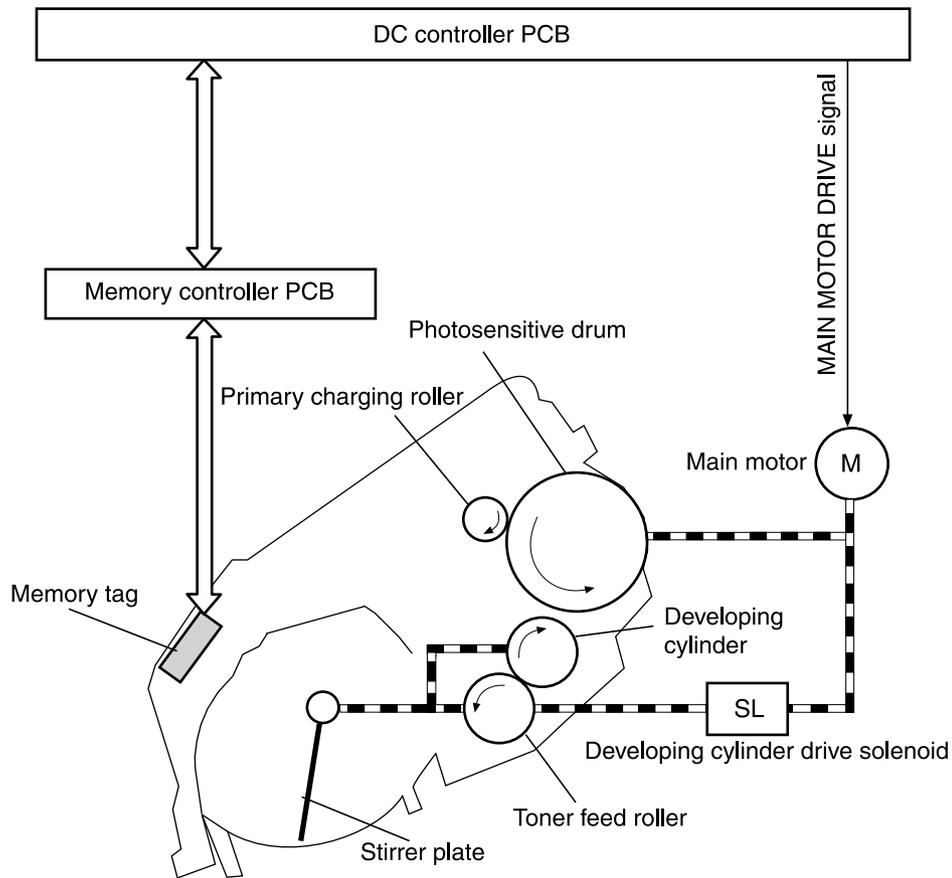
**Figure 4-7** Print cartridge structure
