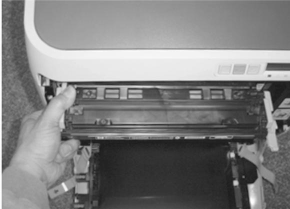
Installing the cartridge at an angle can damage or break the E-label reader guide pin.
