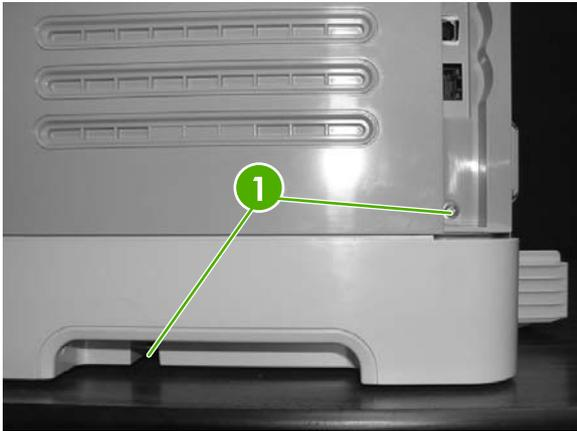
2. Remove the paper-delivery-tray assembly (RM1-1859-000CN).
