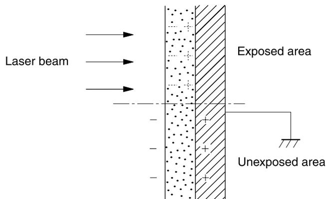
**Figure 4-5** Laser beam exposure
