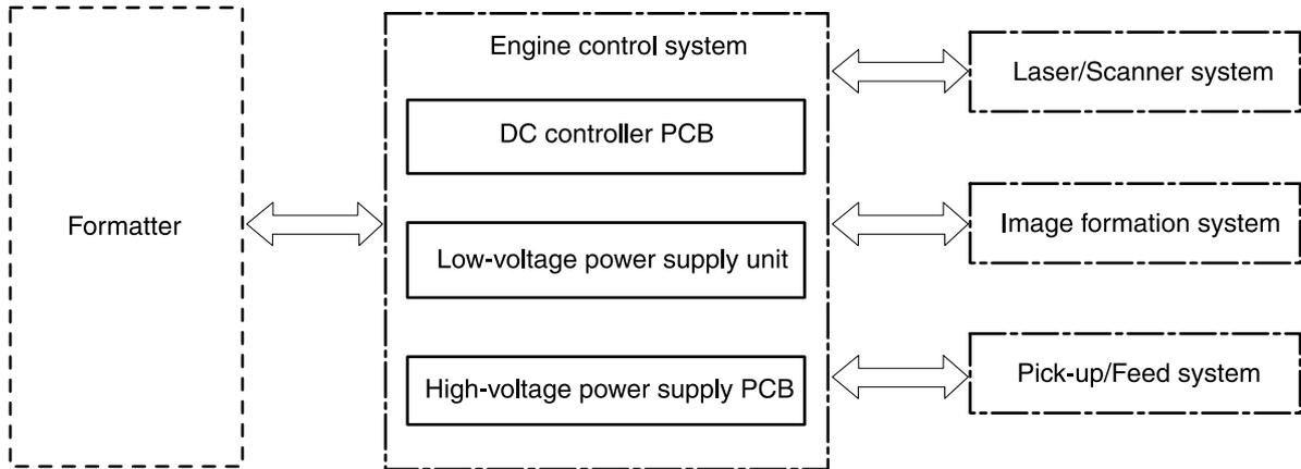
**Figure 4-1** Engine control system
