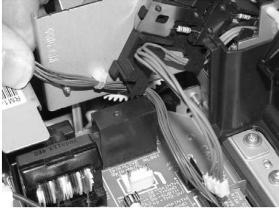
17. Remove three screws from the fuser chassis.
