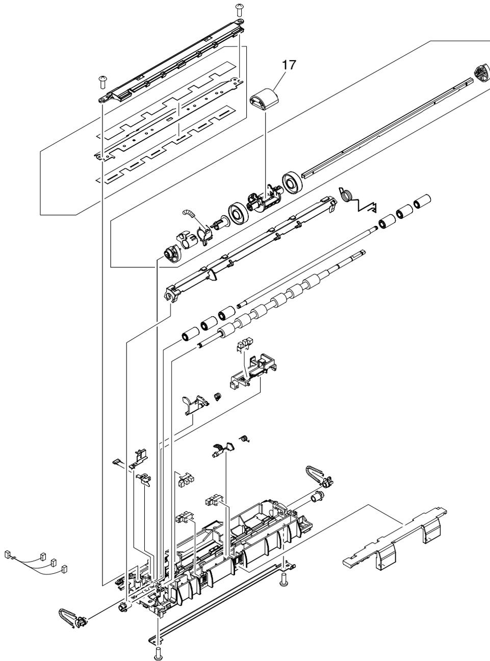
**Figure 7-19** Paper pick-up feeder assembly (Tray 2)
