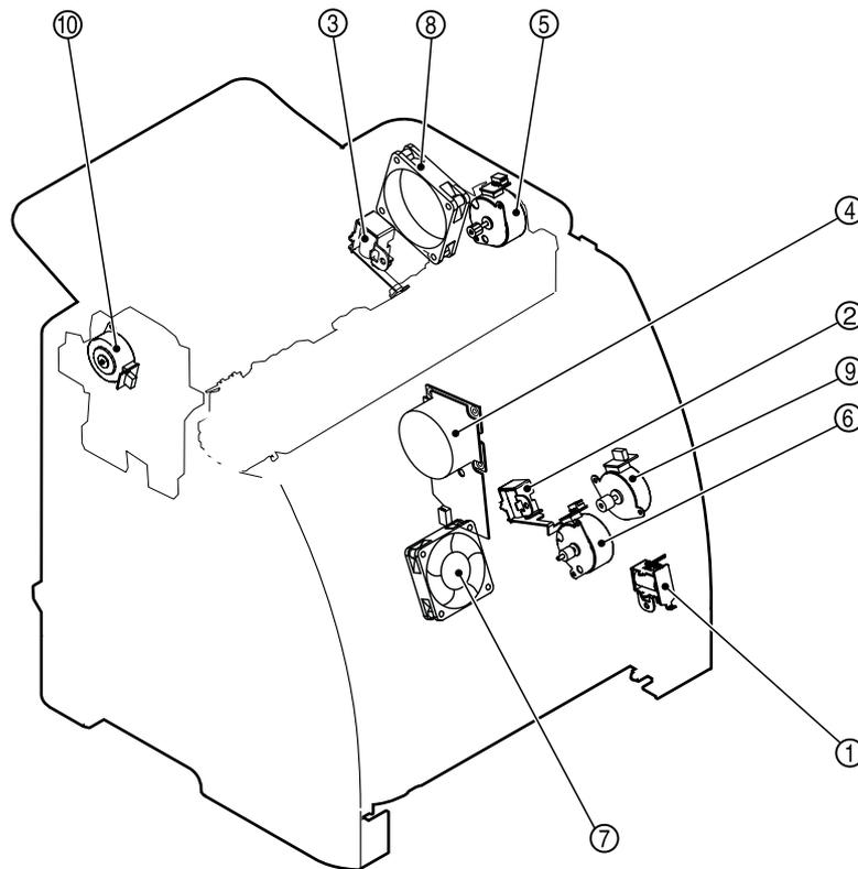
**Figure 4-14** Location of solenoids, motors, and fans
