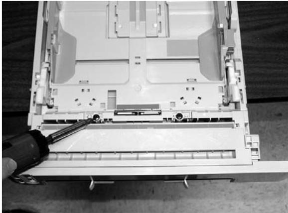
3. Remove the separation assembly (RM1-1922-000CN).
