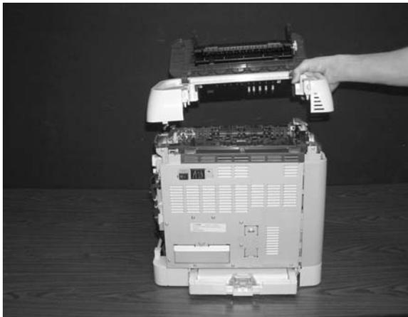
9. Remove the two upper screws attaching the inside right cover to the printer.
