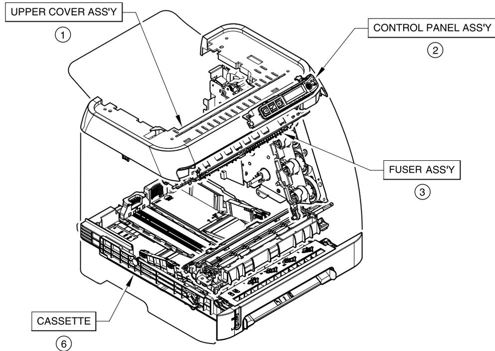
**Figure 7-1** Assembly location diagram - simplex model
