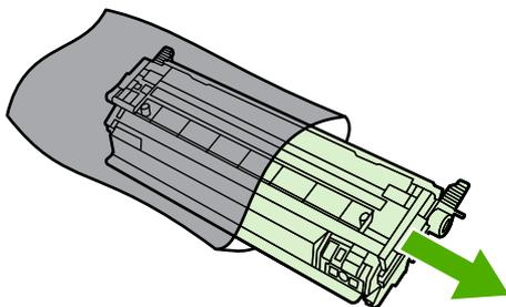
4. Grasp the blue handle on each side of the print cartridge and distribute the toner by gently rocking the print cartridge from back to front.
