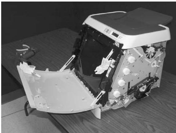
9. Remove the small black cable cover on the left side of the printer by carefully snapping it out of place.
