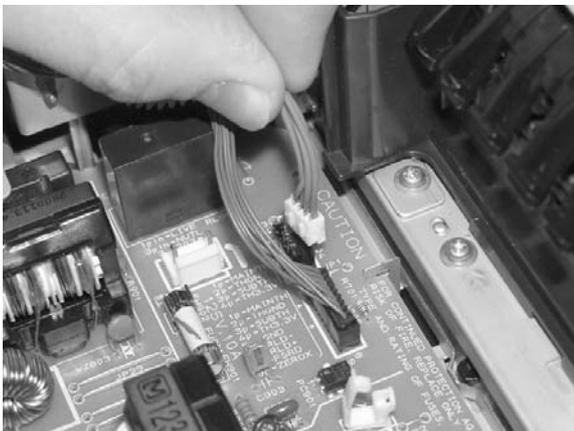
16. Remove the wiring harness.
