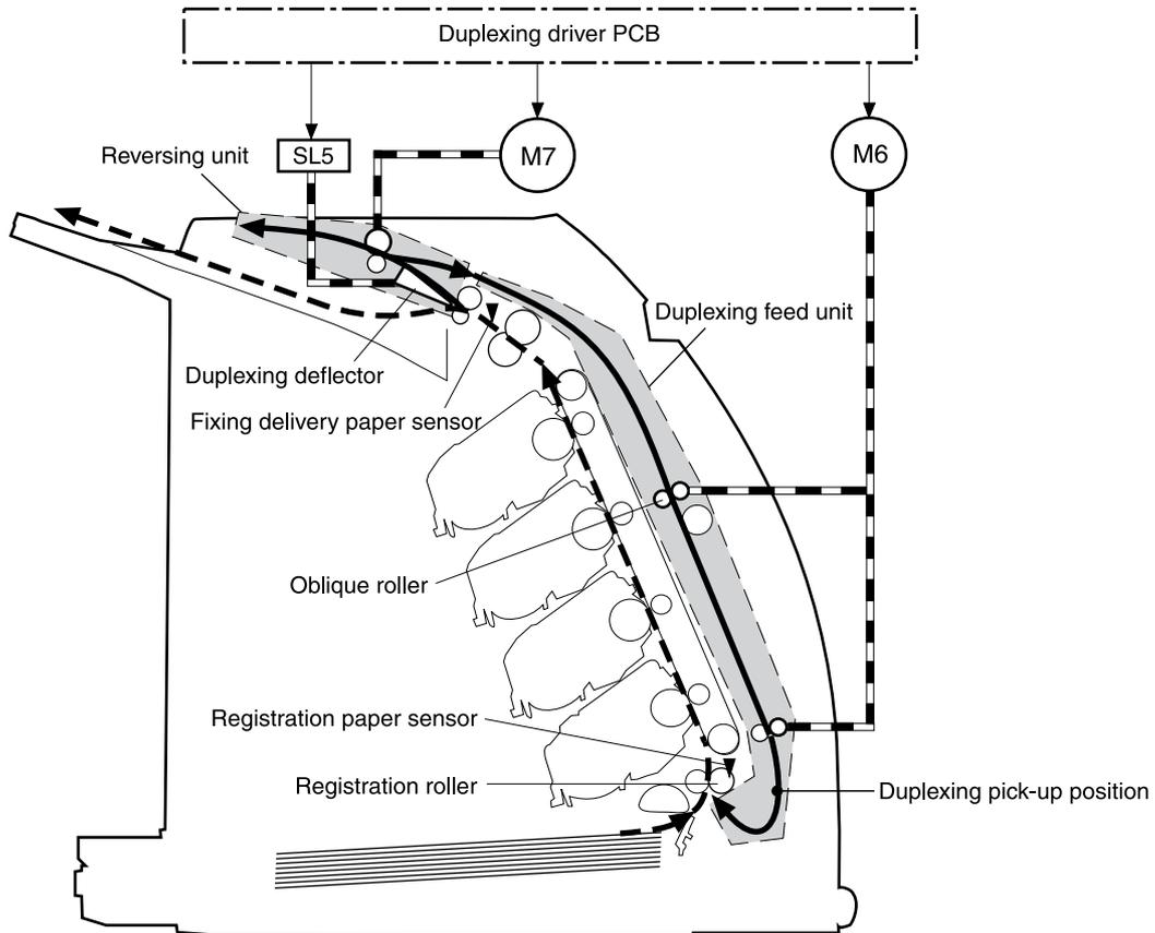
**Figure 4-19** Duplexing components
