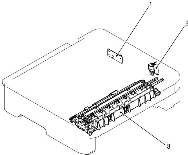
**Figure 4-16** Location of 250-sheet tray solenoid and printed circuit assembly
