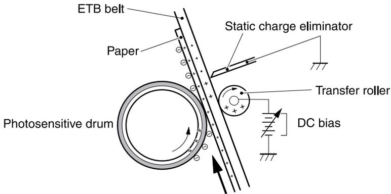
**Figure 4-10** Separation stage
