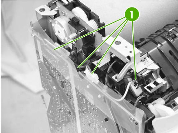
15. Remove the screw with washer (1) and the three tapping screws (2) that anchor the PCA to the printer.
