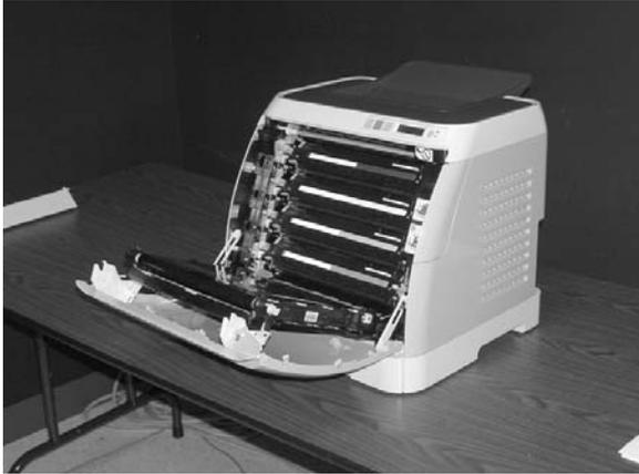
2. Remove the print cartridges.
