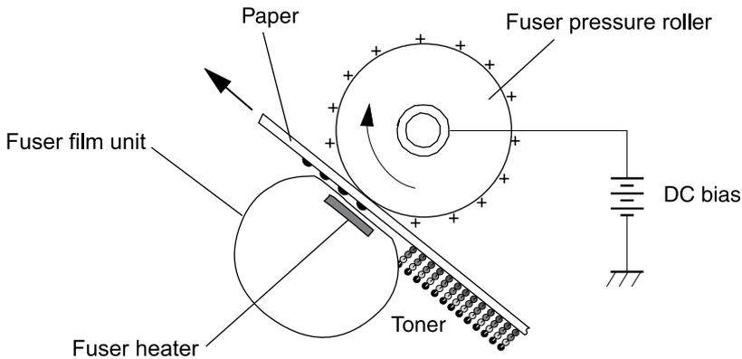
**Figure 4-11** Fusing stage
