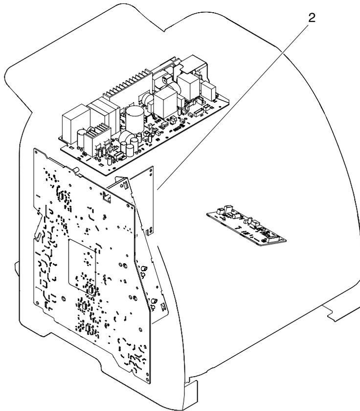
**Figure 7-15** PCA assembly location
