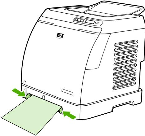
2. Feed print media into Tray 1 with the side to be printed down, and the top, short edge in first. Make sure that the media is inserted far enough into the printer for the paper feed mechanism to grab the media.
