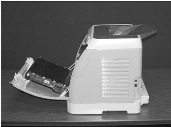
4. Remove the right cover (RM1-1858-000CN), carefully twisting the front edges of the side cover outward.
