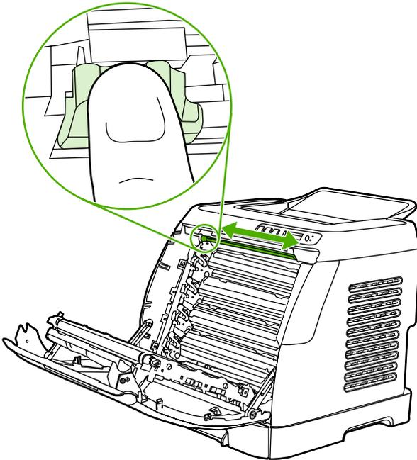
4. Ensure that the cleaning tool is returned to the left when the cleaning is finished.
