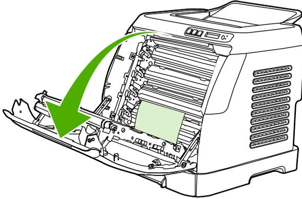
**CAUTION** Do not place anything on the transfer belt, which is located on the inside of the front door. Otherwise, the printer may be damaged, adversely affecting print quality.
