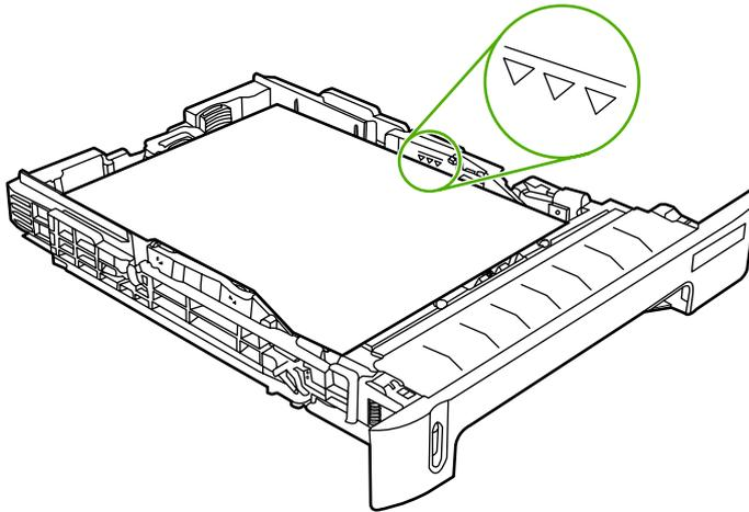
7. Slide the tray into the printer. The back of the tray will protrude from the back of the printer.
