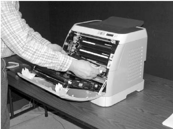
3. Remove the new print cartridge from the bag. Place the used print cartridge in the bag for recycling.
