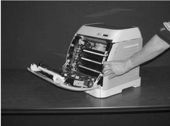
5. Unplug two connectors (1), remove two screws (2), and remove the duplexing-driver unit (3).
