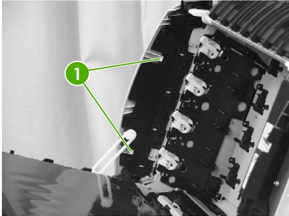
11. Unhook the lowest claw (1) on the front edge of the left cover, and then remove the left cover (2) and left cassette cover (3) together.
