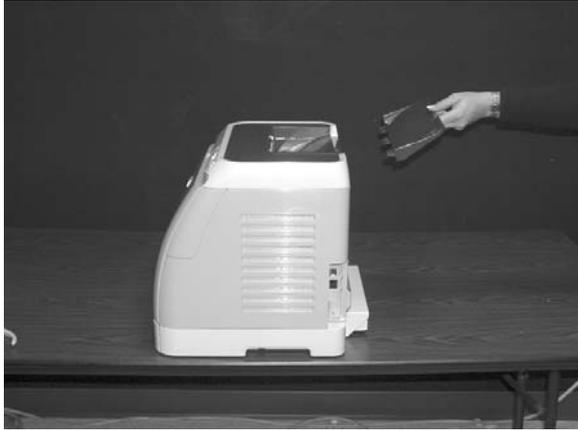
3. Remove the right-cover assembly (RM1-1860-000CN), carefully twisting the front edges of the side covers outward to remove.
