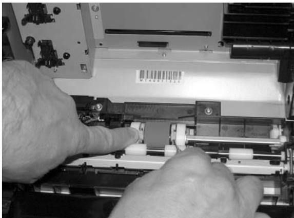
6. Rotate the paper pickup roller (RC1-5440-000CN) toward the back and remove it.
