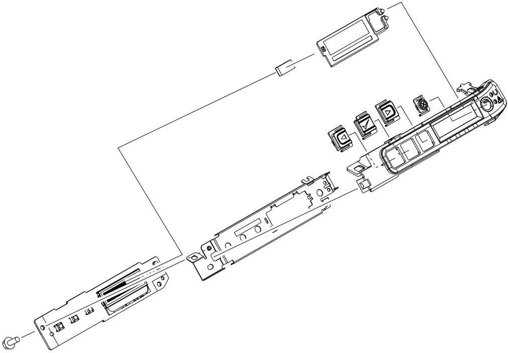
**Figure 7-9** Control panel assembly
