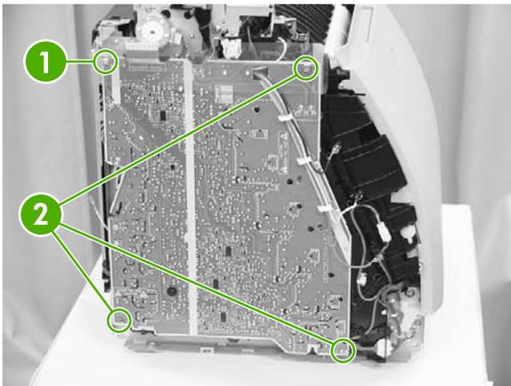
16. Unhook the three claws (1) and remove the high-voltage power supply PCA (2).
