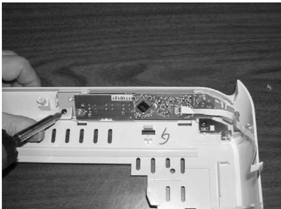
9. Remove the control-panel assembly (RM1-1861-000CN).
