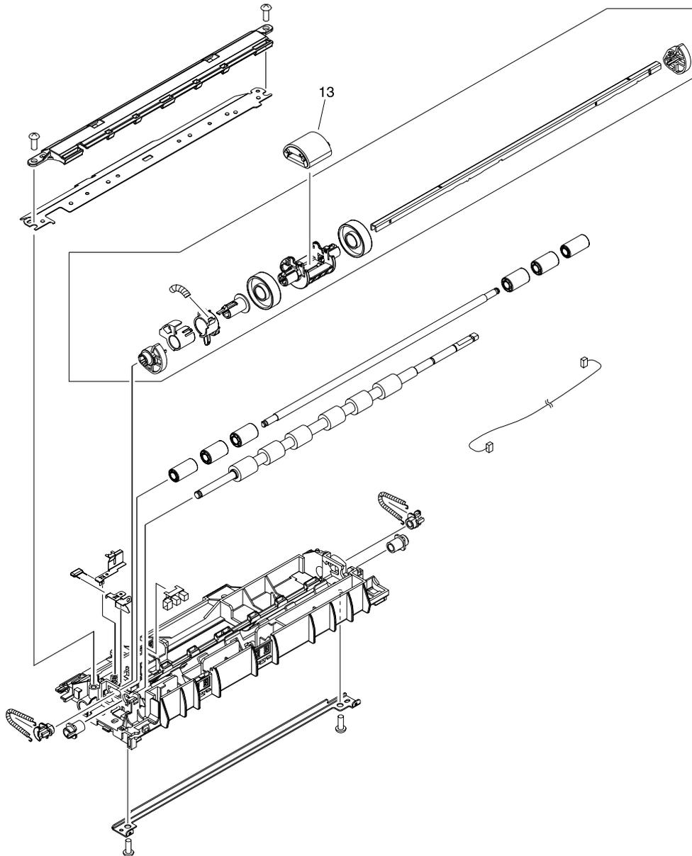
**Figure 7-21** Paper pickup feeder assembly (Tray 3)
