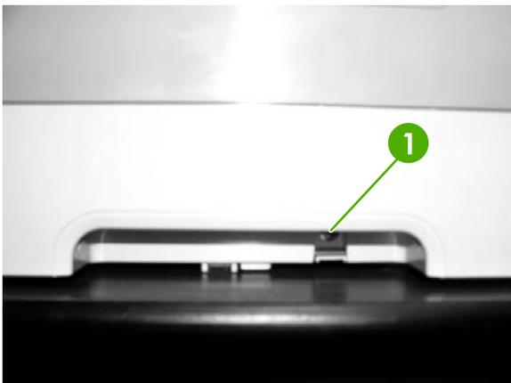
10. Unhook the two upper claws (1) on the front edge of the left cover assembly.
