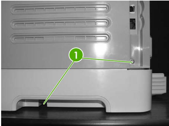
2. Remove the paper-delivery-tray assembly (RM1-1859-000CN).
