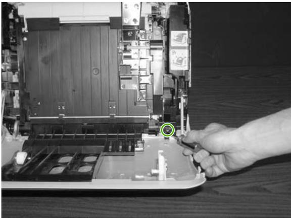
12. Open the ETB approximately a quarter of the way, and then gently remove the inside right cover and let it rest on the back of the front door.
