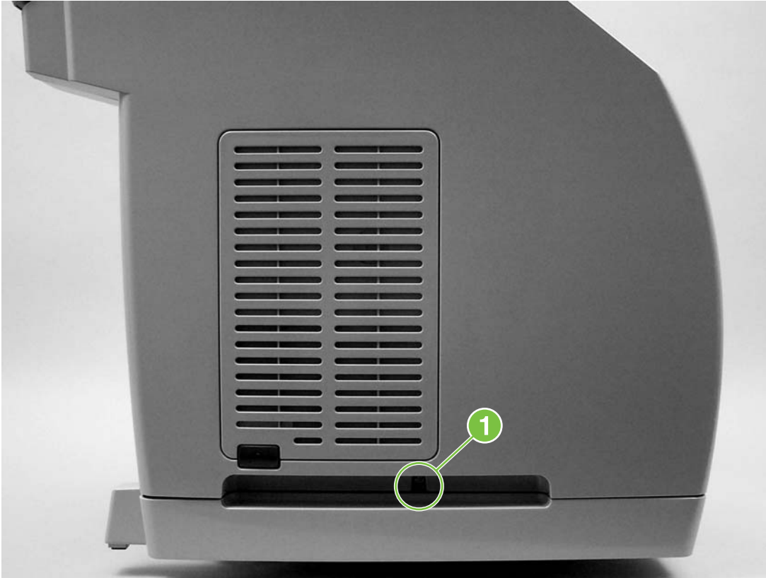
Figure 5-20 Left cover screw
