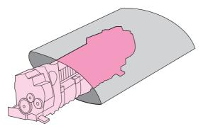
8. Hold the fuser with your thumbs on the blue ridges and fingers on the blue latches. Push both sides of the fuser into the printer.
