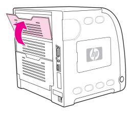
5. If no paper is visible, open the lower rear door (rear output bin).
