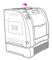
3. Adjust the length guides. For letter-size paper, raise the blue rear stop. For A4-size paper, lower the blue rear stop.
