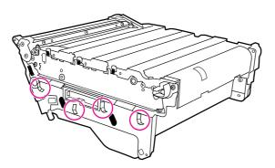
2. Grasp the right blue handle. Press and hold down the blue button. Slightly lift the right side of the transfer unit.
