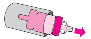
5. Hold the blue side of the pickup roller, and insert the left peg into the round hole in the printer.
