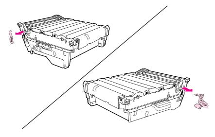
6. Guide the left side of the transfer unit into the front door of the printer. Insert the two pegs on the left side into the holes, and then lower the right side into the door.
