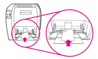
5. Adjust the guides to touch the envelope stack without bending the envelopes. Make sure the envelopes fit under the tabs on the guides.
