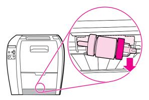
4. Remove the new pickup roller from the bag.
