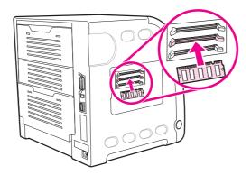
7. Firmly press the DIMM straight into the slot. Close the locks on each side of the DIMM until they snap into place.
