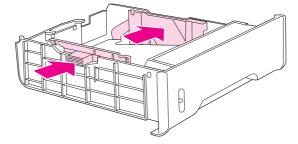
5. Load the paper into the tray. If this is special paper, such as letterhead, load it with the side to be printed down and the top edge toward the front of the tray.
