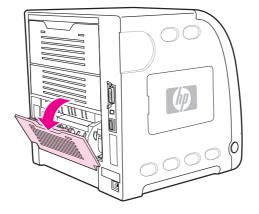
2. Press down on the green levers and remove the paper.
