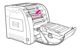
3. Remove the new print cartridge from the bag. Place the used print cartridge in the bag for recycling.
