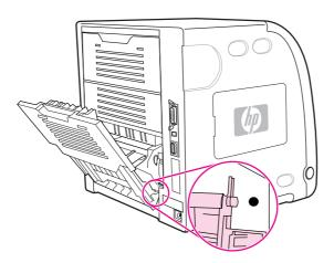
12. Press the ridges on the tab on the left side of the door, and fit the peg into the round hole.
