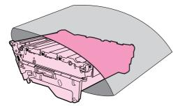
5. Place the new transfer unit on a flat surface. Remove the orange tape and orange shipping locks.
