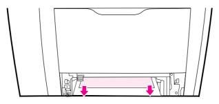
5. Push the metal paper-access plate (duplex pan) up until it locks in place.
