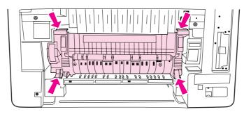
11. Press the black ridges on the front of the fuser until the fuser clicks into place.
