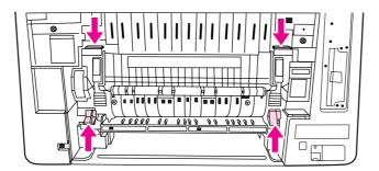
6. Pull the fuser out of the printer.
