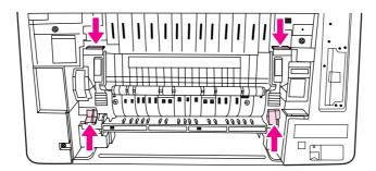
7. Pull the fuser out of the printer.
