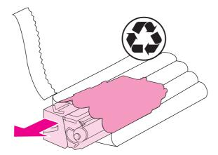
4. Grasp both sides of the print cartridge and distribute the toner by gently rocking the print cartridge from side to side.
