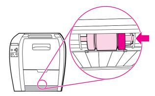
3. Pull down gently on the pickup roller to remove the left peg of the pickup roller from the printer.
