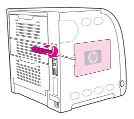
4. Loosen the screws that hold the formatter door on the printer. Remove the formatter door.
