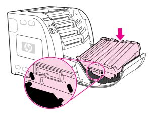
7. Make sure that the blue button on the right blue handle has released (popped up). If the button has not released, grasp the right blue handle and pull the transfer unit toward you.
