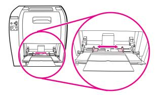
5. Place print media into the tray with the side to be printed up, and the top, short edge in first.
