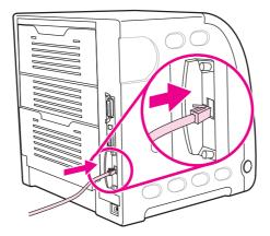
6. Reconnect the power cable, and turn the printer on.
