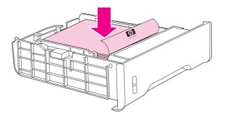
6. Make sure the stack of paper is flat in the tray at all four corners, and keep it below the height tabs.
