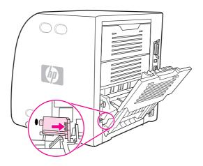
6. Place your thumbs on the blue ridges (near the warning label), and using your fingers, pull up on the blue latches.
