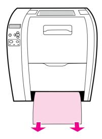
5. If the paper is not visible, check inside the printer in the top of the tray opening. Remove any paper.
