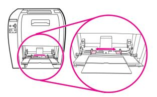
4. Load up to 10 envelopes in the center of Tray 1 with the side to be printed on facing up, with the stamp area closest to the printer, and the short edge toward the printer. Slide the envelopes into the printer as far as they will go without forcing them.
