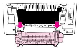
8. On the fuser, squeeze and lift the black tabs to open the shutter door.
