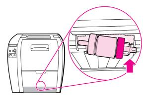
7. Rotate the blue side of the pickup roller until it clicks into place.
