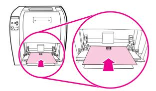
6. Slide the paper width guides inward until they lightly touch the print media stack on both sides without bending it. Make sure the print media fits under the tabs on the width guides.
