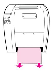
3. On the left side of the tray opening, pull the green lever straight forward until the metal paper-access plate (duplex pan) drops.
