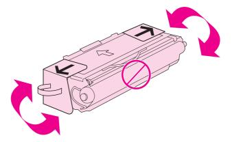
5. Remove the orange shipping locks and the orange shipping tape from the new print cartridge. Discard the shipping tape and shipping locks according to local regulations.
