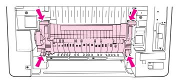
9. Press the black ridges on the front of the fuser until the fuser clicks into place.
