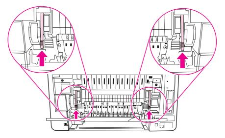
11. To reattach the lower rear door (rear output bin), hold the door at a 45° angle, and fit the peg into the round hole on the right side.
