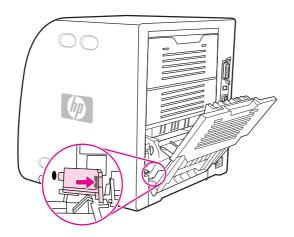
5. Place your thumbs on the blue ridges (near the warning label) and, using fingers, pull up on the blue latches.
