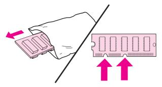
6. Holding the DIMM by the edges, align the notches on the DIMM with the bars in the DIMM slot.
