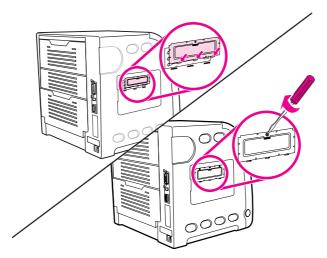
9. Replace the DIMM access door by inserting the tabs on the door into the slots on the printer. Swing the door shut.
