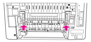
12. To reattach the lower rear door (rear output bin), hold the door at a 45° angle, and fit the peg into the round hole on the right side.
