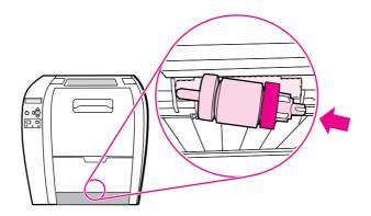
6. Push in on the pickup roller while lifting up on the right side of the pickup roller, so the pin goes into the hole and clicks into place.
