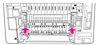
10. Rotate the green levers to the up position.
