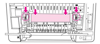
3. Lift the green levers, and close the lower rear door (rear output bin).
