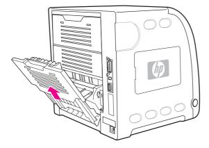
5. Remove the lower rear door (rear output bin) by lifting and pulling the right side of the door while pressing the tab with the ridges on the left side of the door.
