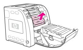
3. If necessary, turn the green roller wheel toward the rear of the printer to advance the paper. Remove any paper.
