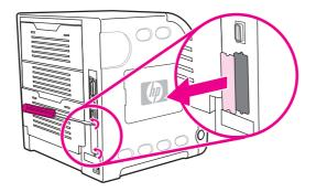
4. Firmly insert the HP Jetdirect print server card into the EIO slot. Insert and tighten the retaining screws that came with the print server card.
