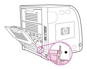
13. Press the ridges on the tab on the left side of the door, and fit the peg into the round hole.
