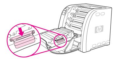
3. Grasp the left blue handle and lift to remove the transfer unit from the printer.
