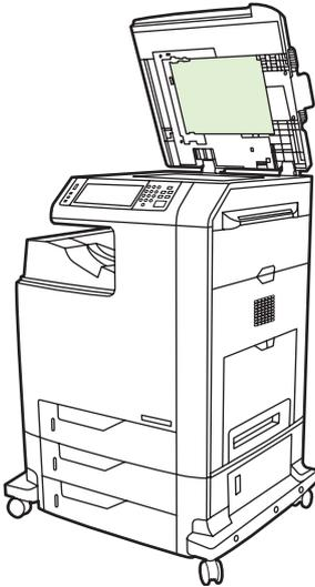
3. Clean the ADF backing with a clean, damp, lint-free cloth. Use an ammonia-based surface cleaner only when a water-dampened cloth does not clean the ADF components.
