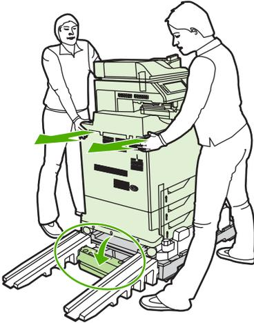
6. Remove the packing tape from the front and rear of the MFP.
