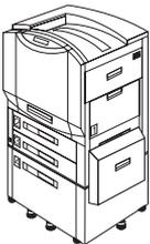
The HP Color LaserJet 8550DN comes standard with a 100-sheet tray 1, a 500-sheet tray 2, a 500-sheet tray 3, a (tray 4) 2000-sheet input tray, a duplexer, 64 MB RAM, an HP JetDirect print server (10/100 Base-TX), an internal hard disk, and five stabilizing legs.
