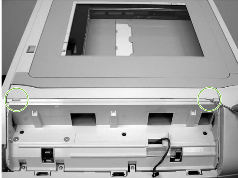
Figure 5-282 Remove the top covers (1 of 2)
