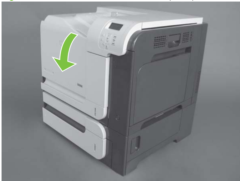
Figure 6-9 Remove the toner-collection unit (1 of 4)
