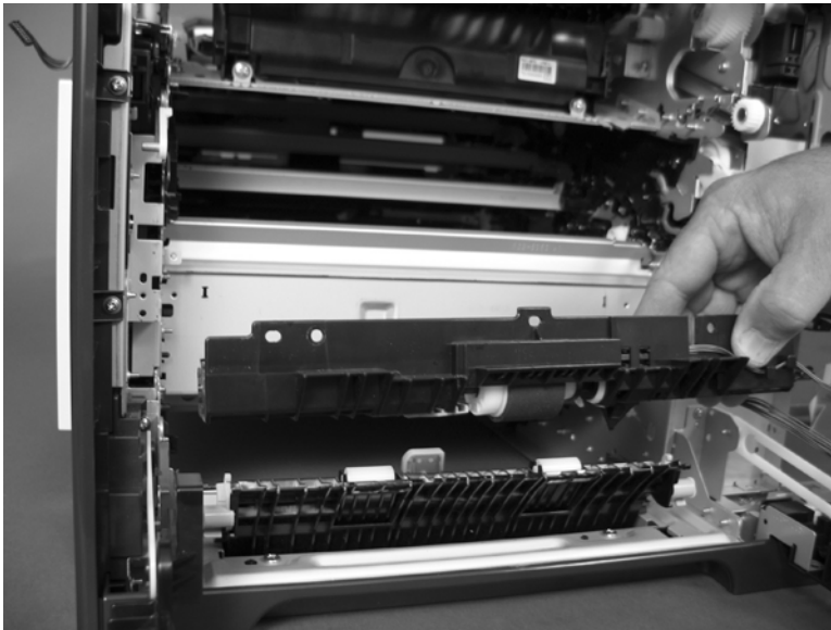
Figure 6-159 Remove the cassette-pickup assembly (3 of 3)
