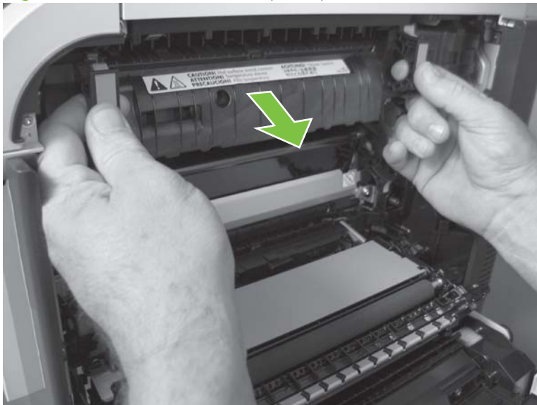
Figure 6-19 Remove the fuser (2 of 2)
