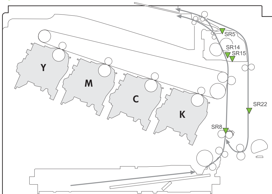
Figure 5-43 Jam detection sensors
