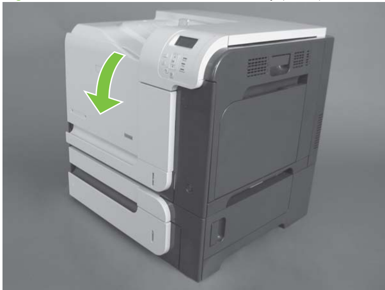
Figure 6-42 Remove the front-door assembly (1 of 2)
