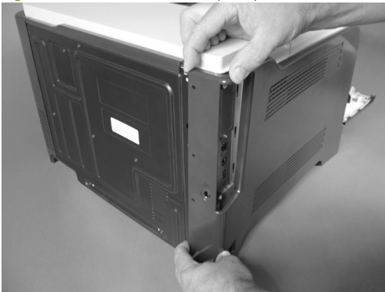
Figure 6-56 Remove the left cover (2 of 5)
