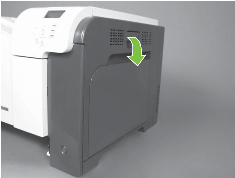
Figure 6-44 Remove the right-door assembly (1 of 8)
