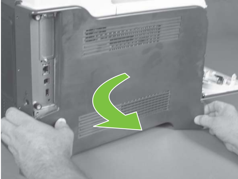
Figure 6-59 Remove the left cover (5 of 5)
