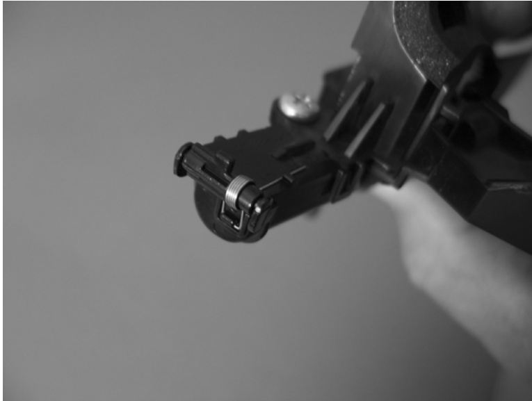
Figure 6-100 Reinstall the residual-toner collection door
