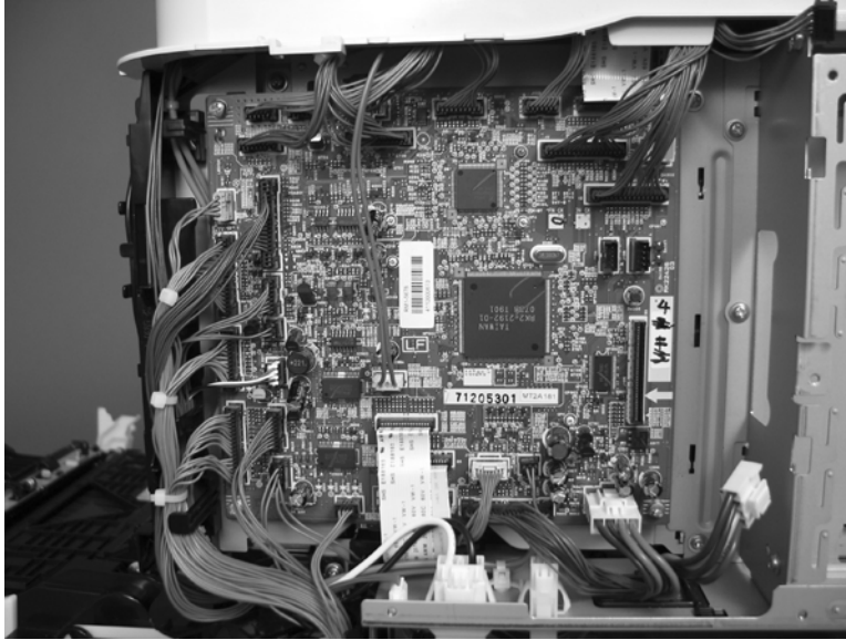
Figure 6-123 Remove the DC controller PCA and tray (2 of 4)
