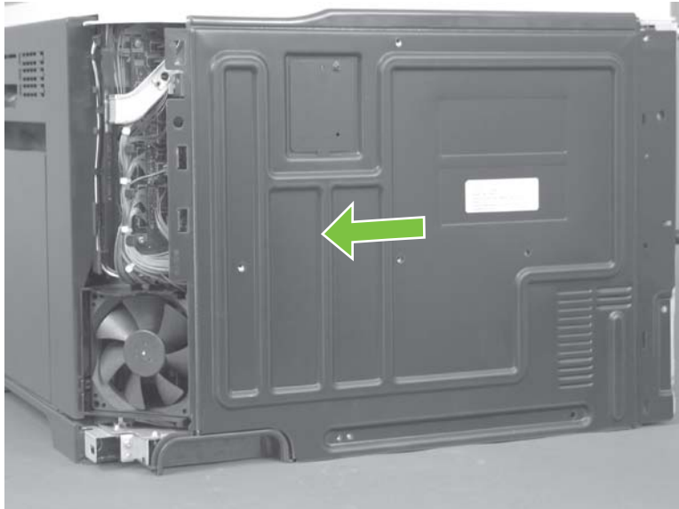
Figure 6-73 Remove the rear cover and upper-rear cover (2 of 4)
