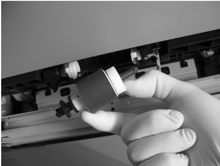
Figure 6-23 Remove the pickup roller (Tray 2) (4 of 4)
