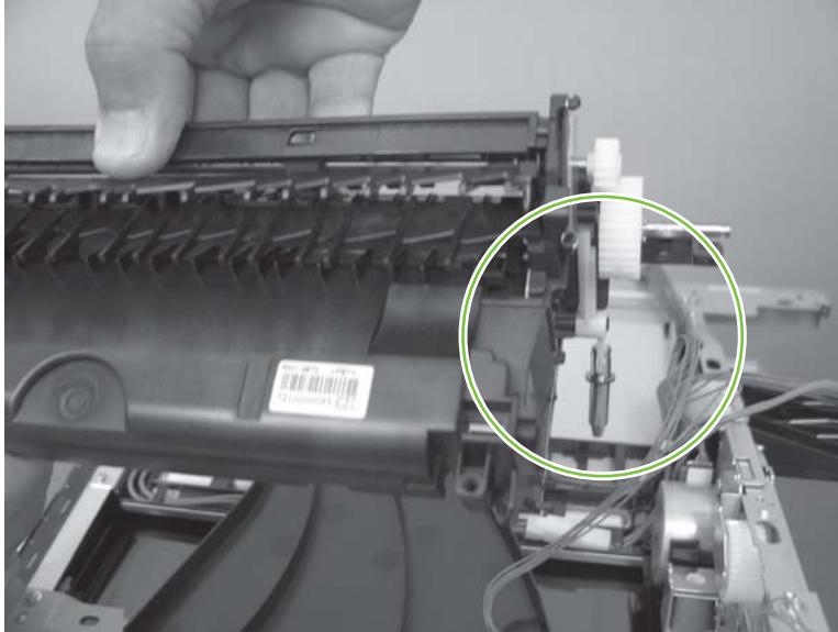
Figure 6-223 Reinstall the delivery assembly (1 of 2)
