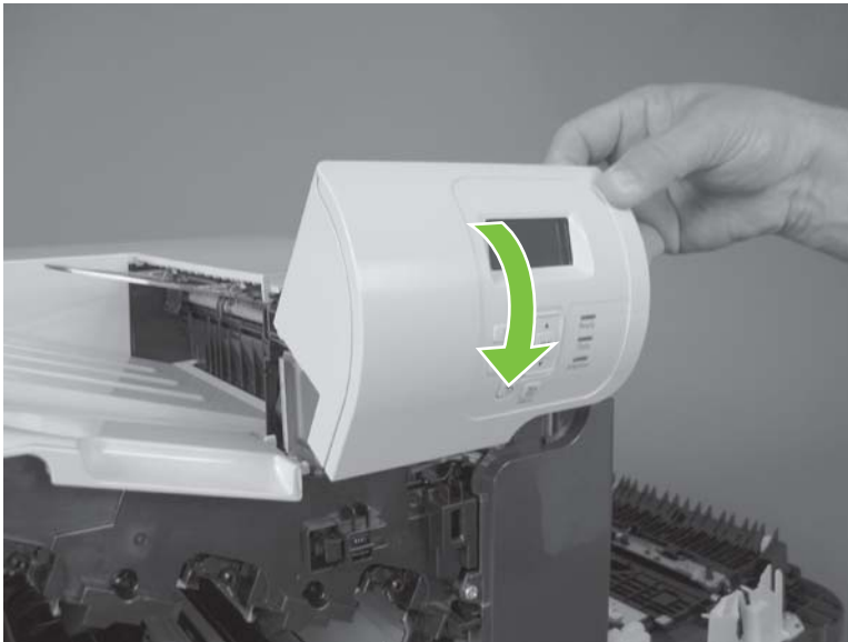
Figure 6-62 Remove the control-panel assembly (3 of 4)
