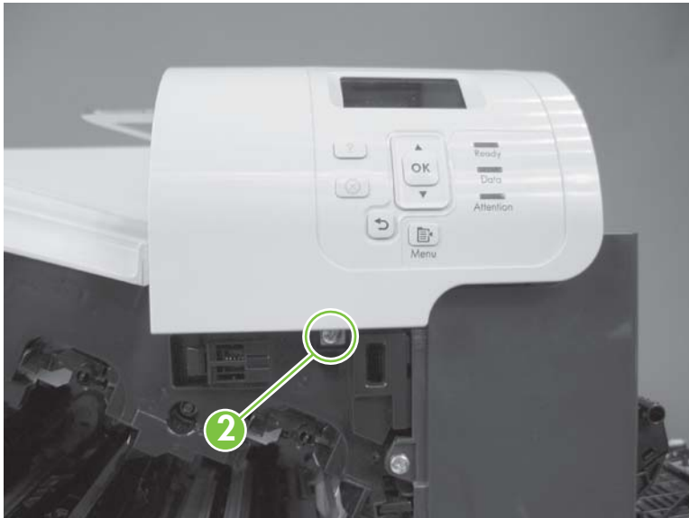
Figure 6-61 Remove the control-panel assembly (2 of 4)
