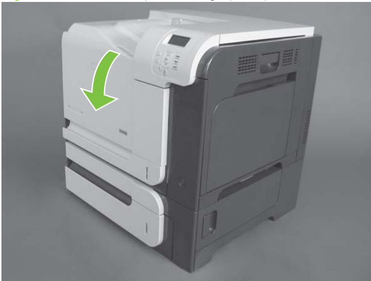
Figure 6-5 Remove the print cartridge (1 of 2)
