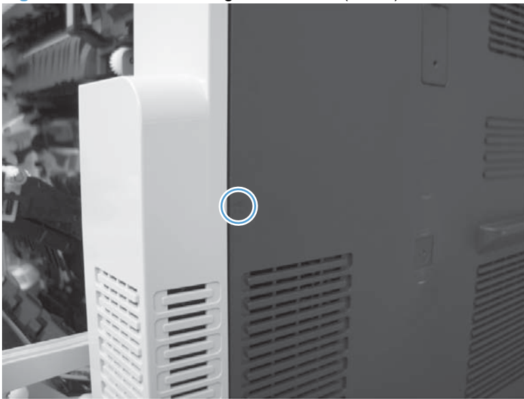
Figure 2-57 Remove the right-rear cover (1 of 2)
