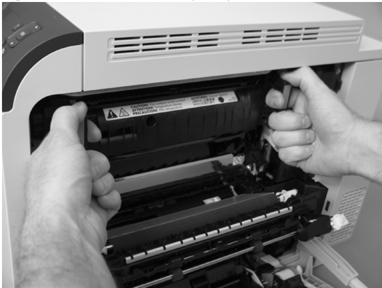
Figure 2-19 Remove the fuser (2 of 2)
