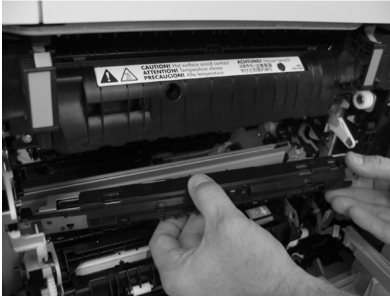
Figure 2-87 Remove the RD sensor assembly (7 of 7)
