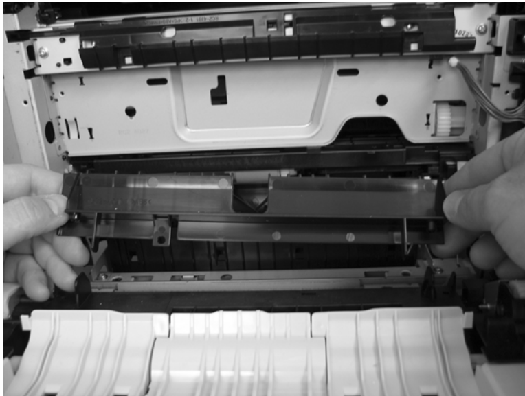
Figure 2-170 Remove the tray-pickup assembly (7 of 11)
