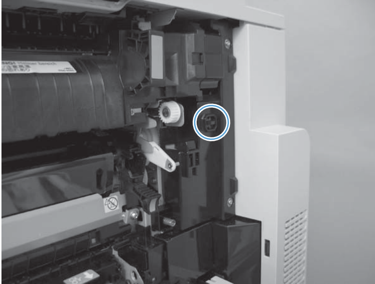
Figure 3-18 Test the right door switch
