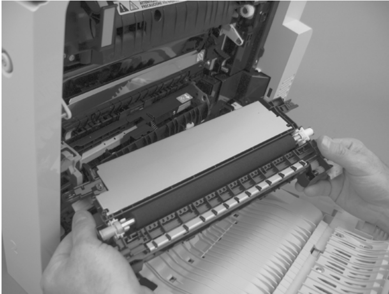
Figure 2-73 Remove the secondary transfer assembly (3 of 3)
