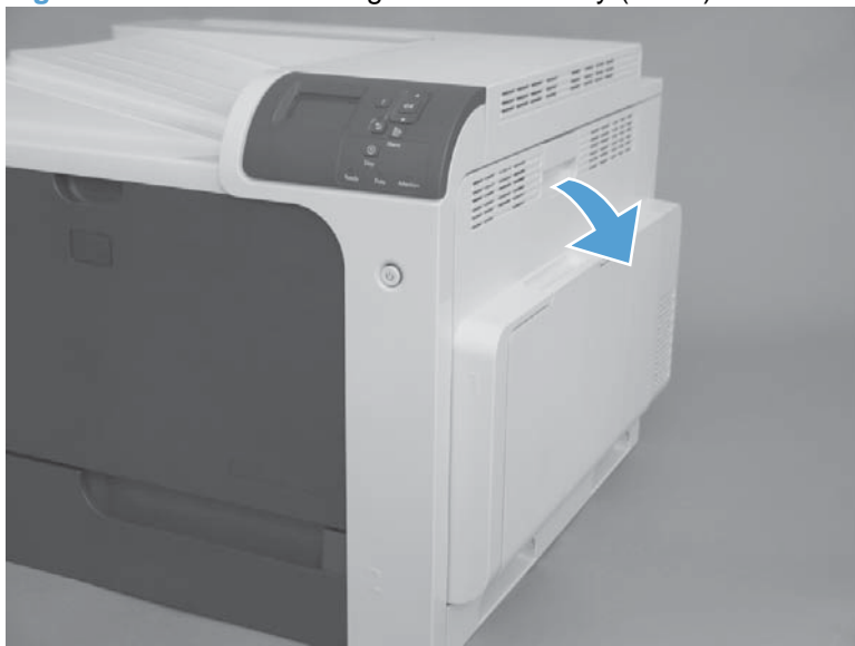
Figure 2-60 Remove the right-door assembly (1 of 9)
