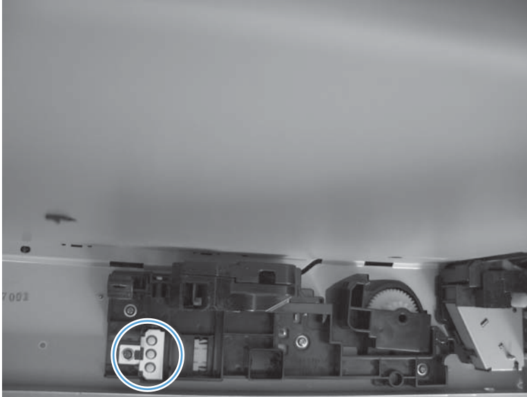
Figure 3-22 Test the Tray 2 paper size switches
