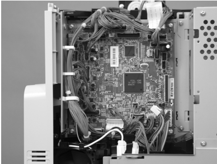
Figure 2-128 Remove the DC controller PCA only (1 of 2)
