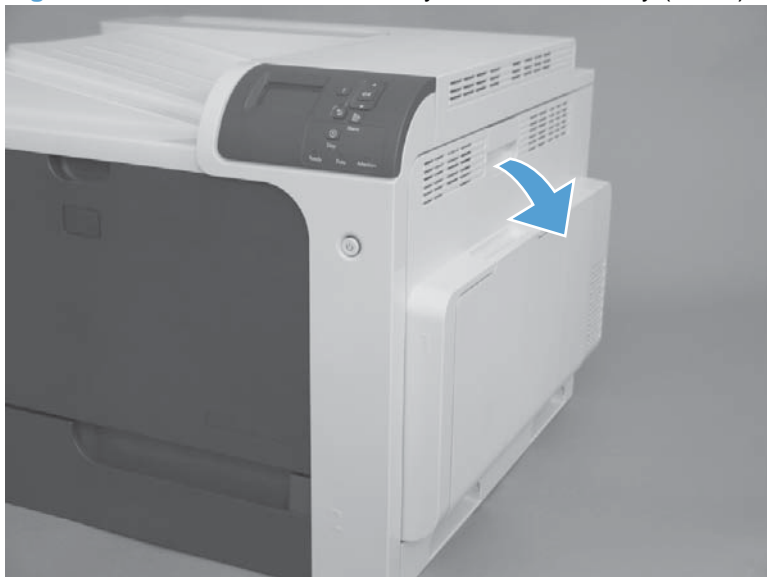
Figure 2-71 Remove the secondary transfer assembly (1 of 3)
