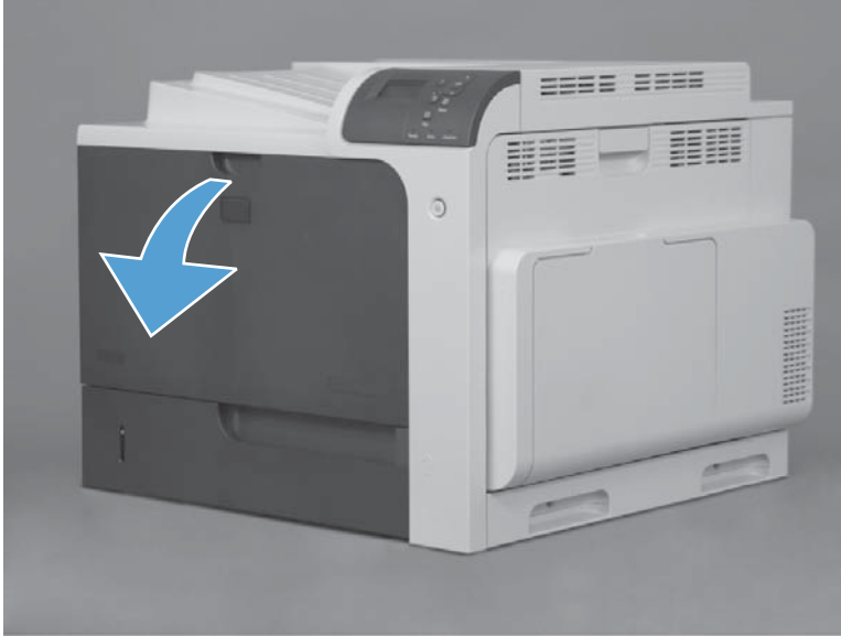
Figure 2-35 Remove the upper-left cover (1 of 3)
