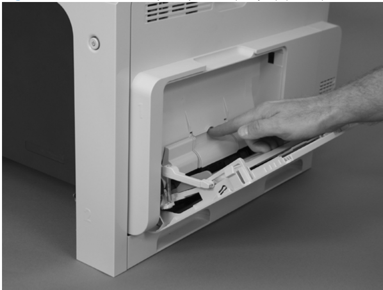
Figure 2-22 Remove the pickup roller (Tray 1) (2 of 5)
