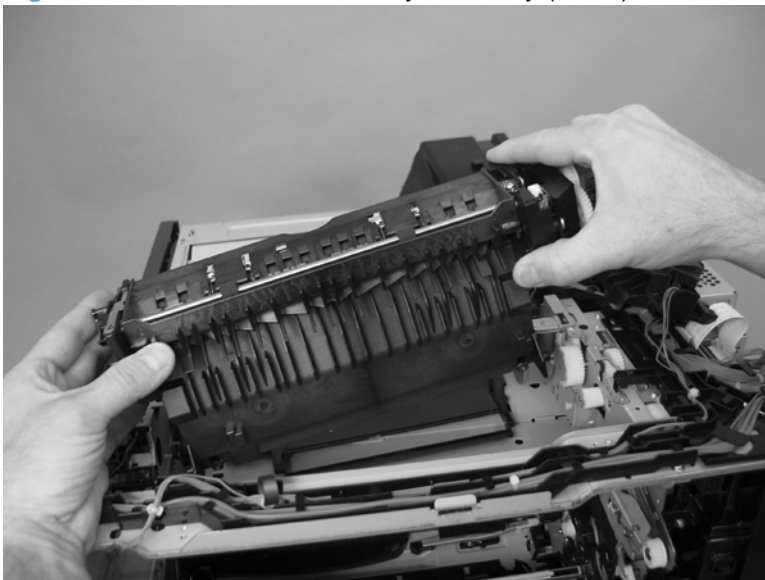
Figure 2-119 Remove the delivery assembly (7 of 7)
