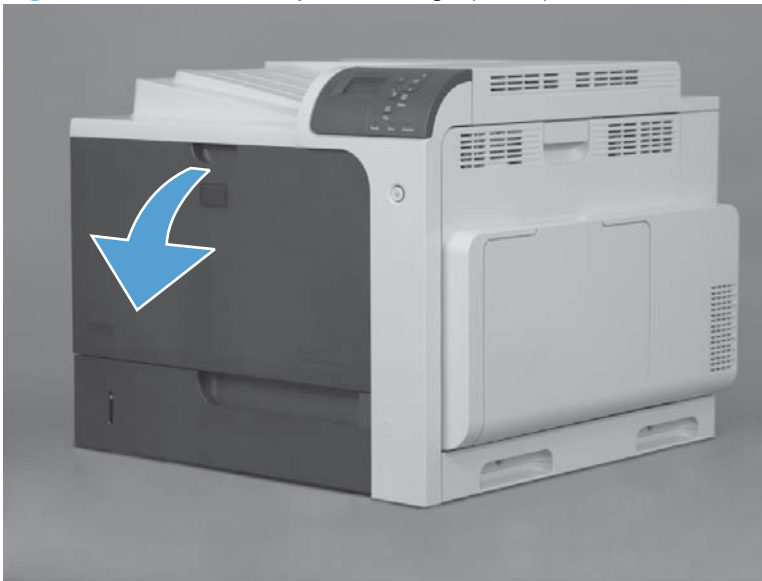
Figure 2-4 Remove the print cartridge (1 of 2)
