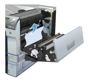
3. If paper is visible entering the bottom of the fuser, gently pull downward to remove it.
