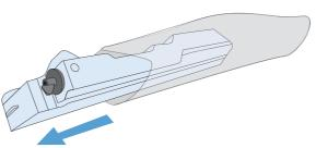
Insert the bottom of the new unit into the product first and then push the top of the unit until it clicks into place.
