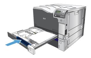
5. The control panel prompts you to set the paper size and type. Select the **Custom** setting, and then configure the X and Y dimensions of the custom paper size.
