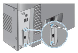
6. Reconnect the power cable, connect the interface cable to the HP Jetdirect print server card, and turn the product on.
