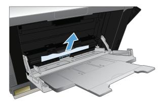
2. If you cannot remove the paper, or if no jammed paper is visible in Tray 1, close Tray 1 and open the upper right door.
