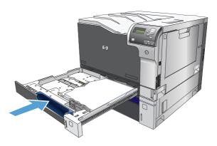
3. If the jam is in Tray 3, you also can open the door on the right side of the tray, remove the jammed paper, and then close the door.
