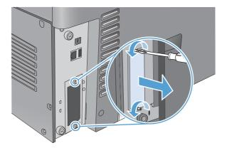
4. Firmly insert the HP Jetdirect print server card or other EIO accessory into the EIO slot.
