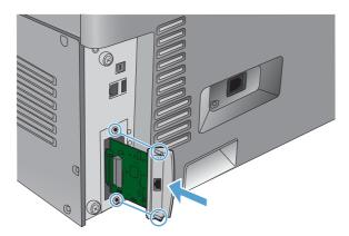
5. Insert and tighten the retaining screws that came with the print server card.
