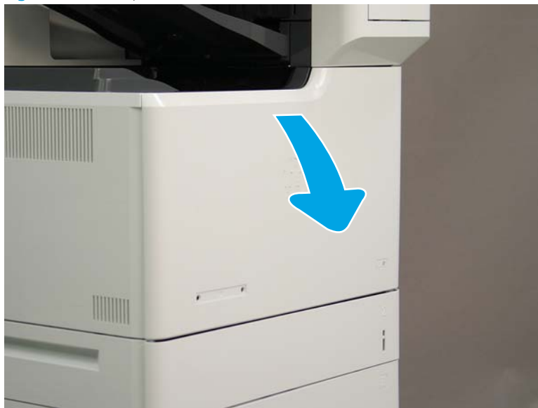
Figure 1-1278 Open front door
