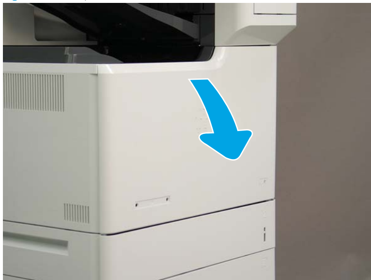
Figure 1-618 Open front door
