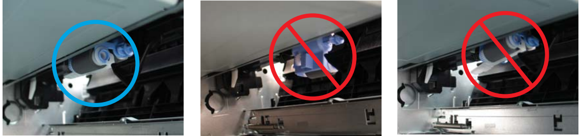
Figure 1-244 Roller correct and incorrect installation
