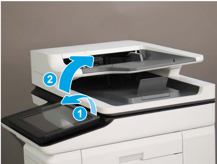
Figure 1-1190 Tilt the control panel and open the document feeder
