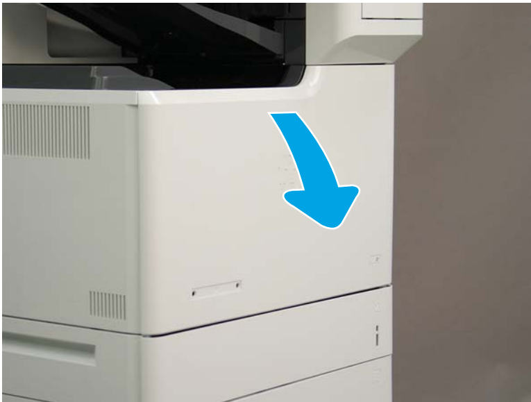
Figure 1-1179 Open front door
