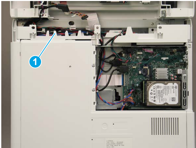
Figure 1-335 Cable routing for M681dh, M681f, and Flow M681f
