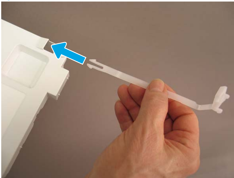
Figure 1-1017 Reinstall the link arm
