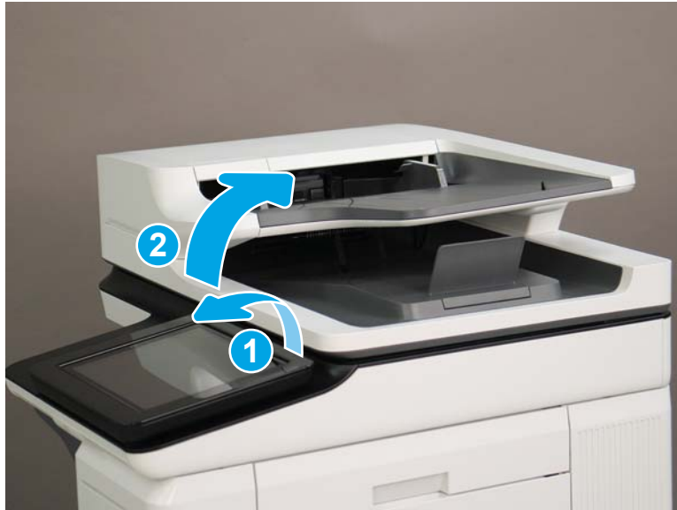
Figure 1-1774 Tilt the control panel and open the document feeder
