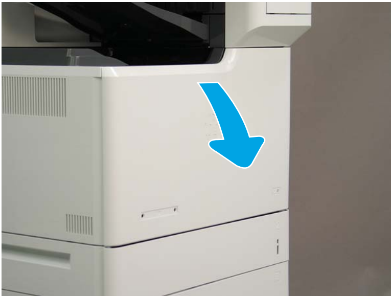
Figure 1-1267 Open front door
