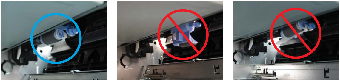
Figure 1-249 Roller correct and incorrect installation
