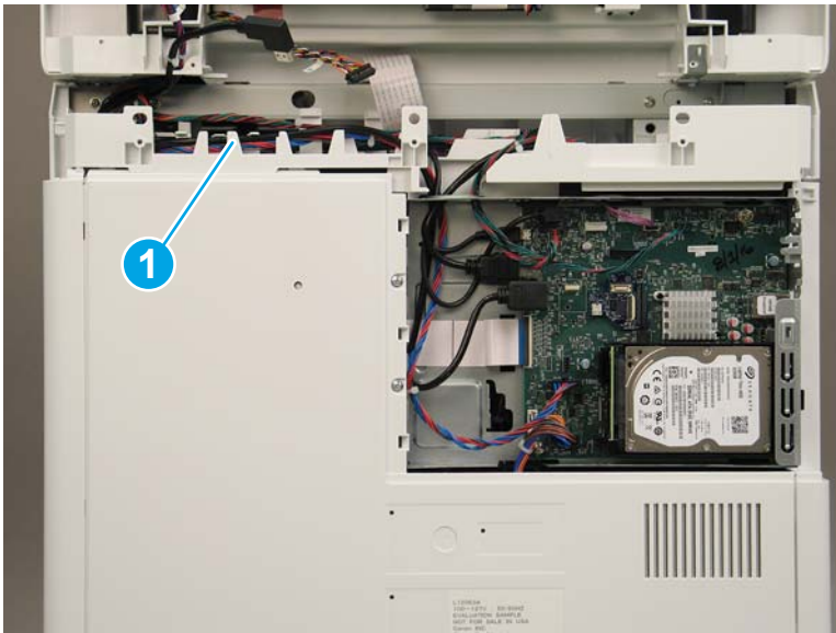
Figure 1-1436 Cable routing for M681dh, M681f, and Flow M681f
