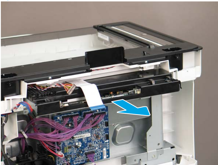
Figure 1-671 Remove the SCB
