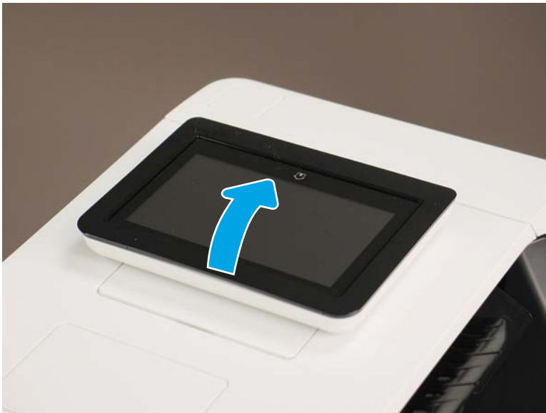
Figure 1-1879 Tilt the control panel up
