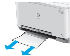
3. If no jammed paper is visible, or if jammed paper is deep enough in the Tray 2 cavity that it is difficult to remove, press down on the single-sheet priority feed slot, and then remove the feed slot tray.
