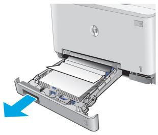
Remove any jammed or damaged sheets of paper.
