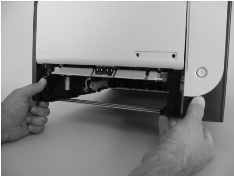
3. Release the two roller-cover locking pins, and then remove the cover.
