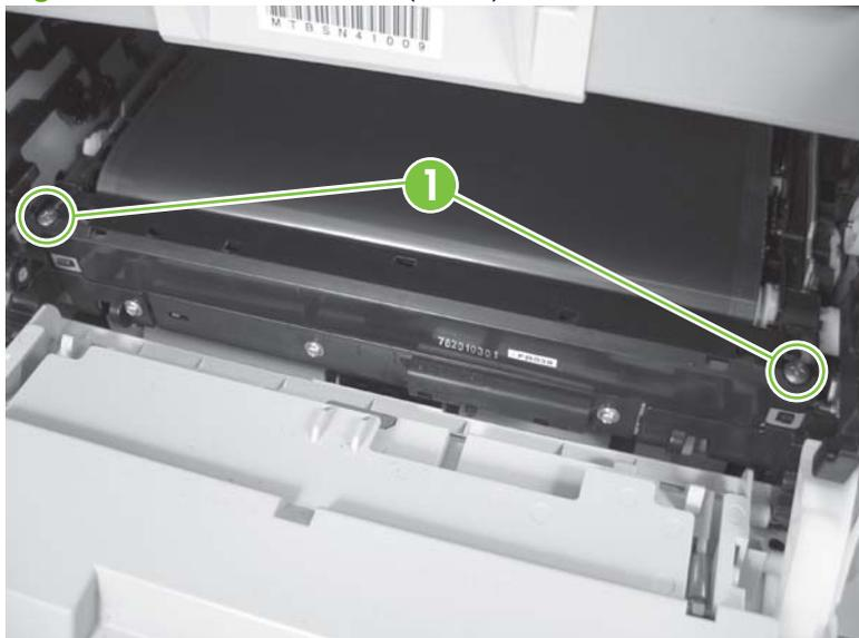
3. Carefully rotate the color misregistration sensor away from the ITB.
