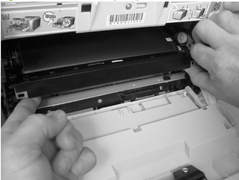
6. To release the ITB, you might have to pen the rear door, and carefully lift up on the sheet-metal portion (callout 3).
