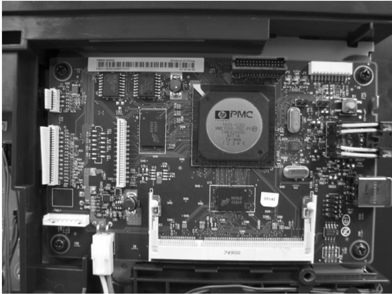
3. Remove four screws (callout 1), and then remove the formatter PCA.
