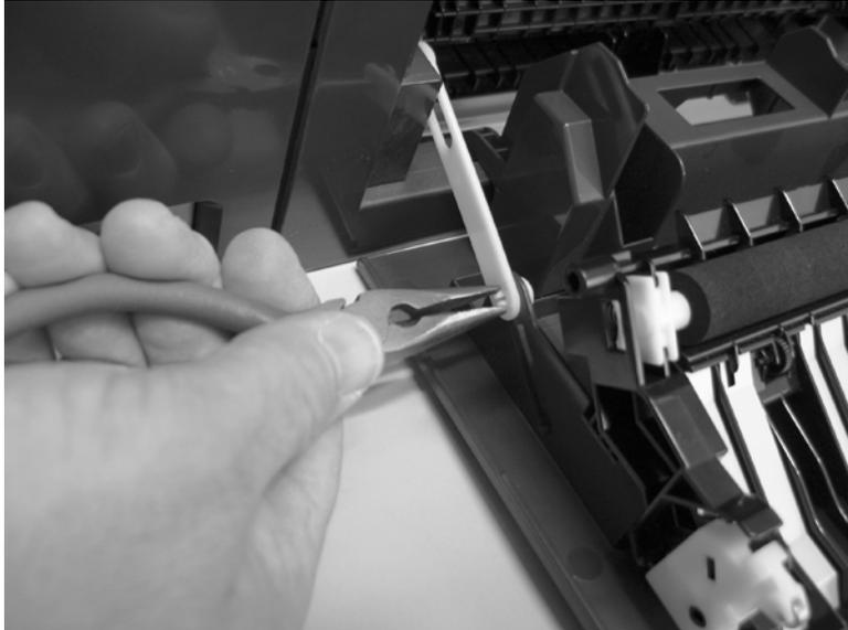
3. Use a small, flat-blade screwdriver to carefully remove the remaining link cap, and then remove the rear-door stopper.
