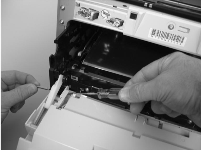
4. Use a precision-point screwdriver to push the right-side door pin out of the link.
