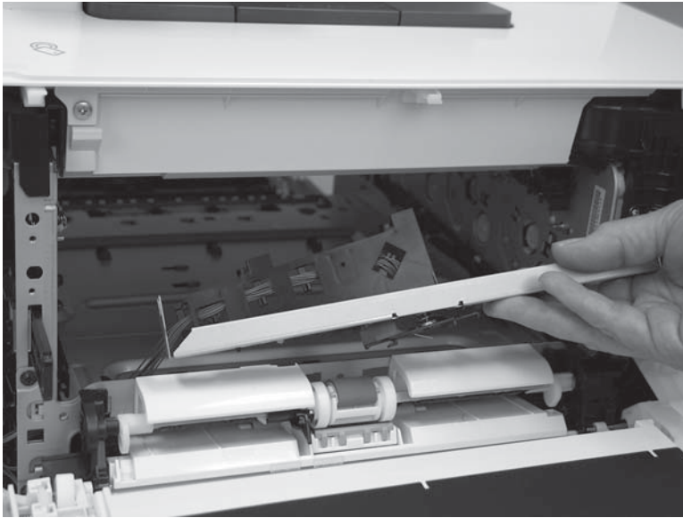
Figure 1-2082 Remove the registration density sensor and guide
