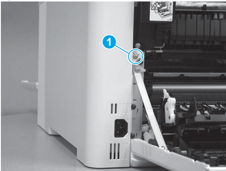
Figure 1-1140 Install one screw
