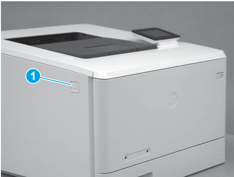
Figure 1-1268 Release the front door
