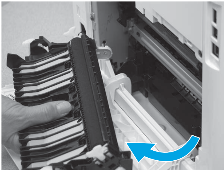
Figure 1-1867 Remove the secondary transfer assembly
