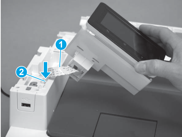
Figure 1-981 Install the flat cable
