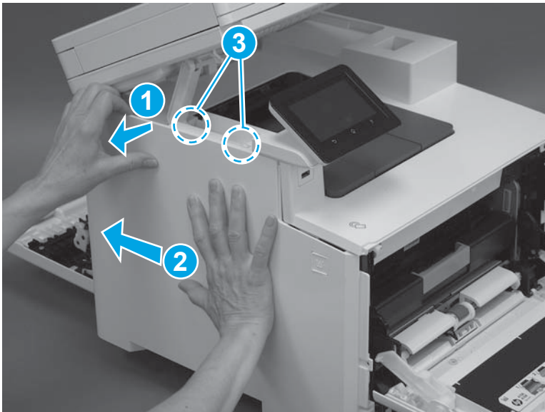
Figure 1-1646 Release one tab and two hooks
