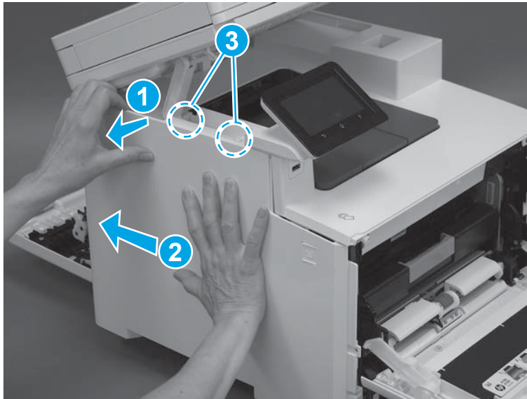
Figure 1-4697 Release one tab and two hooks
