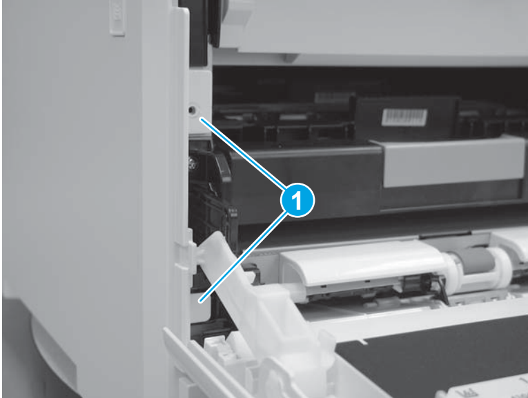
Figure 1-589 Release two tabs
