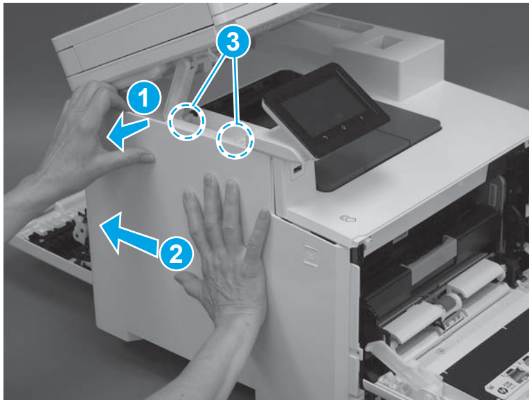
Figure 1-1473 Release one tab and two hooks
