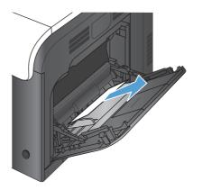
2. If you cannot remove the paper, or if no jammed paper is visible in Tray 1, close Tray 1 and open the right door.
