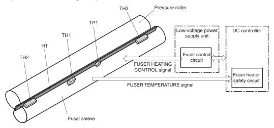
Table 1-9 Fuser (fixing) components
