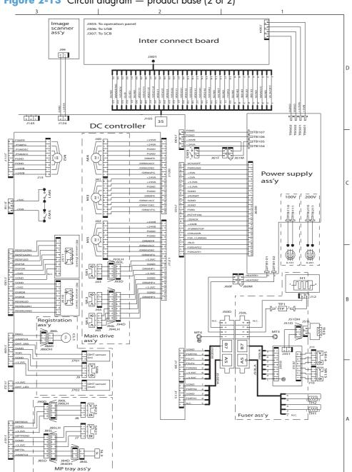
Figure 2-13 Circuit diagram — product base (2 of 2)
