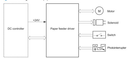
The input trays contain several motors, solenoids, sensors, and switches, as described in the following table.
