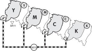
Four developing units disengaged
