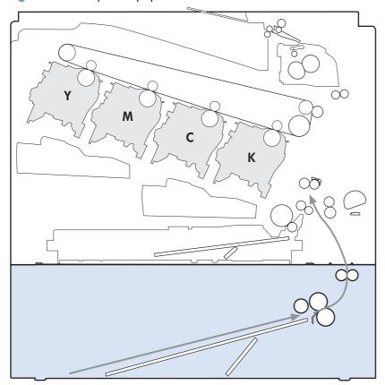
The paper-deck drivers contain a microcomputer and control the paper feeder. The paper-deck drivers receive commands from the DC controller. If the DC controller is unable to communicate with a paper-deck driver, it notifies the formatter that the optional paper feeders are not connected correctly.
