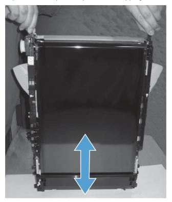
d. Reinstall the ITB, and then close the right and front doors to initialize the product. After about 35 seconds, the message Install supplies will appear on the control-panel display.
