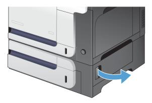
If paper is visible, gently pull the jammed paper up or down to remove it.
