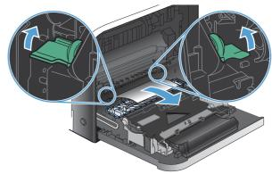
**8.** If paper is visible entering the bottom of the fuser, gently pull downward to remove it.
