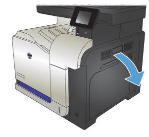
If paper is visible inside the right door, gently pull the trailing edge to remove it.
