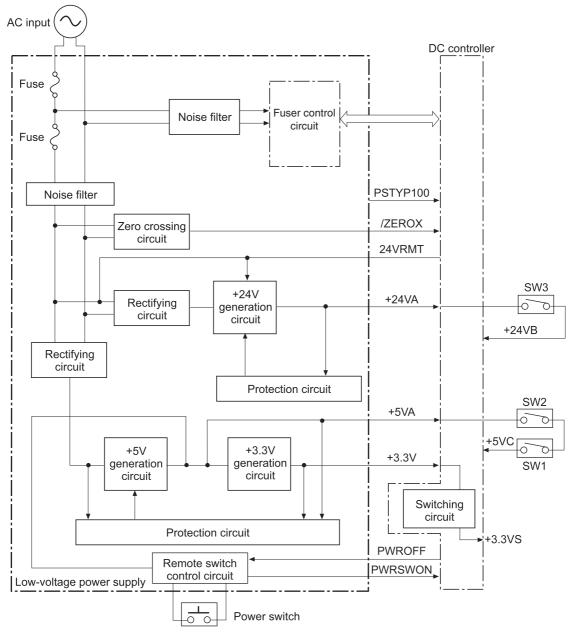
The low-voltage power supply converts the AC power into three DC voltages, which it then subdivides, as described in the following table.
