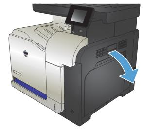
2. If paper is jammed as it enters the output bin, gently pull the paper downward to remove it.
