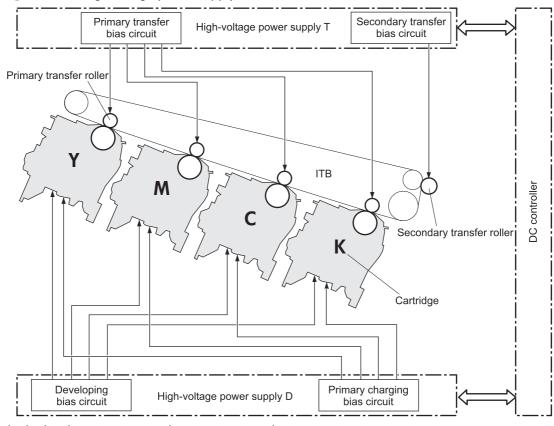
The high-voltage power supply contains several separate circuits.
