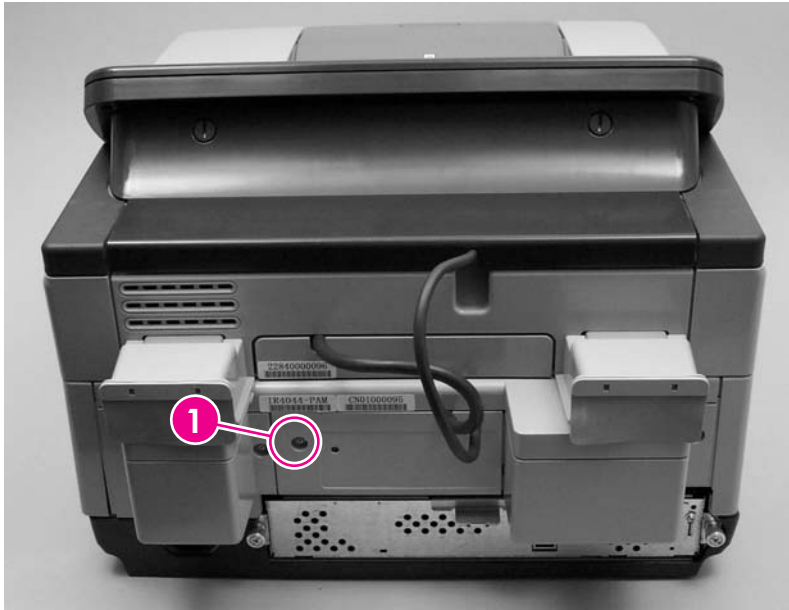
Figure 6-46 Removing the scanner rear cover
