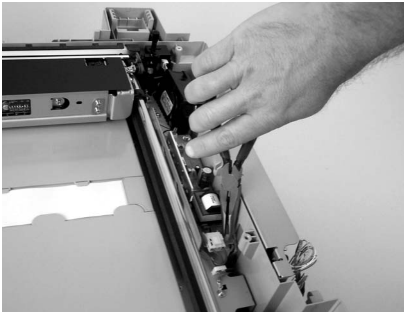
Figure 6-92 Removing the inverter (3 of 4)
