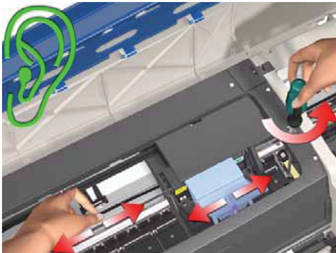
Figure 5-4 Cross-Section - Raising the Pivot Assembly
