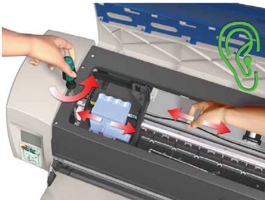
Figure 5-2 Cross-Section - Raising the Pivot Assembly
