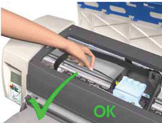
Correct: move using the belt.
