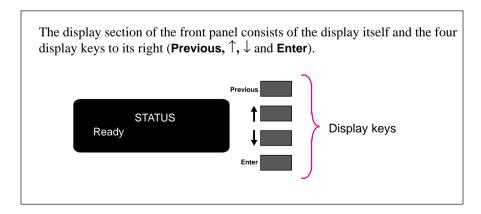
The display can show two lines of text and is used for displaying:
