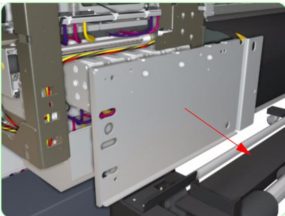
**11.** Remove the metal plate from the chassis.
