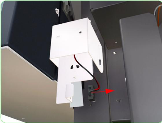
**8.** Remove the Waste Bottle Sensor from the Printer.
