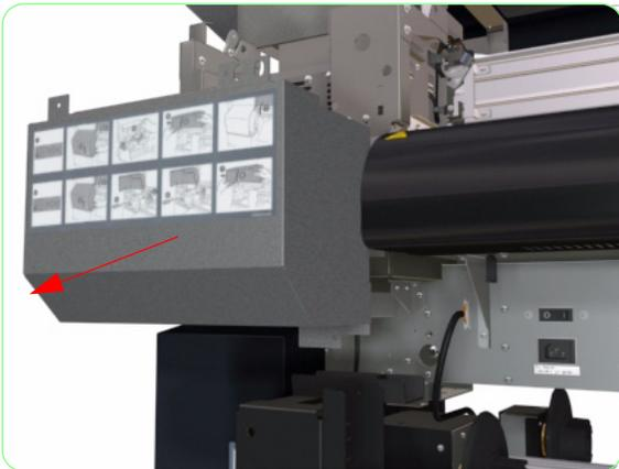
6. Remove the Lower Capping Cover from the Printer.
