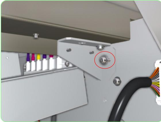
**25.** Remove one screw that secures the metal bracket.
