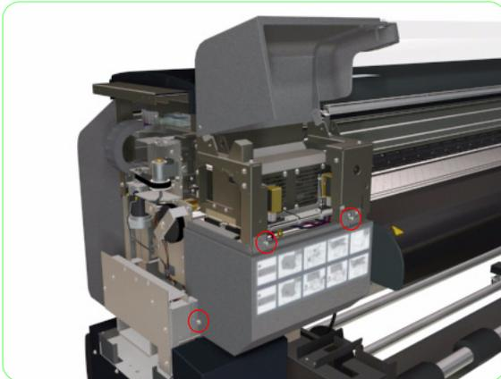
4. Remove three screws that secure the Lower Capping Cover to the Printer.
