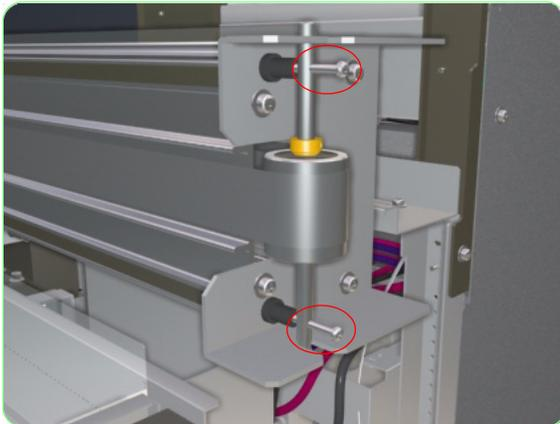
5. Remove one screw that secures the Belt to the left side of the Carriage Assembly and then release the Belt from the Carriage Assembly.
