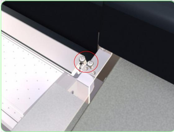
1. Remove two screws that secure the Rear Cover to the right hinge.
