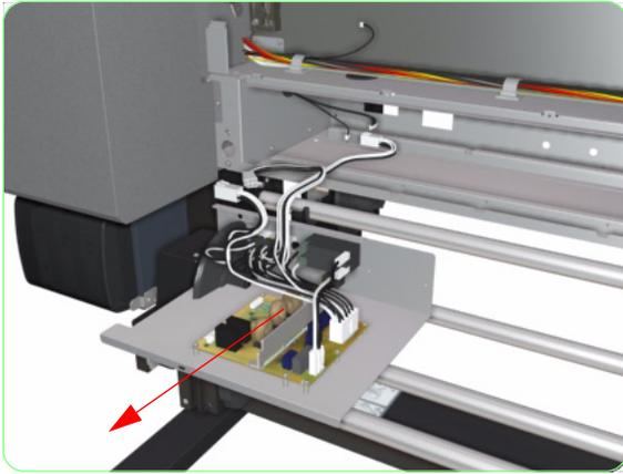
8. Remove the Heater Relay Assembly from the Printer.
