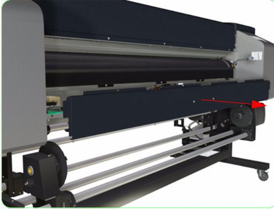
7. Remove the Electronics Module Cover from the Printer.
