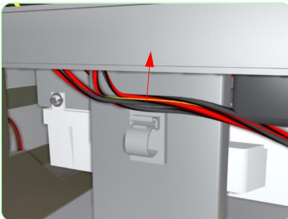
7. Release the Wiping Station cables from the cable clip.
