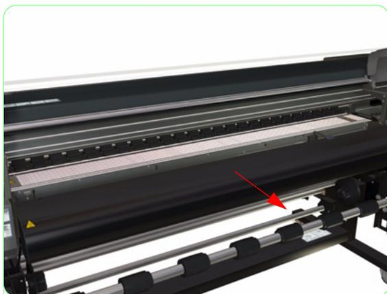
3. Pull out the Rear Heater slightly.
