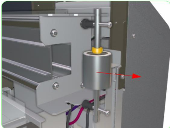
**11.** Remove the Tension Pulley from the Printer.
