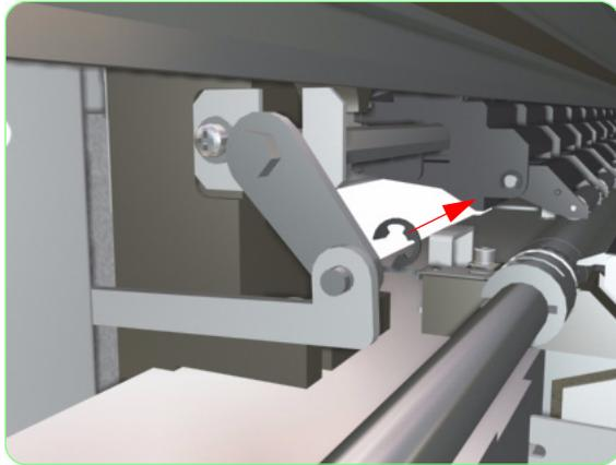
9. Remove the C ring that secures the Linkage to the Pinchwheel Cam.
