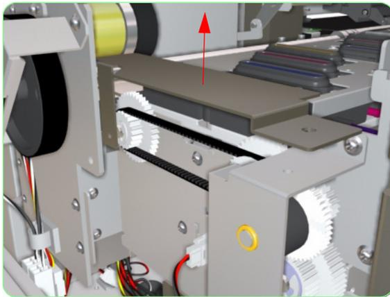
**17.** Remove the metal bracket from the Capping Station.
