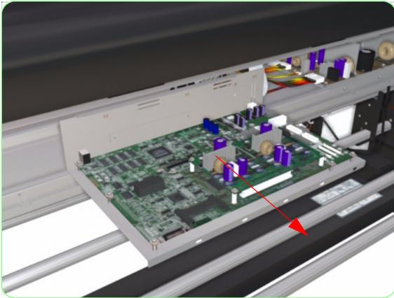
**6.** Remove the Main PCA Tray from the Printer.
