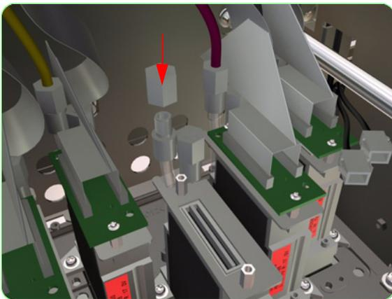
9. Install a Tube Cap on to the Printhead.
