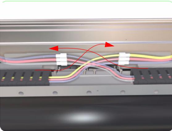
**34.** Pull the tubes out of the cable carrier in the direction shown.
