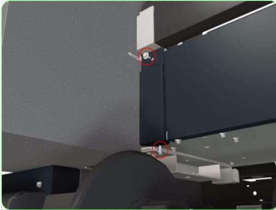
1. Remove two screws that secure the Left Electronics Module Side Trim to the Printer.
