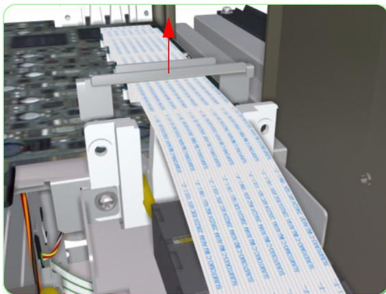
**13.** Remove the metal bracket from the Carriage Assembly.
