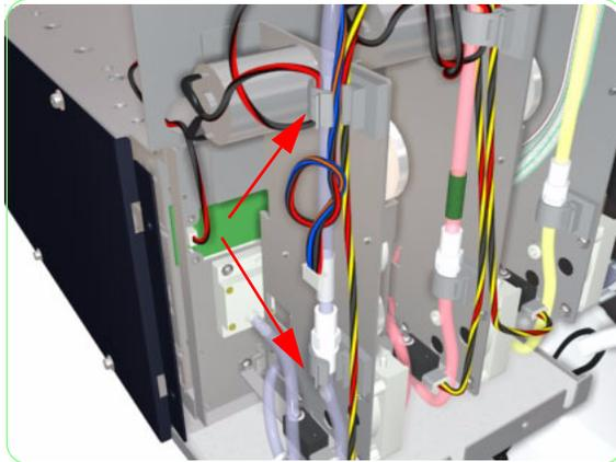
**26.** Detach each tube from its plastic securing clamp.
