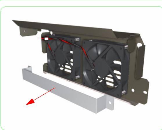
**12.** Remove the metal bracket from the Printhead Cooling Fan Assembly.
