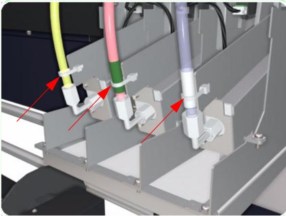
**29.** Cut the Insulock ties (but do not loosen the plastic nuts) and drain the ink from the subtank. When the flow of ink stops, pull the tube through from the back to the front side and drain the rest of the ink from the subtanks.
