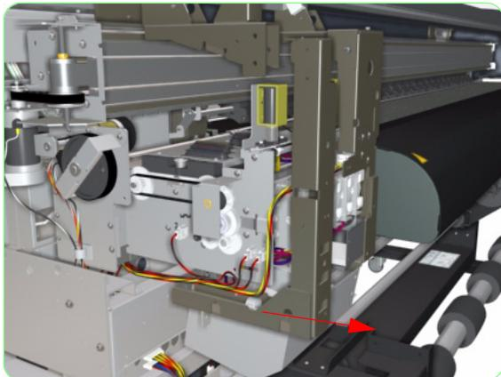
**22.** Remove the Left Capping Frame from the Printer.
