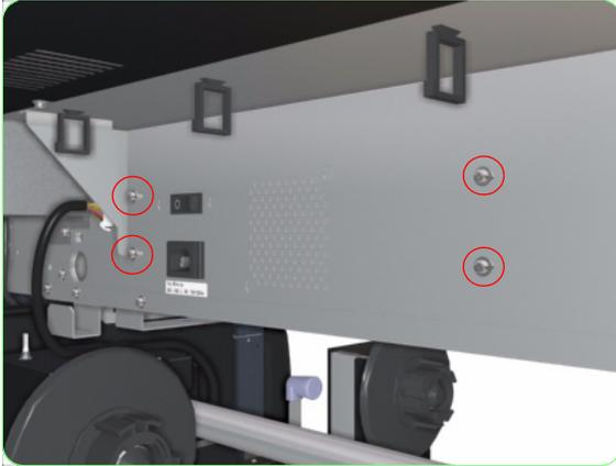
3. Remove three screws that secure the Power Supply Unit to the Printer from the front.
