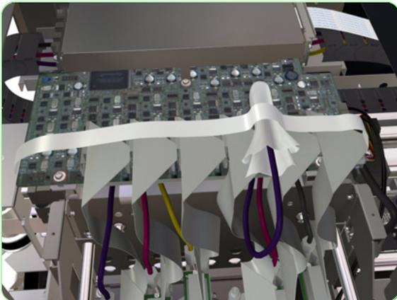
8. Cover the Ink Tube carefully with a paper cloth and secure it to the Carriage Assembly with some tape.
