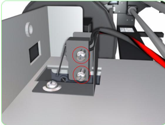
**6.** Remove two screws that secure the IC Door Sensor to the Ink Supply Station.
