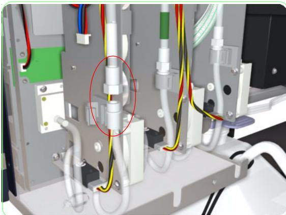
**58.** Connect the subtank tube to the supply pump.
