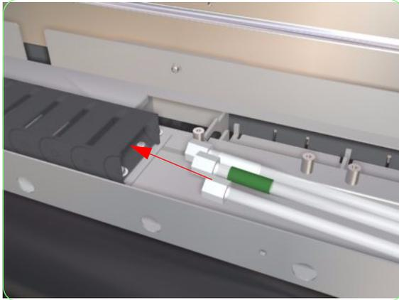
**43.** Thread the *narrow ends* of remaining three tubes through the other end of the cable carrier.
