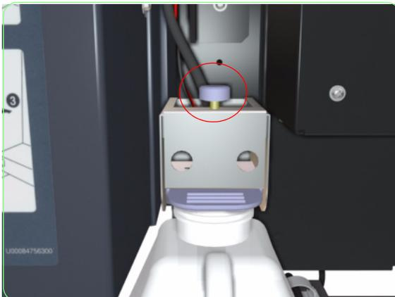
**25.** Loosen the screw that locks the Waste Bottle Bracket into place. You will use the waste bottle to collect the ink.
