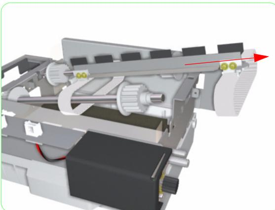
**13.** Remove the Wiper Blade and belts from the Wiping Station.
