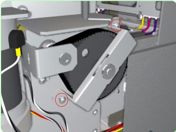
5. Remove the Paper-Axis Gear Plate from the Printer.
