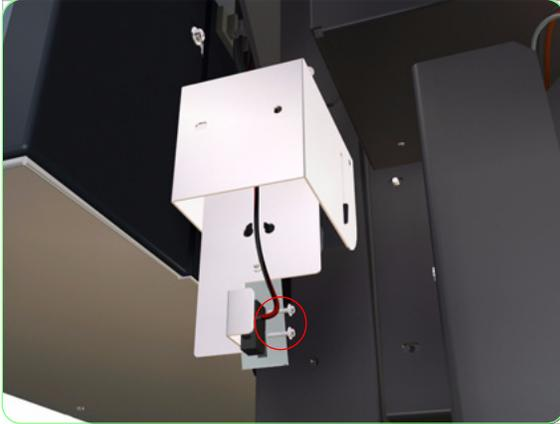
**7.** Remove two screws that secure the Waste Bottle Sensor to the Bracket.
