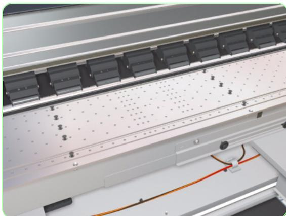
4. Remove the Center Platen from the Printer.
