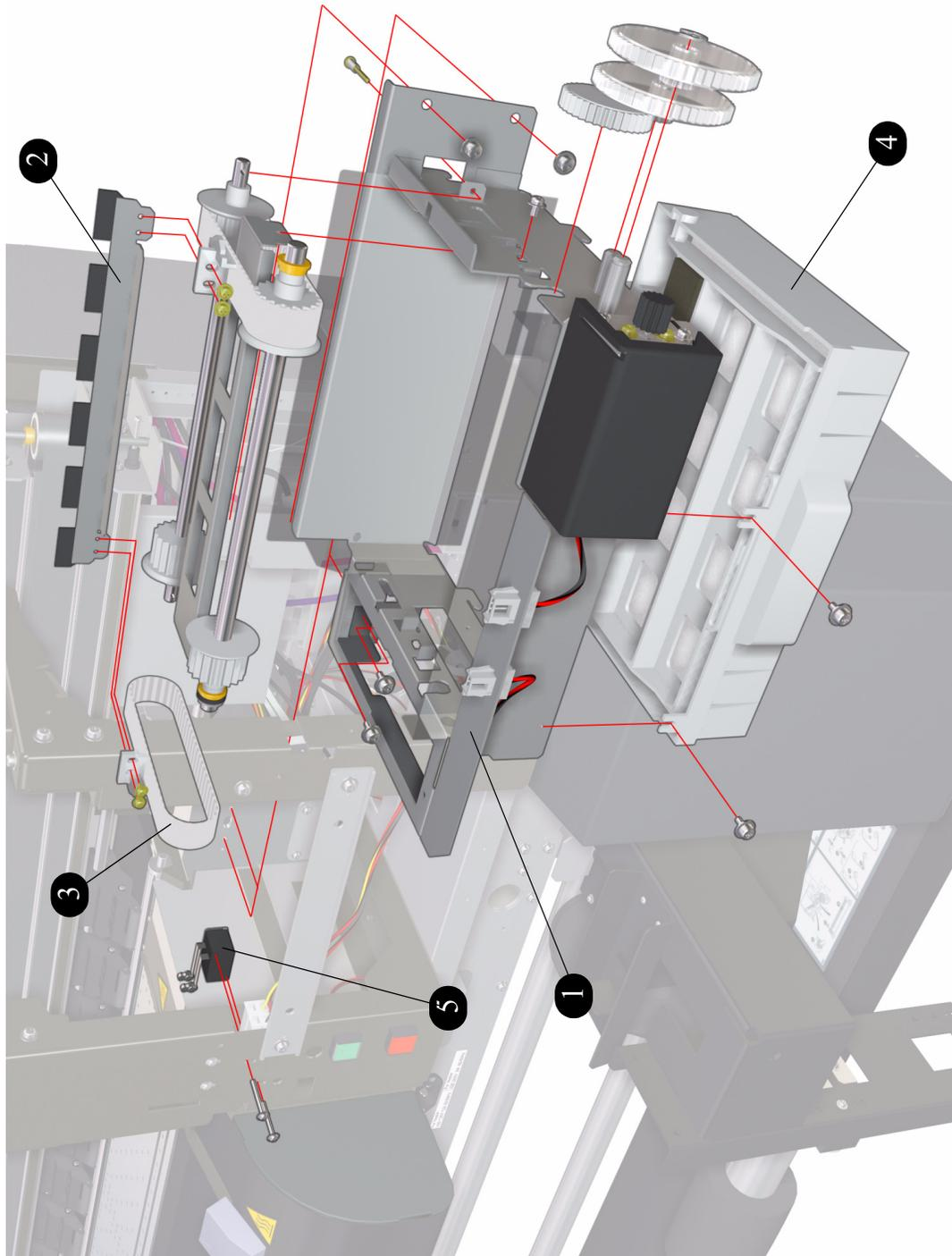
**Figure 12: Wiping Assemblies**
