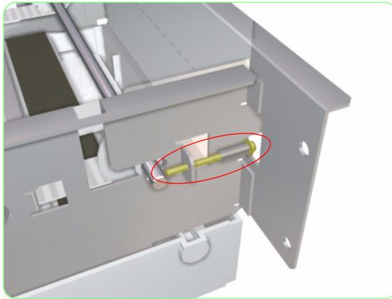
**9.** Remove the screw and spring from each side of the Wiping Station.
