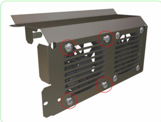
**13.** Remove four screws that secure the Printhead Cooling Fan to the Printhead Cooling Fan Assembly.
