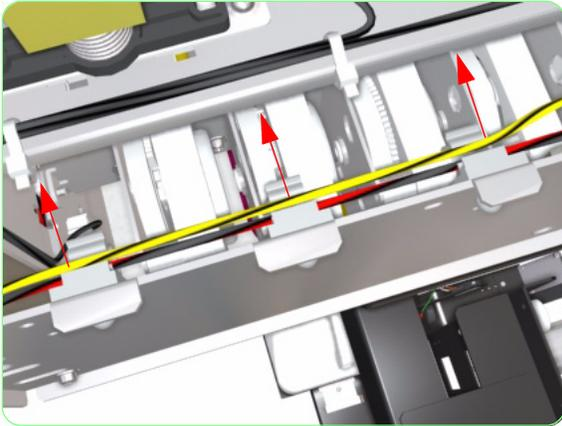
**8.** Release ALL the cables from the cable clips.
