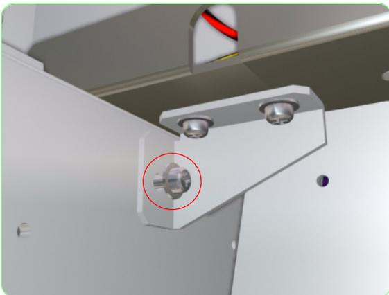
**21.** Remove one screw that secures the metal bracket.
