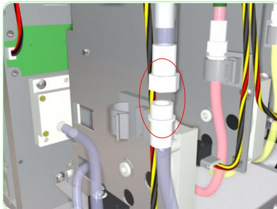
**27.** Taking one tube at a time, loosen the nut, separate the connected tubes.
