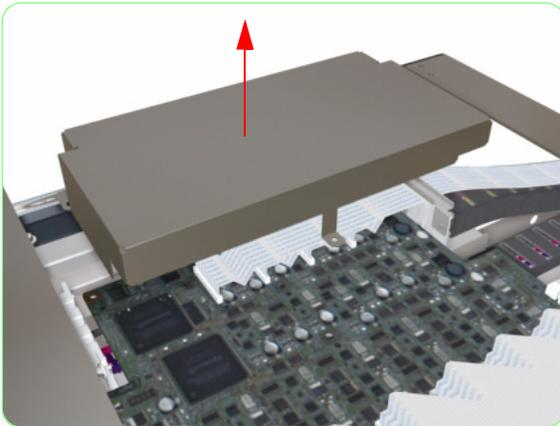
**11.** Remove the Carriage PCA Cover from the Carriage Assembly.
