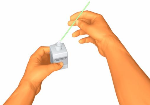
**Make sure that you use the Wiping Cleaning Liquid and NOT the Cap Cleaning Liquid to clean the Wiper Blade. The Cap Cleaning Liquid is not strong enough to clean the Wiper Blade properly and could cause damage to the Printheads.**
