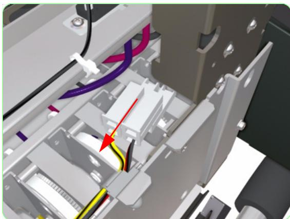
**12.** Disconnect the Cable from the Right Rear Cover Sensor.
