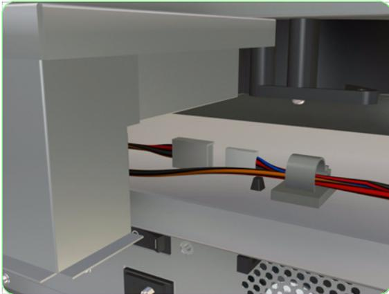
3. Remove one screw that secures the Rear Media Sensor to the Bracket.
