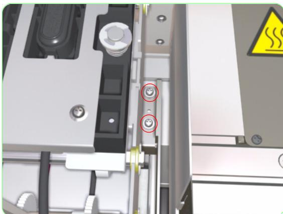
**24.** Remove two screws that secure the Right Capping Frame to the bottom.
