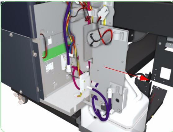
8. Remove the Ink Pump Assembly from the Printer.
