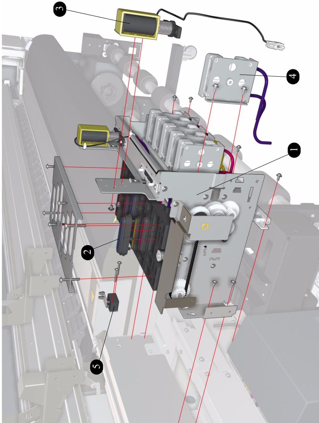
**Figure 11: Capping Assemblies**
