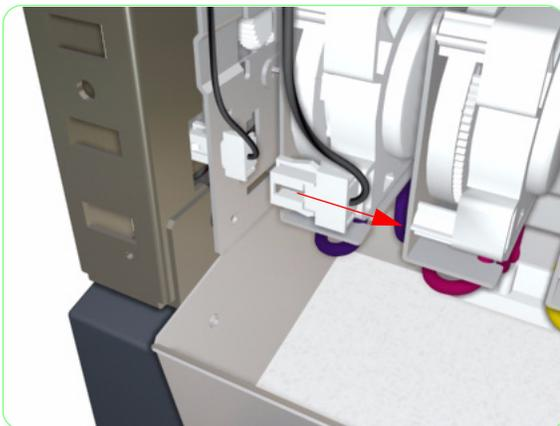
**14.** Release the Solenoid Assembly cable connector from the chassis.
