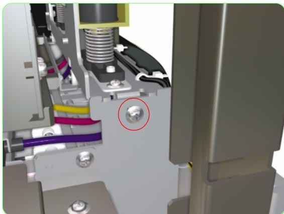
**10.** Remove one screw from each side of the Solenoid Assembly.
