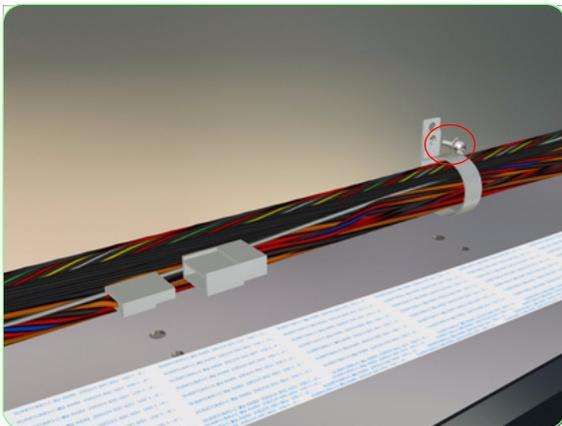
4. Remove one screw that secures the Front Media Sensor to the Bracket.
