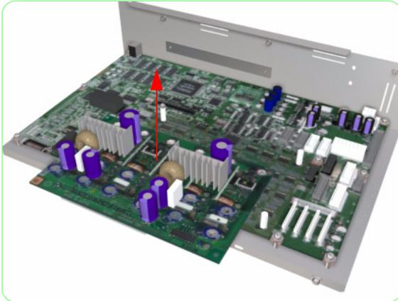
**8.** Remove the Head Relay Board from the Main PCA.
