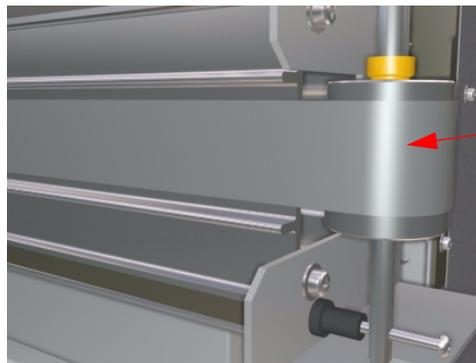
Make sure the Belt stays in the center of the Tension Pulley
