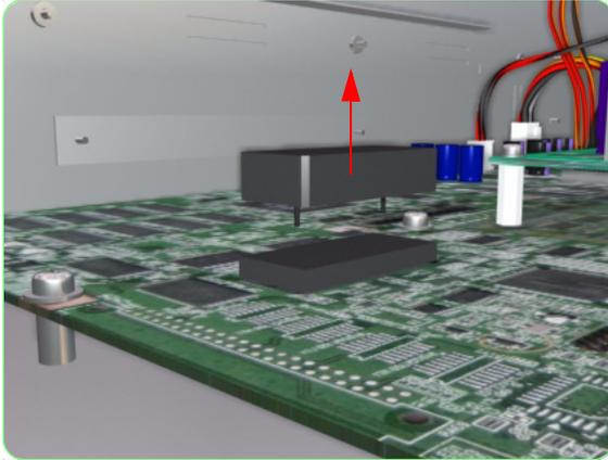
1. Remove the Electronics Module Cover ⇒ Page 8-27.
