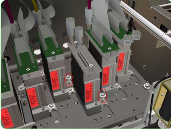
10. Remove two screws that secure the Printhead to the Carriage Assembly.
