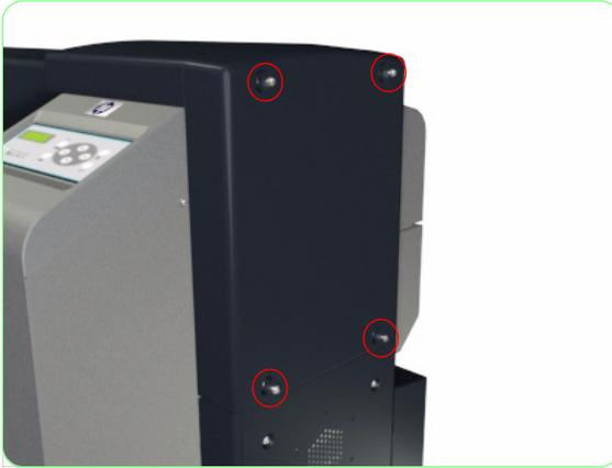
1. Remove four screws that secure the Upper Side Cover to the Printer.
