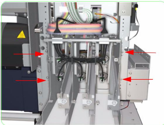
**54.** Attach the subtank to the printer body by hanging the subtank on the top two screws. Then insert the bottom two screws and tighten all four screws.
