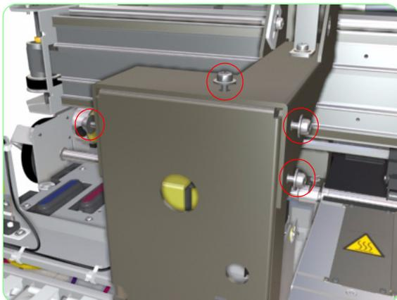
**23.** Remove four screws that secure the Right Capping Frame at the top.
