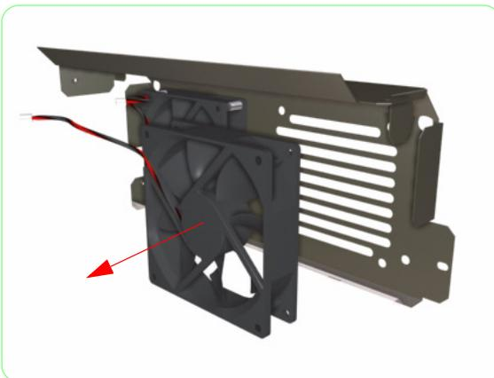
**14.** Remove the Printhead Cooling Fan from the Printhead Cooling Fan Assembly.
