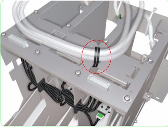
**55.** Secure the tubes to the subtank with the twist-tie.
