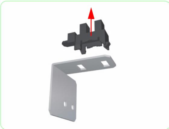
**7.** Unclip the Home Position Sensor from the Support Bracket.
