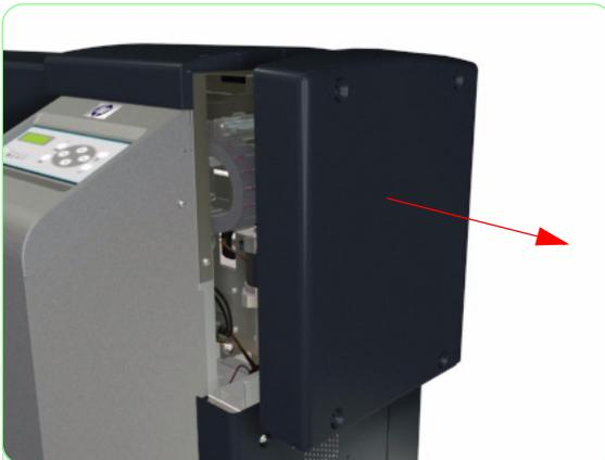
2. Remove the Upper Side Cover from the Printer.
