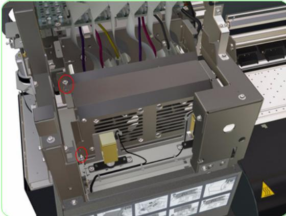
7. Remove two screws that secure the Printhead Cooling Fan Assembly to the Carriage Assembly.
