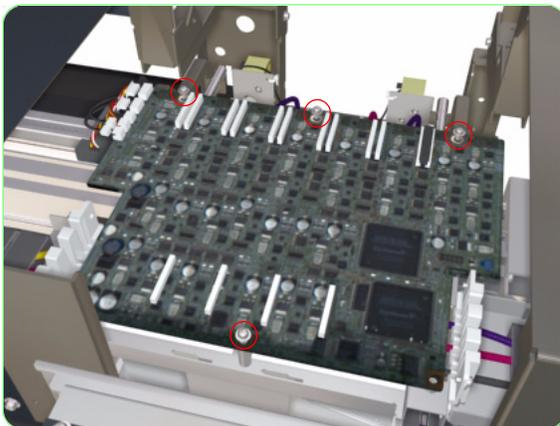
**12.** Remove four screws that secure the Carriage PCA to the Carriage Assembly.
