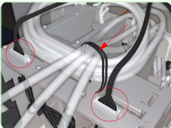
**60.** Connect the cables to the subtank and ensure that the tubes are secured with a twist-tie as shown in the image.
