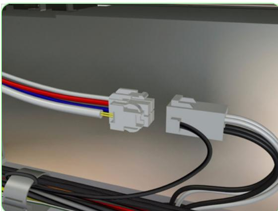
3. Disconnect the Front Heater Cable from the Front Heater.
