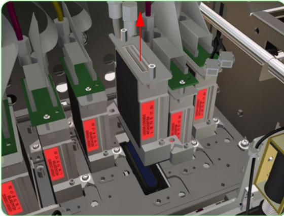
11. Remove the Printhead from the Carriage Assembly.
