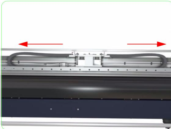
**49.** After securing the tubes, slide the carriage PCA back and forth along the length of the printer to ensure that the highest point of the cable carrier is the point at which the ends are attached to the carriage PCA.
