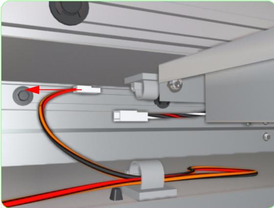
3. Remove 3 screws that secure the Vacuum Fan to the Printer.
