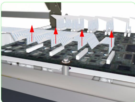
9. Disconnect the Trailing Cable from the Carriage PCA.
