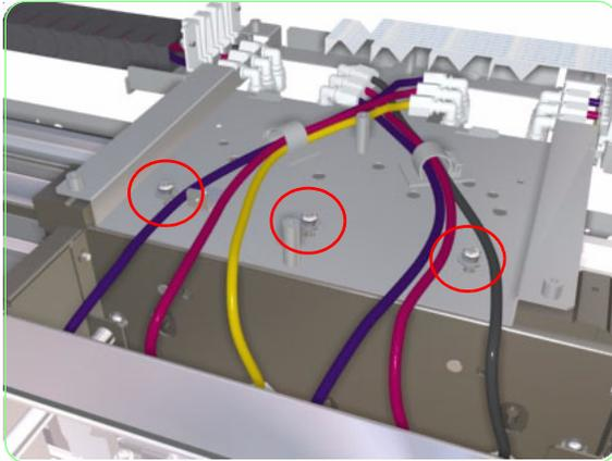
**19.** Remove the three screws that are used to secure the bracket assembly to the headbase.
