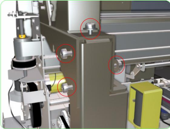
**19.** Remove four screws that secure the Left Capping Frame at the top.
