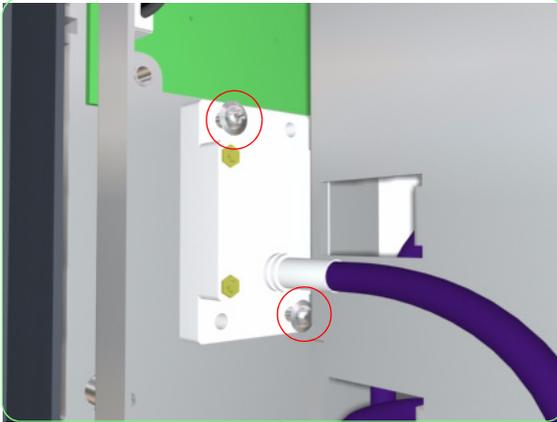
6. Remove the two screws that are used to secure the Needle.
