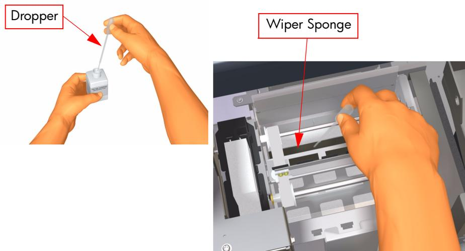
**Make sure that the Wiper Cleaning Liquid does not drip on to other parts of the Printer. If the Wiper Cleaning Liquid drips on to the Belt or any nearby Sensors, this could cause serious damage to the Printer.**
