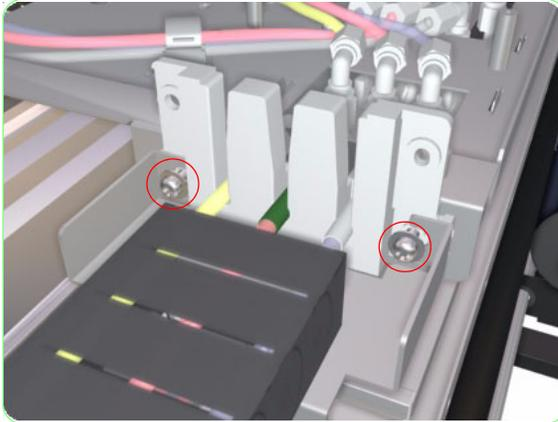
**19.** Remove the two screws used to secure the cable carrier to the guide bracket and carriage.
