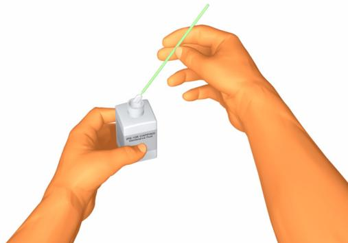
**Make sure that you use the Cap Cleaning Liquid and NOT the Wiper Cleaning Liquid to clean the Capping Unit, otherwise you could cause damage to the Printheads.**
