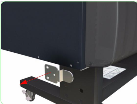
2. Remove the Hinge from the Printer.
