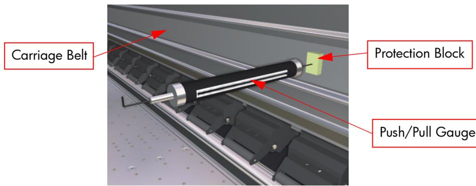
**In order not to damage the Carriage Belt, please use a protection block between the Push/Pull Gauge and the belt.**
