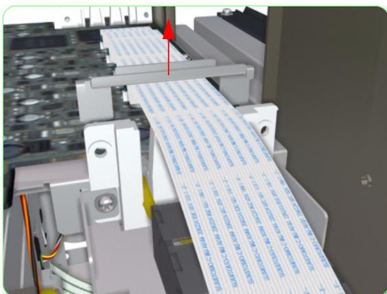
8. Remove the metal bracket from the Carriage Assembly.
