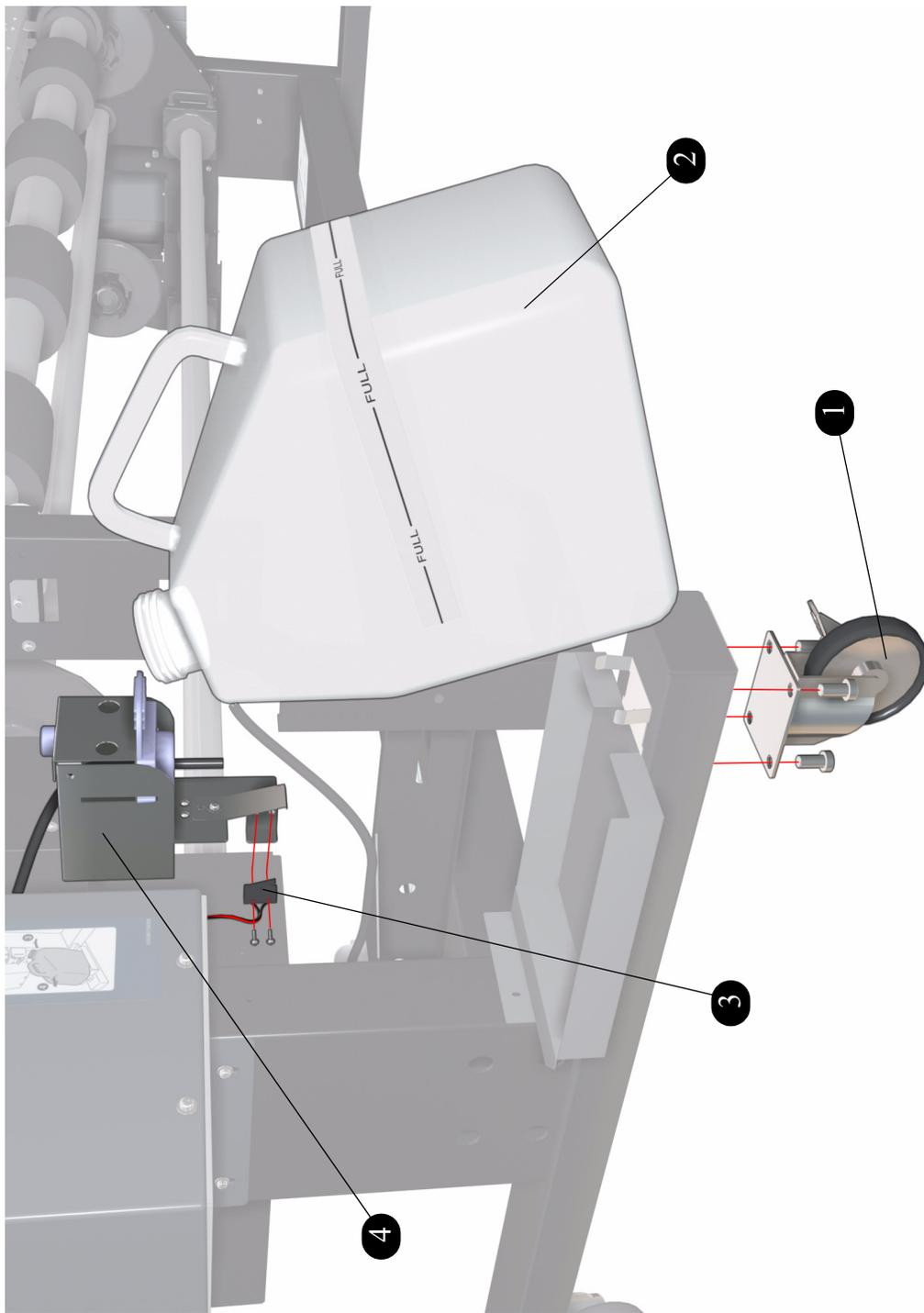
**Figure 14: Printer Stand and Waste Bottle**
