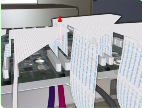
**10.** Disconnect ALL the Printhead Connector Cables from the Carriage PCA.
