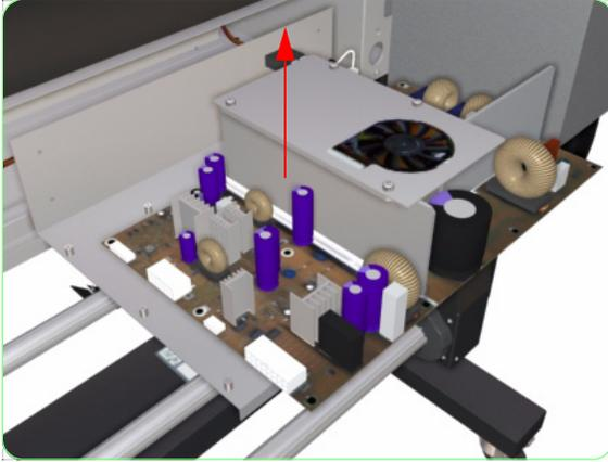
8. Remove the Power Supply Unit from the Support Tray.
