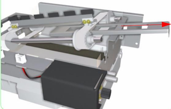
**12.** Remove the metal plate from the Wiping Station.
