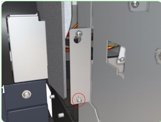
7. Remove one screw from each side of the Subtank Station.
