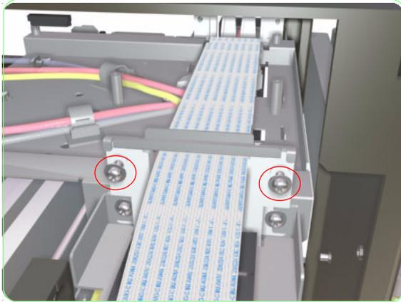
**13.** Remove the two screws that are used to secure the cable bracket to the carriage.
