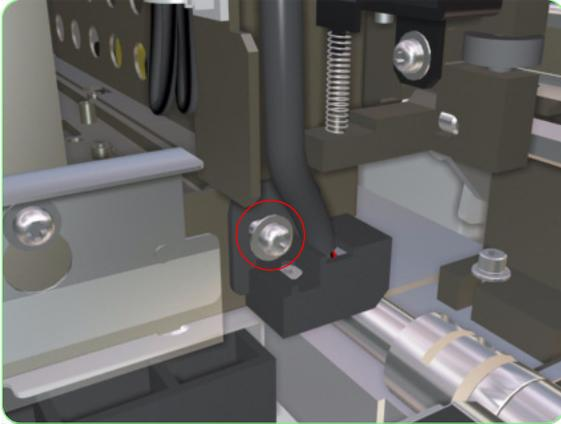
5. Remove one screw that secures the Line Sensor to the Carriage PCA.
