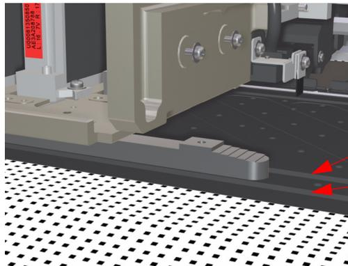
Position tool between the two grooves in the Center Platen
