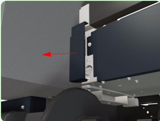
2. Remove the Left Electronics Module Side Trim from the Printer.
