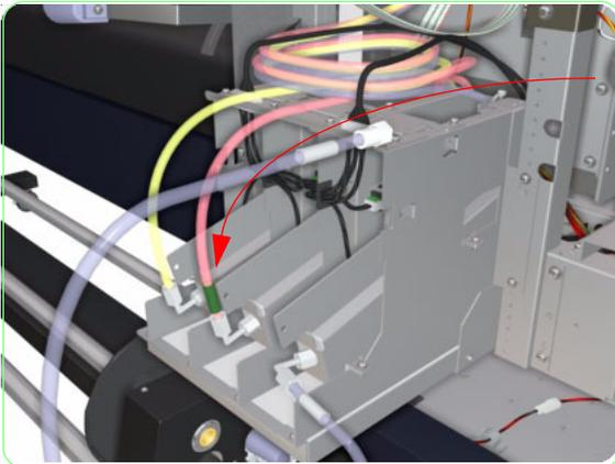
**30.** When the top part of the tube has drained, pull the tube through to the front side of the printer and continue to drain the tube into the waste bottle.
