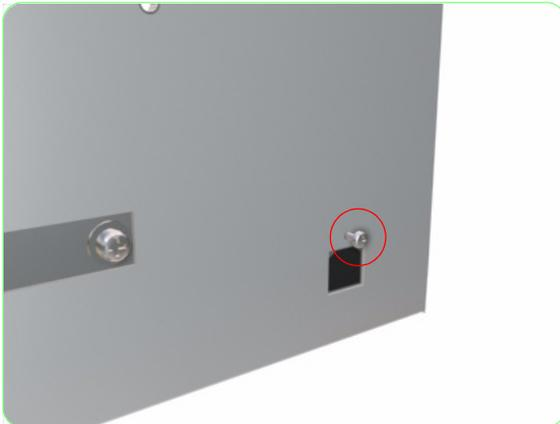
4. Remove three screws that secure the Main PCA Tray to the Printer from the front.
