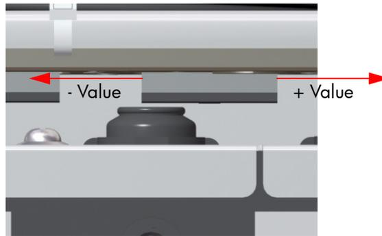
**The value of the Cap Position should never be set as 0.0 mm as this means that the Cap Position has not been adjusted and will not work.**
