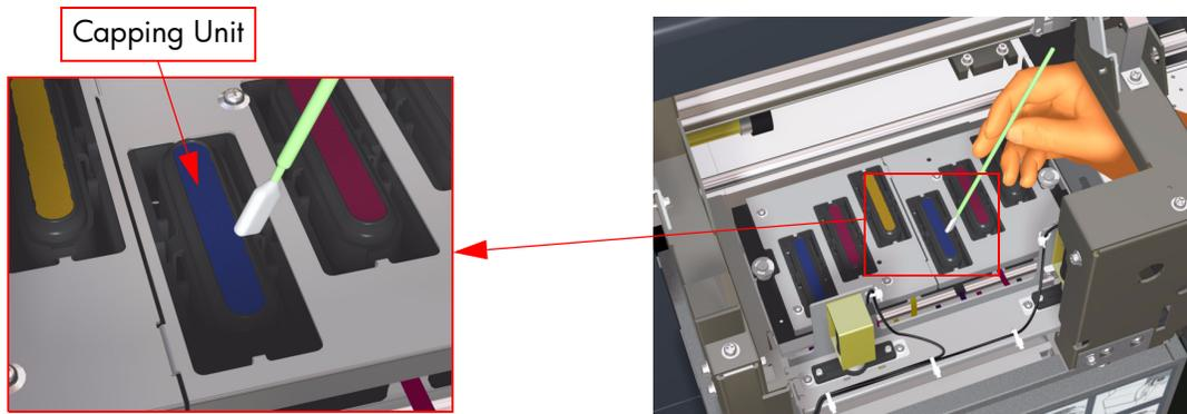
**Make sure that the Cap Cleaning Liquid does not drip on to other parts of the Printer. If the Cap Cleaning Liquid drips on to the Belt or any nearby Sensors, this could cause serious damage to the Printer.**
