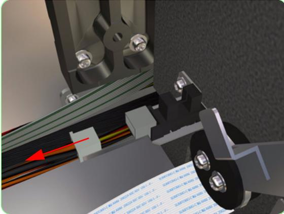
3. Remove one screw that secures the Media Lever Sensor to the Bracket.
