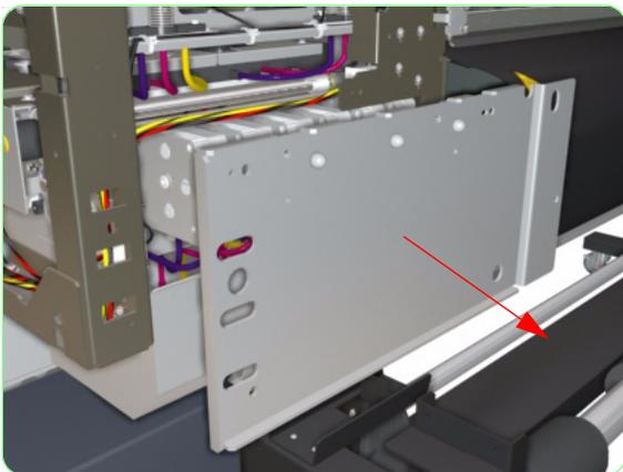
**10.** Remove the metal plate from the chassis.
