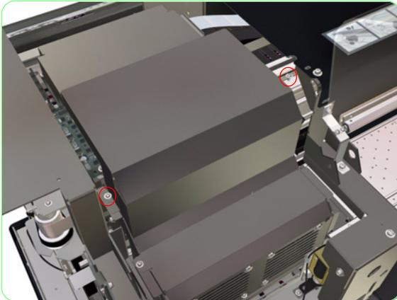
5. Remove the Carriage Cover from the Carriage Assembly.
