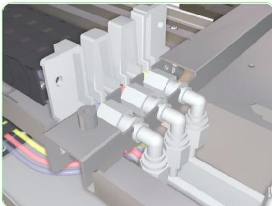
**18.** Loosen the plastic nuts and disconnect the three tubes where they connect at the guide bracket. (Steps 18 - 30 apply to both sides of the printer.)
