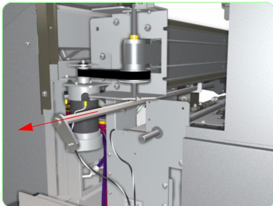
11. Pull out the Pinchwheel Cam until the Pinchwheel Assembly that you want to remove can be accessed.
