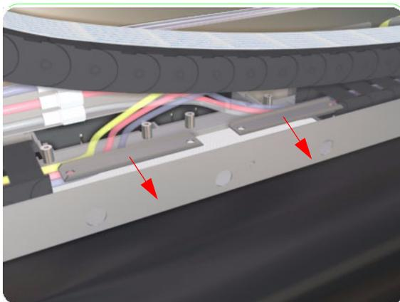
**17.** Remove the tube-holder brackets.
