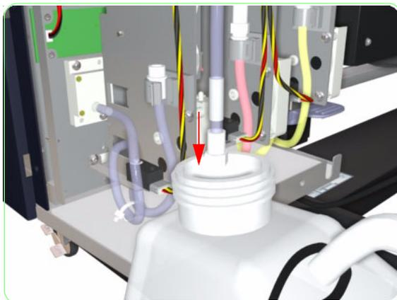
**28.** Drain the upper part of the tube into the waste bottle.
