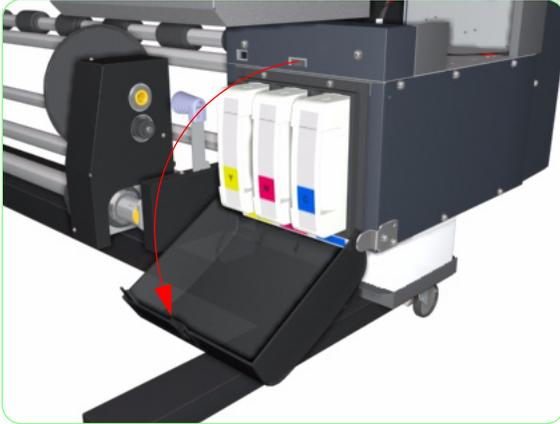
3. Remove two screws that secure the metal cover to the Ink Supply Station.
