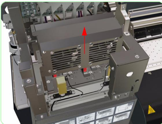
8. Raise the Printhead Cooling Fan Assembly slightly.
