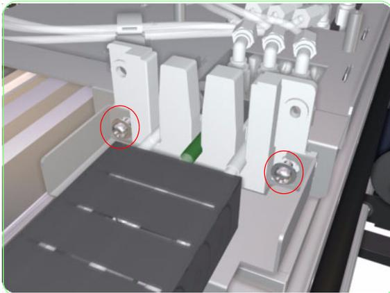
**45.** Use two screws to attach the two guide brackets to each side of the Carriage PCA.
