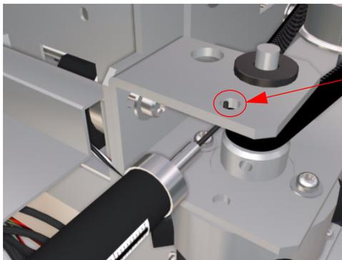
Hook the Push/Pull Gauge onto this hole
