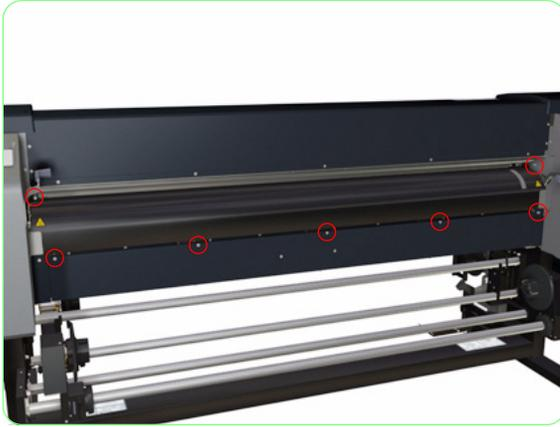
1. Remove seven screws that secure the Front Heater to the Printer.
