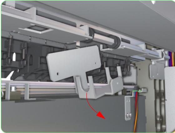
**15.** Remove the Pinchwheel Bracket from the Printer.
