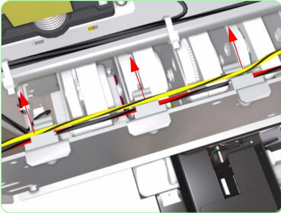
**9.** Release ALL the cables from the cable clips.
