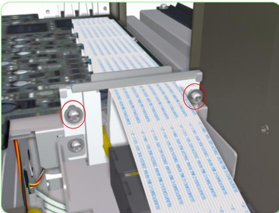
**12.** Remove two screws that secure the metal bracket to the Carriage Assembly.
