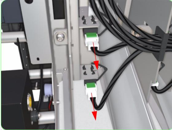
**12.** Disconnect the Subtank Sensor cables.
