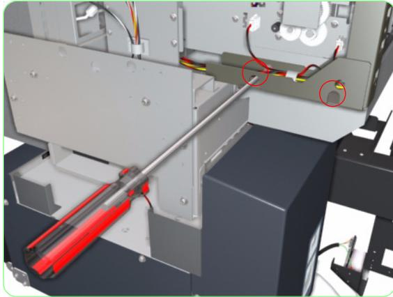
**11.** Remove two screws that secure the metal cover to the side of the Printer.
