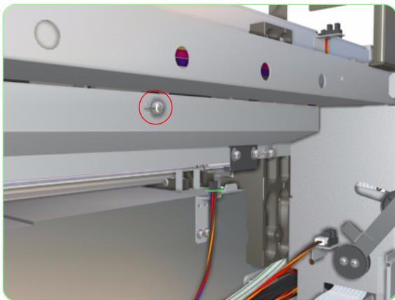
**12.** Remove four screws that secure the Metal Cover.
