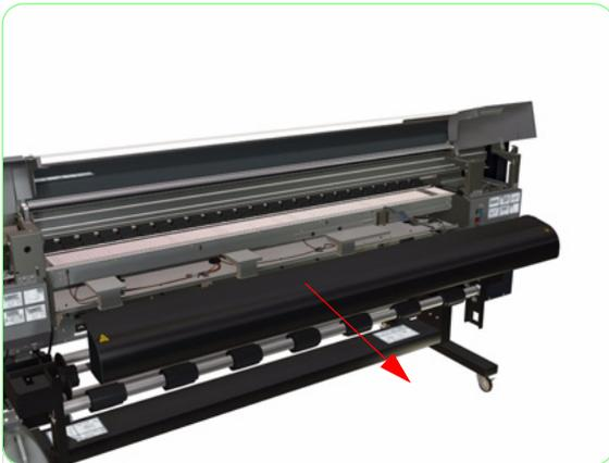
**5.** Remove the Rear Heater from the Printer.
