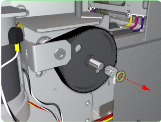
6. Remove the Spring and Washer from the Paper-Axis Gear shaft.
