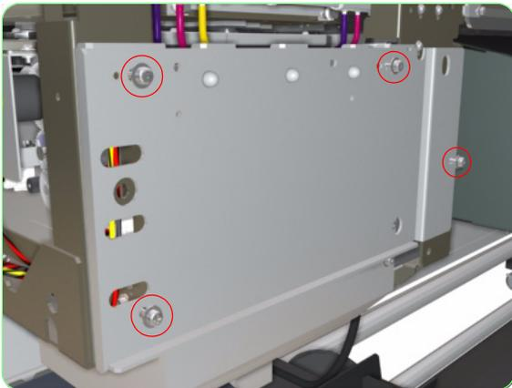
**9.** Remove four screws that secure the metal plate to the chassis.
