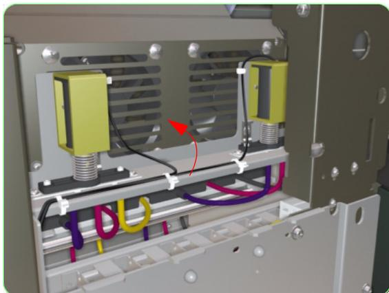
**11.** Rotate the Solenoid Assembly so that the Right Rear Cover Sensor can be accessed.
