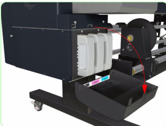
3. Open the Ink Cartridge Door and remove from the Printer.
