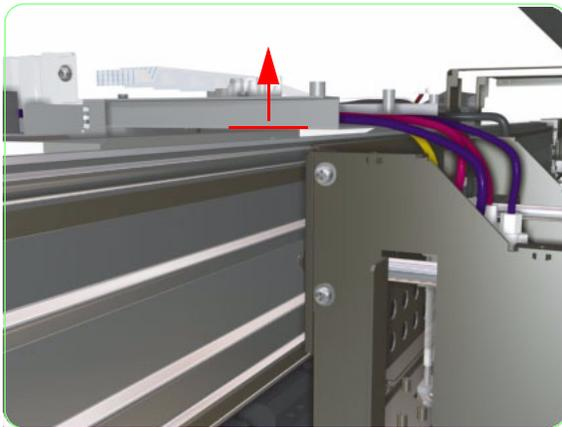
**Move the carriage in a manner such that the bracket assembly does not touch the T-fence. One solution is to put an object with a 15 to 30mm diameter (such as a screwdriver handle) under the bracket assembly, as shown in the following two images.**
