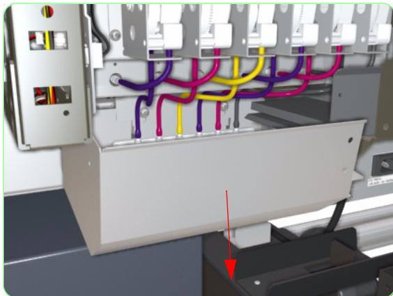
**13.** Pull the metal cover down slightly so that the Priming Tubes are exposed.
