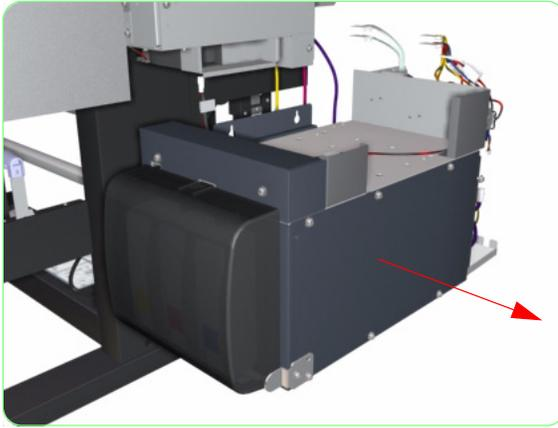
9. Remove the Ink Supply Station from the Printer.
