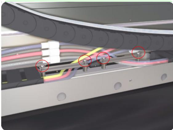
**16.** Remove the two screws from each of the tube-holder brackets.
