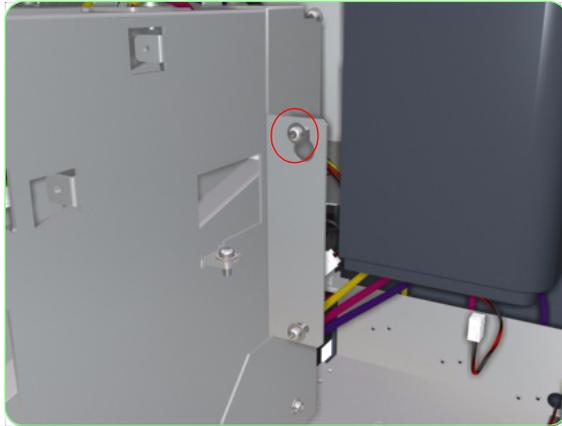
6. Loosen one screw from each side of the Subtank Station.
