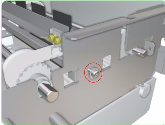
**10.** Remove one screw that secures the metal plate.
