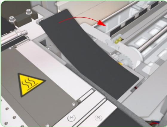
**12.** Remove the Black Cover that is stuck over the hole in the Wiping Station.
