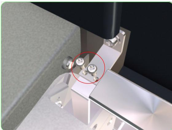
2. Remove two screws that secure the Rear Cover to the left hinge.
