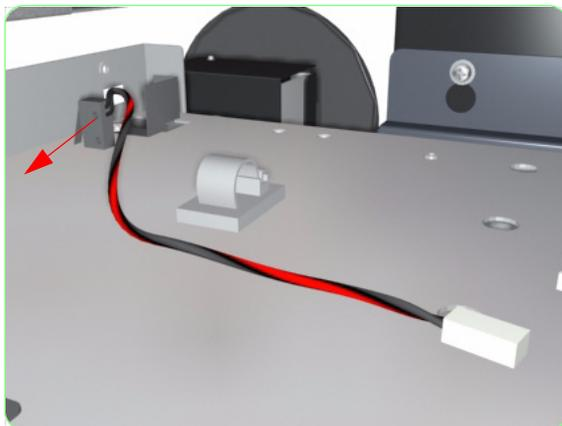
**7.** Remove the IC Door Sensor from the Ink Supply Station.
