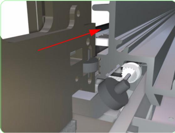
1. At the Y-rail edge, squeeze the spring and install the carriage assembly by sliding it onto the printer chassis.
