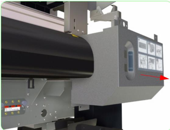
6. Remove the Lower Wiping Cover from the Printer.
