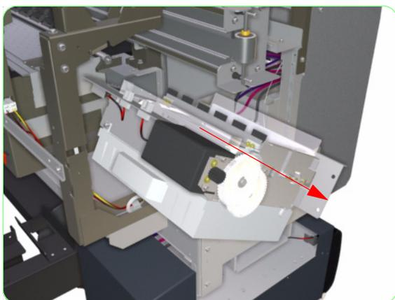
**15.** Remove the Wiping Station from the Printer.
