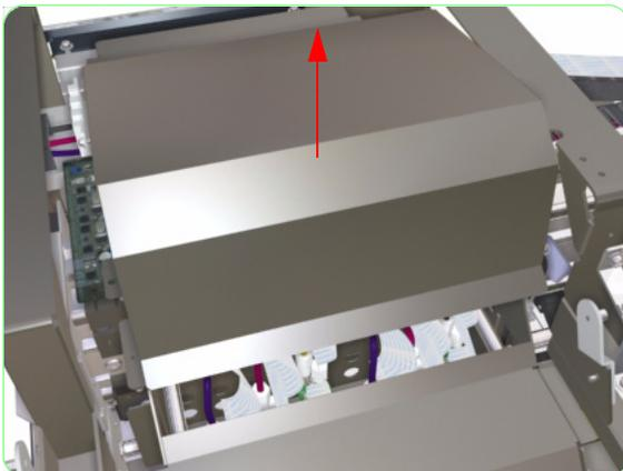
9. Remove the Carriage Cover from the Carriage Assembly.
