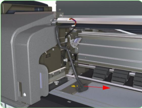
6. Remove the Line Sensor from the Printer.
