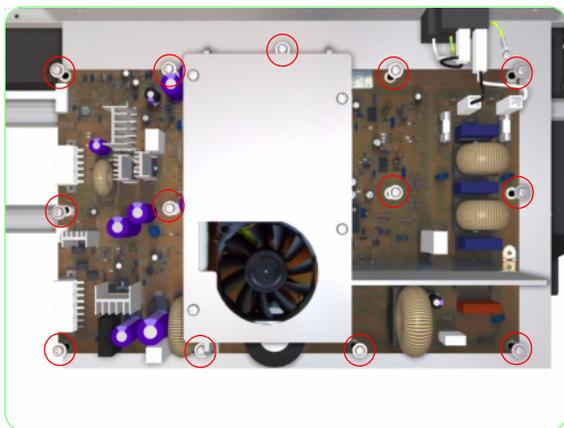
7. Remove 13 screws that secure the Power Supply Unit to the Support Tray.
