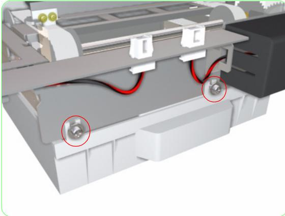
8. Unclip the Wiper Cleaning Assembly from the Wiping Station Assembly.
