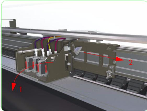
**20.** Remove the three screws that you loosened in step 15, and then move the headbase slightly toward the paper-output side of the printer so that you can then slide the carriage base toward the wiping side.
