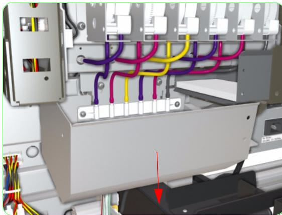
**15.** Pull the metal cover down slightly so that the Priming Tubes are exposed.
