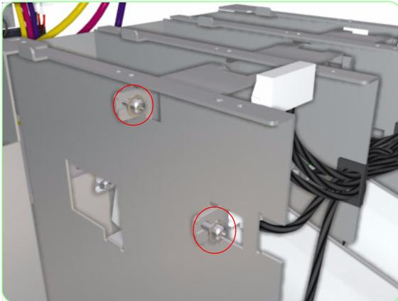
**13.** Remove two screws that secure the Subtank Sensors Assembly to the Subtank Station.
