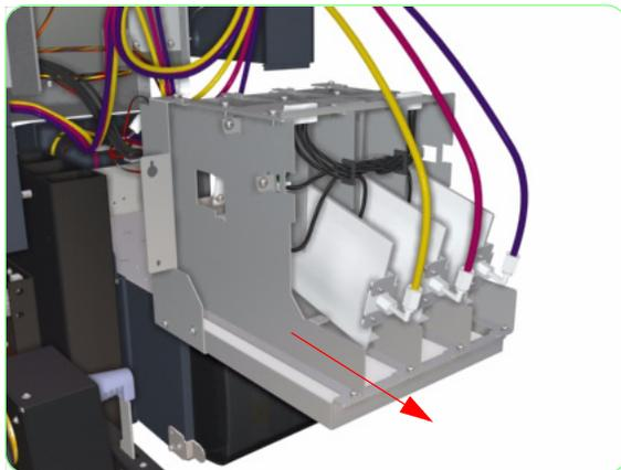
8. Carefully pull out the Subtank Station slightly.
