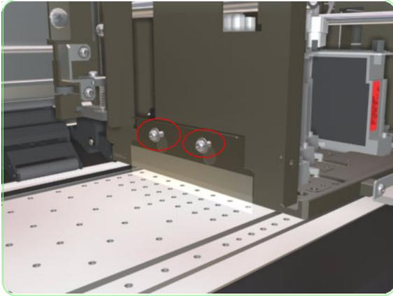
**13.** Remove the two screws that are used to secure the plate assembly.
