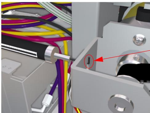
Hook the Push/Pull Gauge onto this hole
