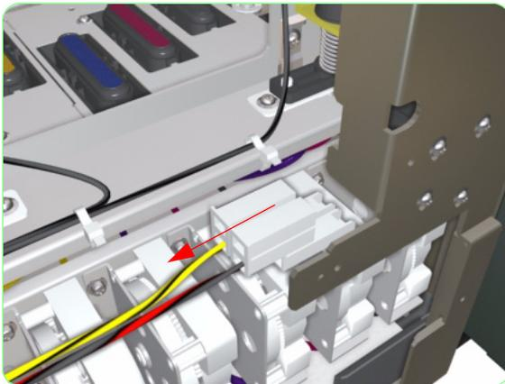
**26.** Disconnect the Cable from the Right Rear Cover Sensor.
