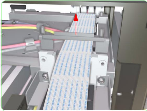
**14.** Remove the cable bracket.
