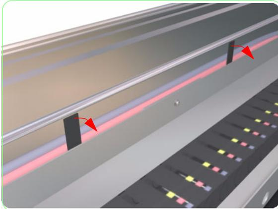
**23.** Bend out the tabs that are used to secure the ink-supply tubes.
