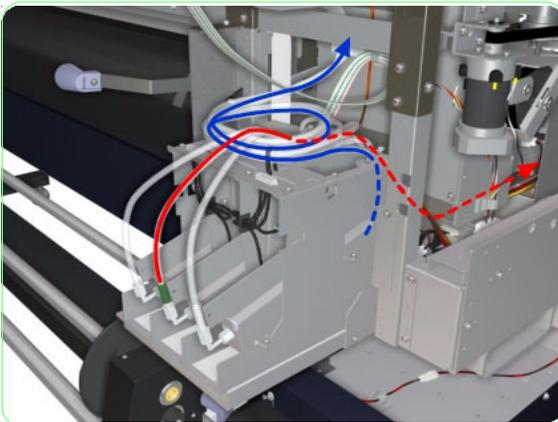
**57.** Feed the disconnected end of the subtank tube to the supply-pump side of the printer.
