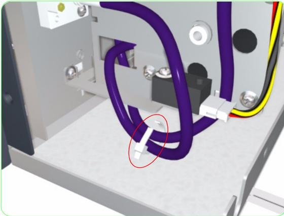
4. Disconnect the Ink Pump Assembly cable.
