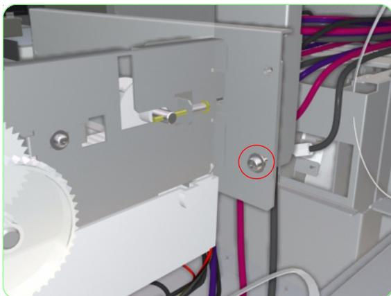
**14.** Remove one screw that secures the Wiping Station to the chassis.
