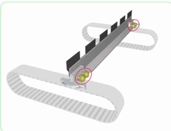
**14.** Remove four screws that secure the Wiper Blade to the Wiper Belts.
