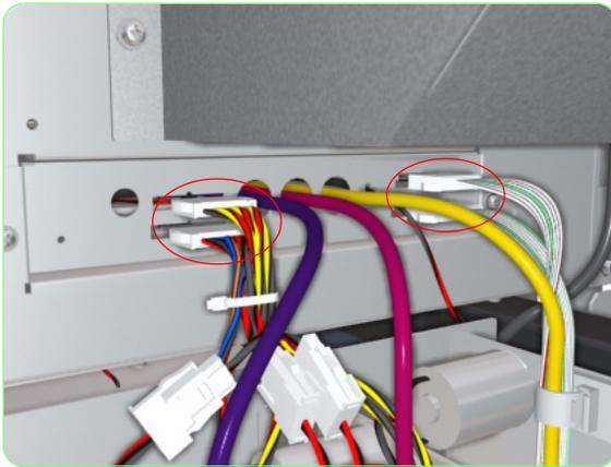
5. Remove the Ink Pump Tubes (for ALL three colors) from the cable clip.
