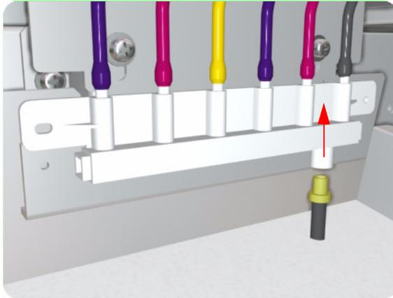
**31.** Disconnect the Waste Tube to the Capping Tubes Bracket.
