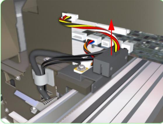
7. Remove the Encoder Sensor from the Printer.
