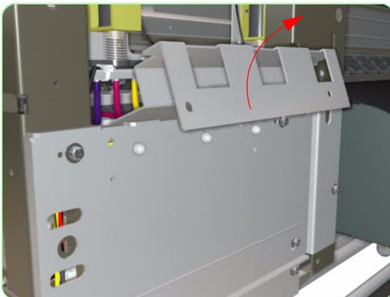
9. Remove the metal bracket from the Printer.
