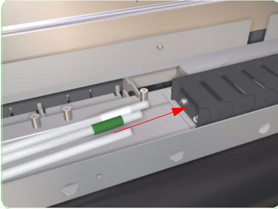
**40.** There is a narrow end and a wide end to each supply tube. Thread the *narrow ends* of three tubes through one end of the cable carrier.
