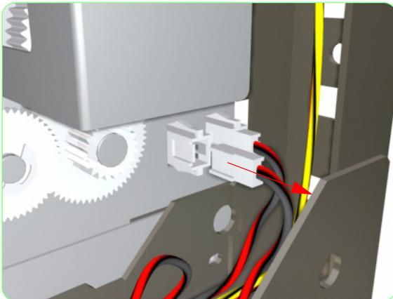
**13.** Disconnect the Solenoid Assembly cable.
