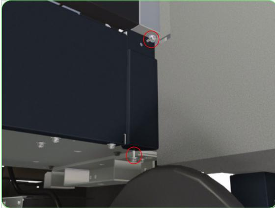
4. Remove the Right Electronics Module Side Trim from the Printer.
