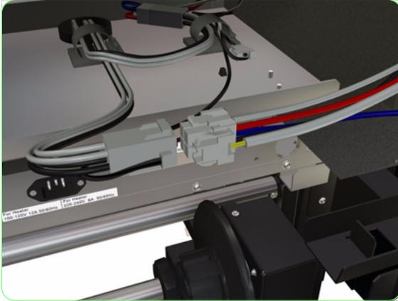
**4.** Disconnect the Rear Heater Cable from the Rear Heater.
