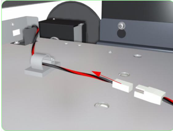
**5.** Disconnect the IC Door Sensor cable.
