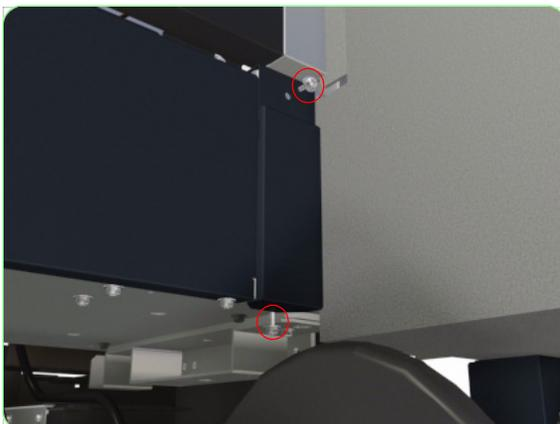
3. Remove two screws that secure the Right Electronics Module Side Trim to the Printer.
