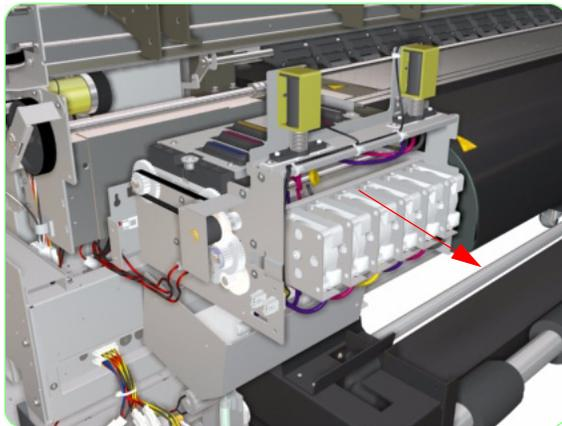
**32.** Remove the Capping Station from the Printer.
