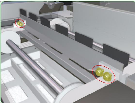
3. Remove four screws that secure the Wiper Blade to the Wiper Belts.
