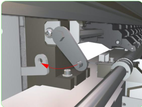
10. Release the Linkage from the Pinchwheel Cam.
