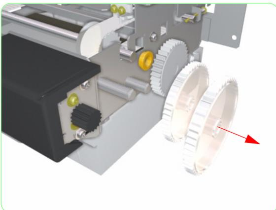
8. Remove the Gears from the Wiping Station.
