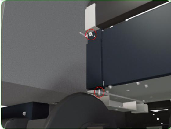
4. Remove the Left Electronics Module Side Trim from the Printer.
