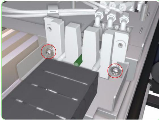
**48.** Use four screws to attach the two cable holder plates.
