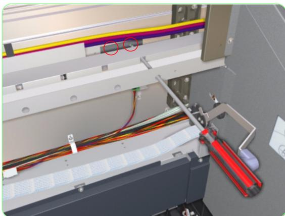
**14.** Remove two/three screws that secure the Pinchwheel Bracket (that secures the Pinchwheel Assembly that you want to remove).
