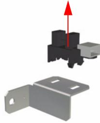
5. Remove the Media Lever Sensor from the Bracket.
