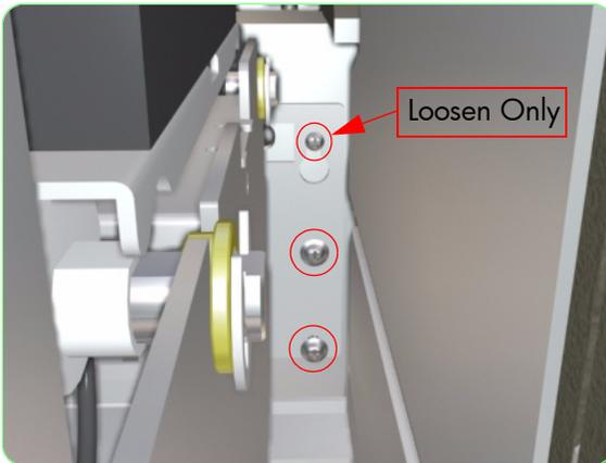
**29.** Loosen one screw (from the top) and two screws that secure the Capping Station.
