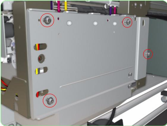
**11.** Remove four screws that secure the metal plate to the chassis.
