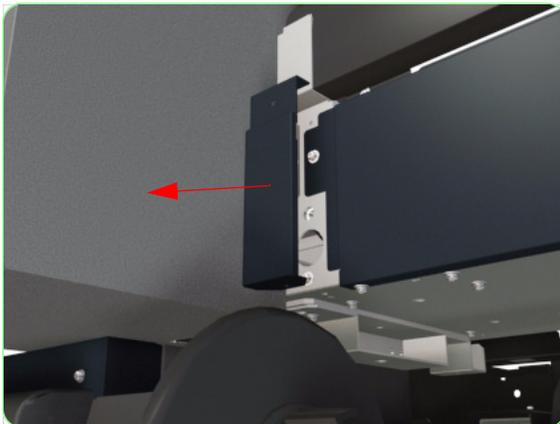
5. Remove two screws that secure the Left Subtank Cover to the Printer.
