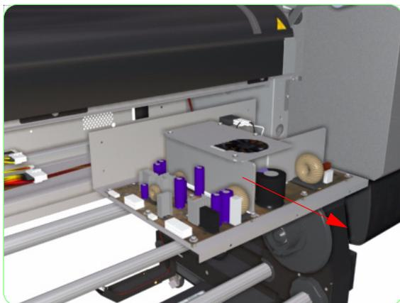
5. Remove the Power Supply Unit (including the Support Tray) from the Printer.
