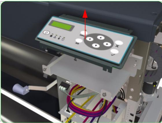
**7.** Remove the Front Panel from the Printer.
