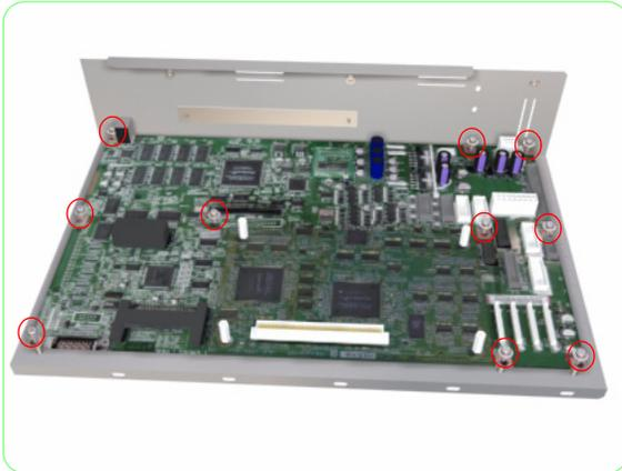
**9.** Remove 10 screws that secure the Main PCA to the Tray.
