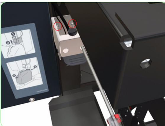
3. Remove two screws that secure the Waste Bottle Bracket to the Printer.
