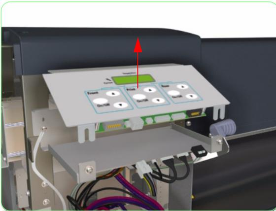
7. Remove the Heater Panel from the Printer.
