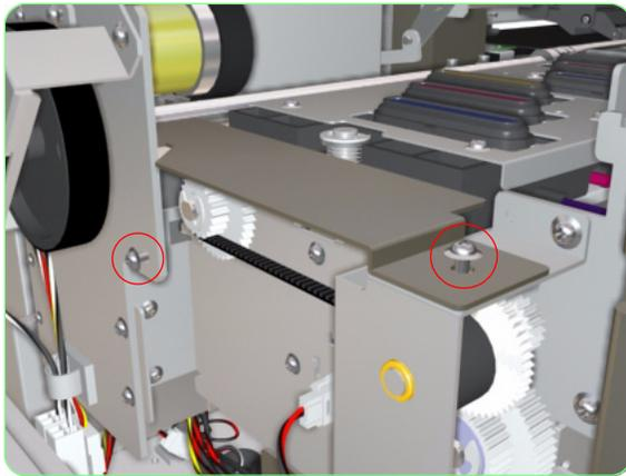
**16.** Remove two screws that secure the metal bracket to the Capping Station.
