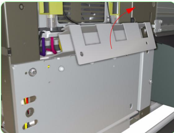
7. Remove the metal bracket from the Printer.
