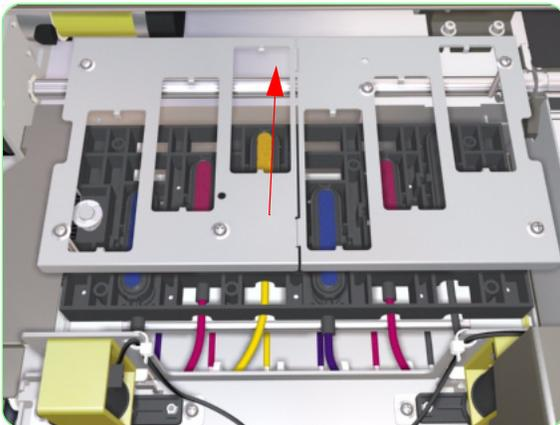
5. Release the Capping Unit and remove from the Capping Station.
