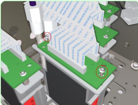
6. Remove two screws that secure the Printhead Connector Assembly to the Printhead.
