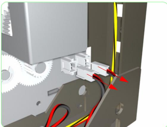
**18.** Disconnect the Capping Station cables.
