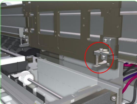
**27.** Remove the carriage base assembly by squeezing the spring and sliding the carriage base off of the printer chassis.
