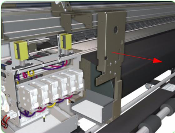
**27.** Remove the Right Capping Frame from the Printer.
