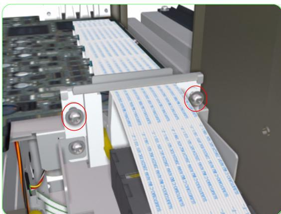
7. Remove two screws that secure the metal bracket to the Carriage Assembly.
