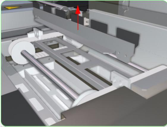
4. Remove the Wiper Blade from the Wiper Belts.
