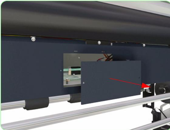
2. Remove the Firmware Access Cover from the Printer.
