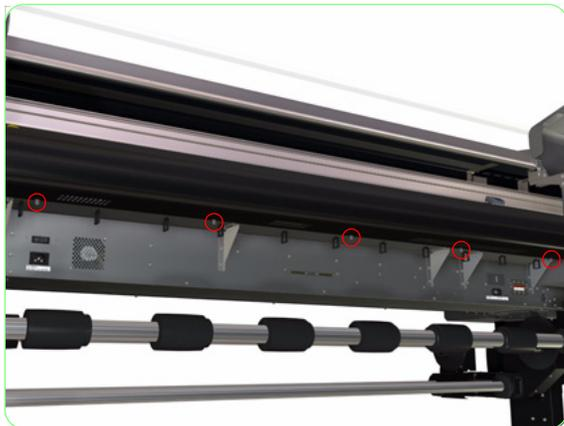
1. Remove five screws that secure the Rear Heater to the Printer.
