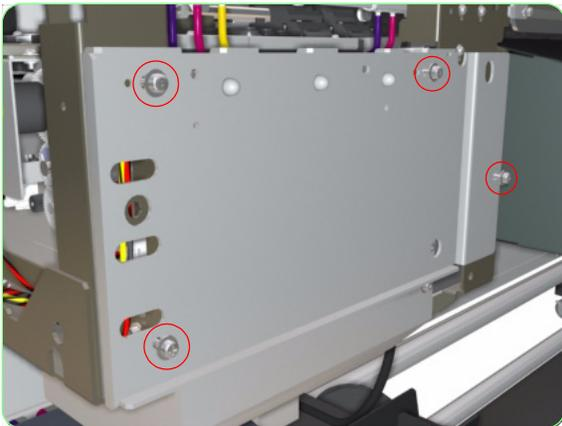
**10.** Remove four screws that secure the metal plate to the chassis.
