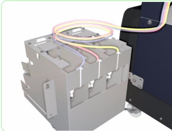
**37.** Remove the subtank and place it on the floor or on a bench.
