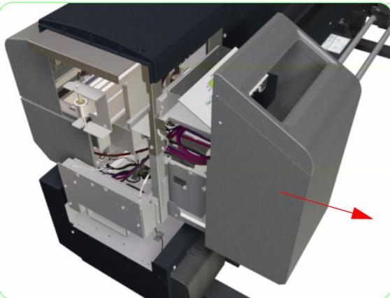
**7.** Remove the Left Subtank Cover from the Printer.
