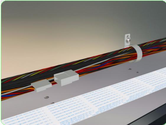
3. Remove one screw that secures the Cable Holder to the Printer.
