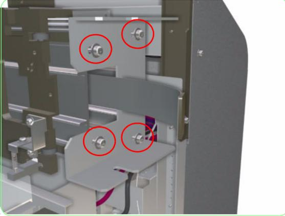
**25.** Remove the four screws that are used to secure the bracket to the printer body.
