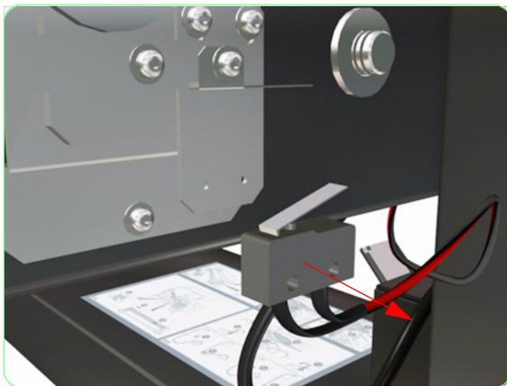
**6.** Remove the End-of-Media Sensor from the Printer.
