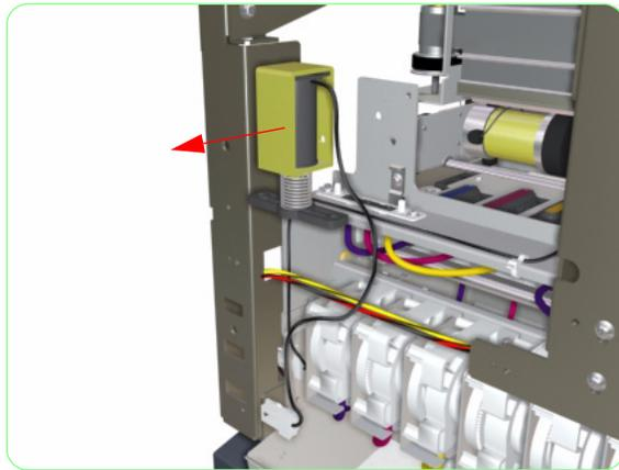
**16.** Remove the Solenoid Assembly from the Capping Station.
