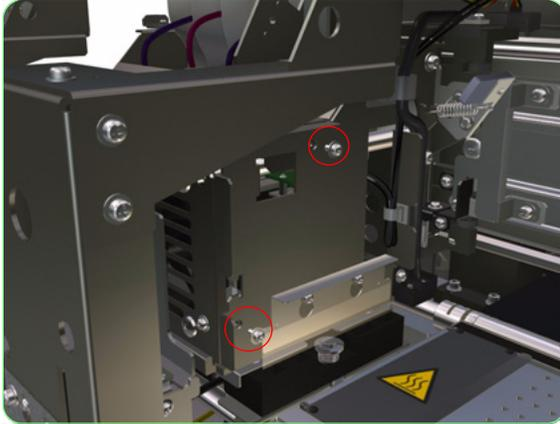
6. Remove two screws that secure the Printhead Cooling Fan Assembly to the Carriage Assembly.
