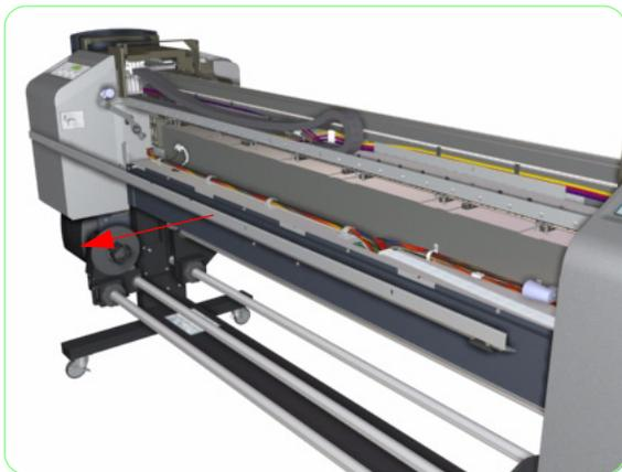
**13.** Remove the Metal Cover from the Printer.
