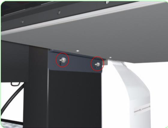
8. Remove two screws that secure the Ink Supply Station to the Printer.
