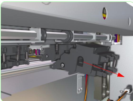
**17.** Remove the Pinchwheel Assembly from the Printer.
