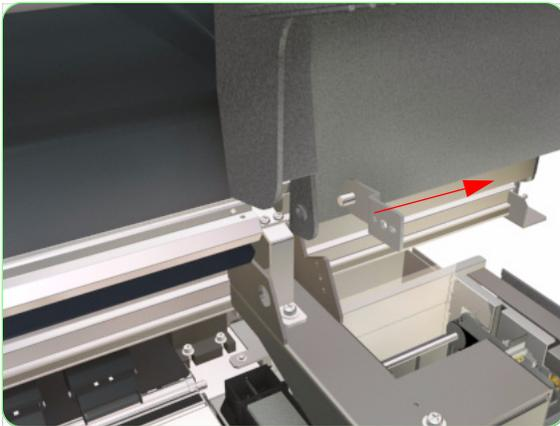
2. Remove the Hinge from the Printer.
