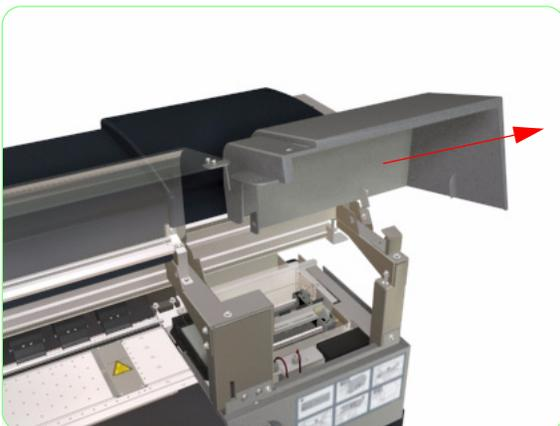
3. Slide the Wiping Door to the right and remove from the Printer.
