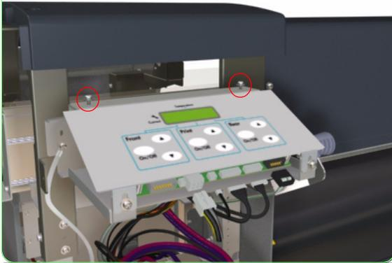
6. Remove two screws that secure the Heater Panel to the Printer.
