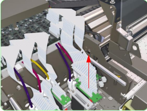
7. Disconnect the Printhead Connector Assembly from the Printhead and remove from the Printer.
