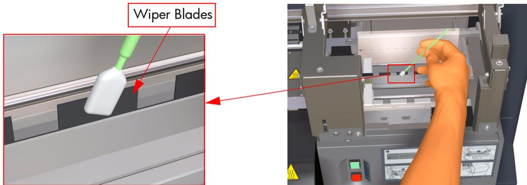
**Make sure that the Wiper Cleaning Liquid does not drip on to other parts of the Printer. If the Wiper Cleaning Liquid drips on to the Belt or any nearby Sensors, this could cause serious damage to the Printer.**
