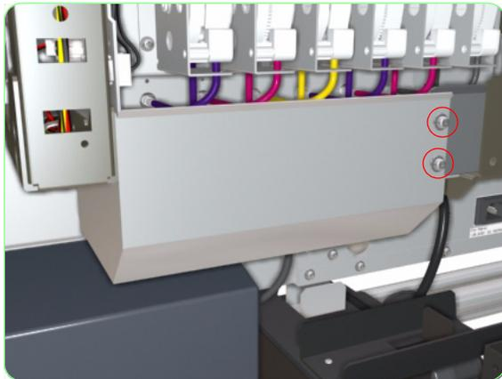
**12.** Remove two screws that secure the metal cover to the front of the Printer.
