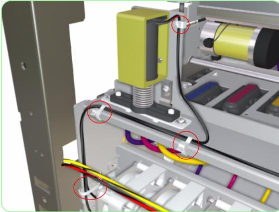
**12.** Cut the cable ties that secure the Solenoid Assembly cable.
