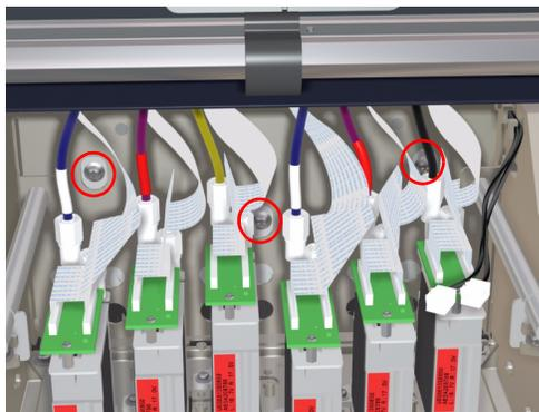
**To loosen the three screws, you will need a 3mm Allen Key that is at least 20 cm long.**
