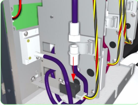
6. Carefully disconnect the Ink Pump Tube (for ALL three colors) from the top side.
