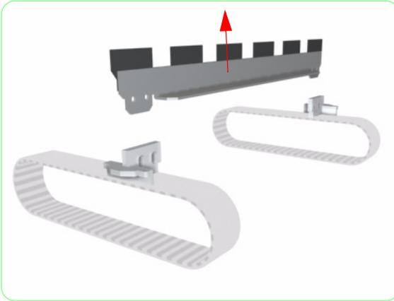
15. Remove the Wiper Blade from the Wiper Belts.
