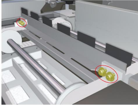
**Make sure that the Carriage is Uncapped before performing the following step. Trying to move the Carriage out of the Capping Station while it is still capped will cause damage to the Printheads.**
