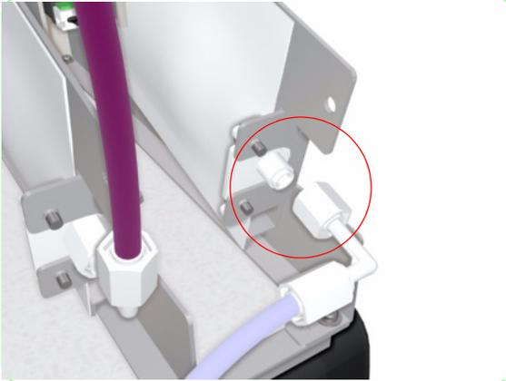
**33.** Loosen the plastic nuts and disconnect the subtank tubes from the subtank.
