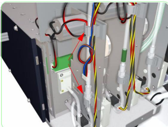
**59.** Clip the tube into the plastic securing clamp.
