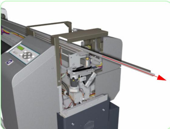
6. Slide the Encoder Strip out of the Printer.
