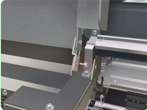
3. Remove the Hinge from the Printer.
