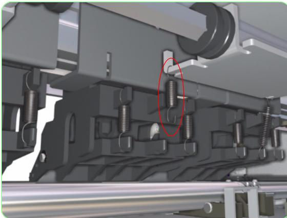
**16.** Release the middle spring from the Pinchwheel Assembly.
