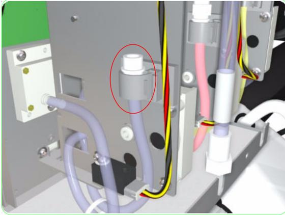
**TIP:** It is helpful to clip the lower part of the tube to the plastic securing clamp to keep it in an upright position while draining the top part of the tube.
