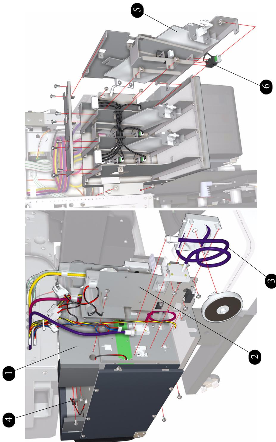
**Figure 13: Ink Supply and Subtank Assemblies**
