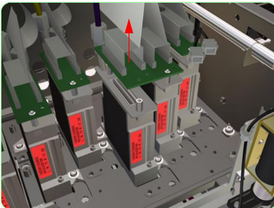
6. Disconnect the Printhead Connector Assembly from the Printhead.
