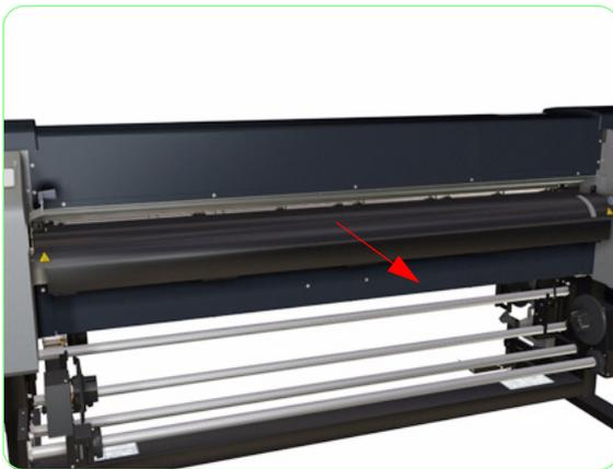
2. Pull out the Front Heater slightly.
