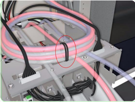
**22.** Undo the twist-ties that are used to secure the ink-supply tubes.
