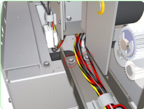
**20.** Remove two screws that secure the Left Capping Frame to the bottom.
