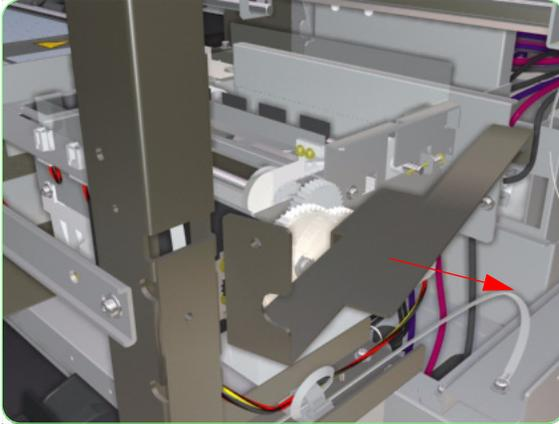
**11.** Remove the Gear Cover from the Wiping Station.
