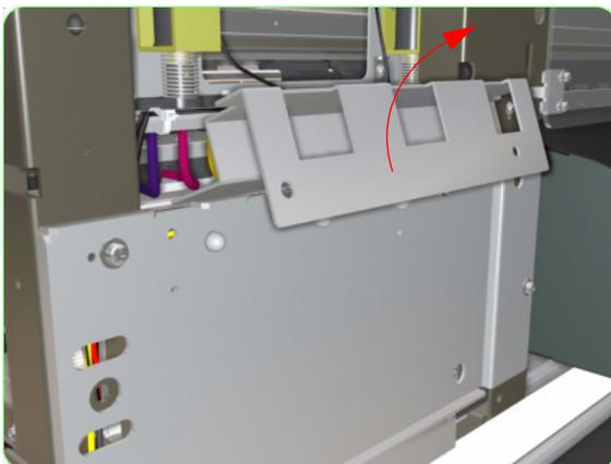
8. Remove the metal bracket from the Printer.
