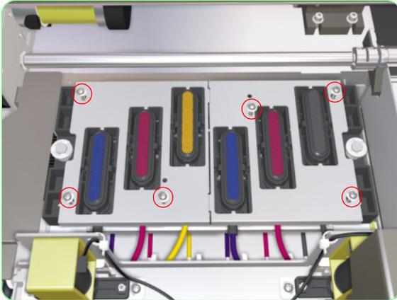
4. Remove the Capping Plates from the Capping Station.
