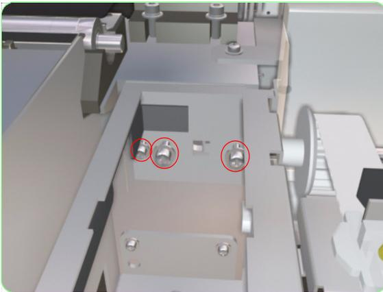
**13.** Remove three screws that secure the Wiping Station to the chassis.
