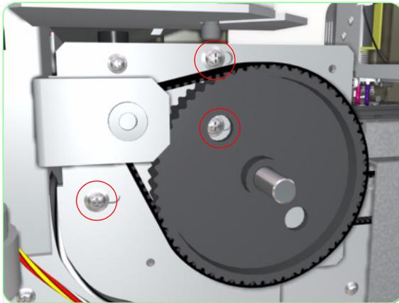
7. Loosen three screws that secure the Paper-Axis Motor Bracket to the Chassis.
