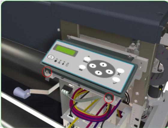
5. Loosen two screws that secure the Front Panel to the Printer.
