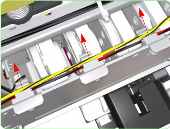
**10.** Release ALL the cables from the cable clips.
