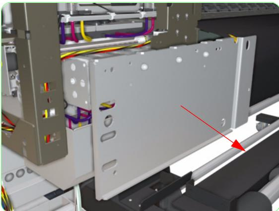
**12.** Remove the metal plate from the chassis.
