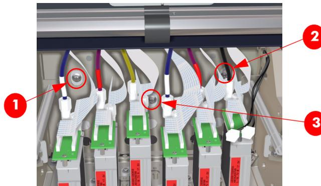
**Before tightening the screws, make sure you place some weight (using your finger) on the front of the Carriage. If this is NOT done, the Carriage will be incorrectly adjusted and could cause some serious Print Quality issues.**
