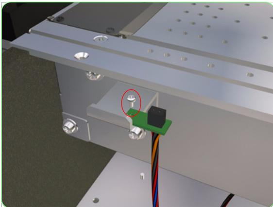
4. Remove the Rear Media Sensor from the Printer.
