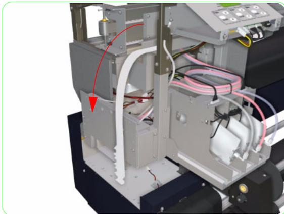
**15.** Lay the cables flat over the side of the printer.
