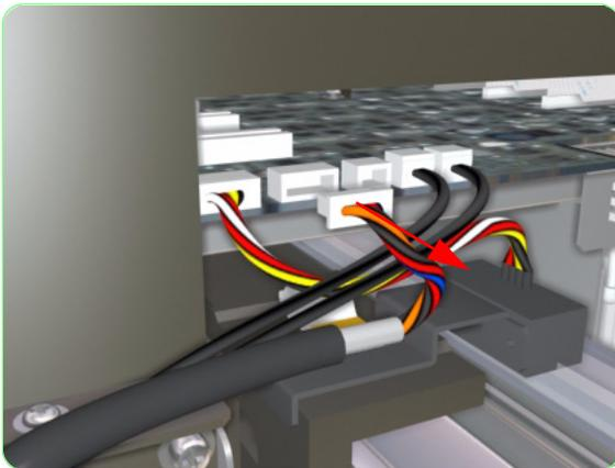
3. Disconnect the Line Sensor Cable from the Carriage PCA.
