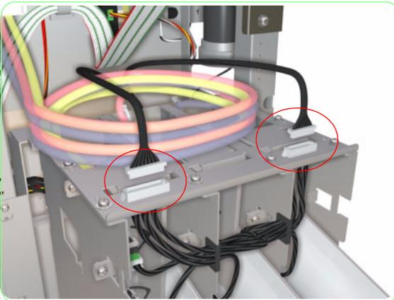
**35.** Remove the electric cable connectors on the subtank.
