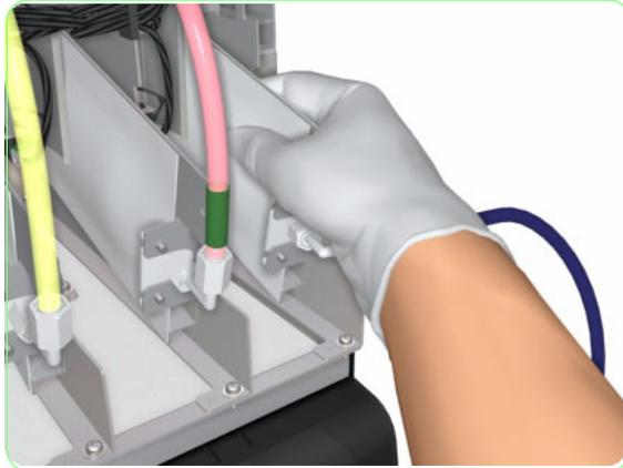
**31.** Press and flatten the subtank to remove as much ink as possible. This is the best way to ensure against creating an inky mess on and around the printer.
