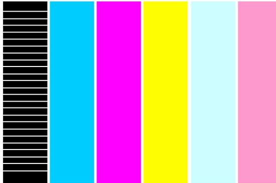
In this situation it is recommended to perform the Printhead Recovery procedure ⇒ Refer to the User's Guide.
