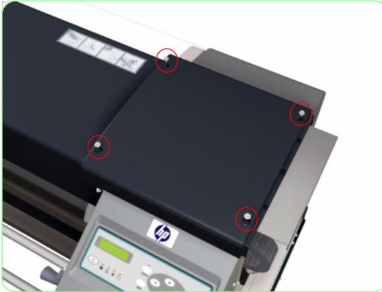
3. Remove the Top Side Cover from the Printer.
