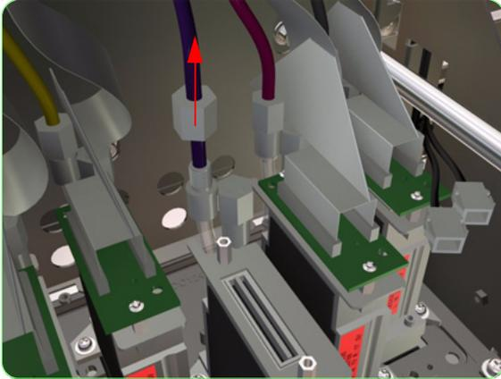
7. Disconnect the Ink Tube from the Printhead.
