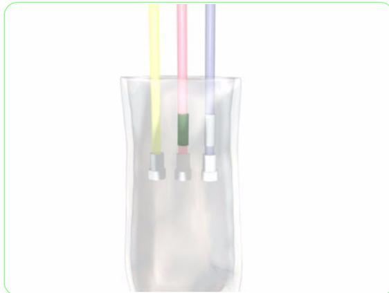
**32.** When the tubes are empty, wrap the ends in plastic to keep them from dripping on and around the printer until you can remove the tubes and dispose of them.
