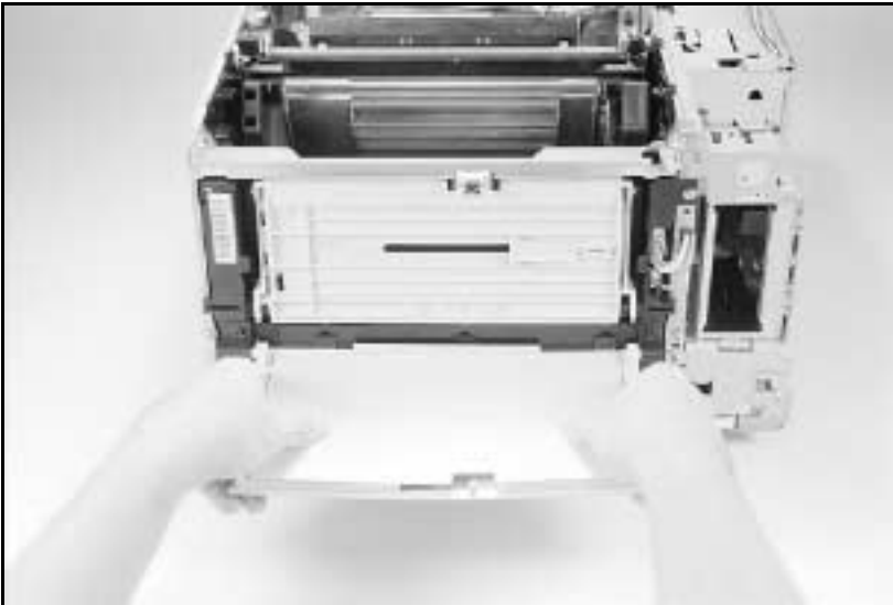
Figure 6-10 Removing the MP Tray Door
