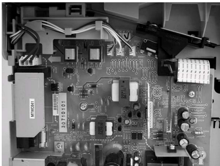
Figure 5-123. Correct routing of the power-supply wire-harnesses
