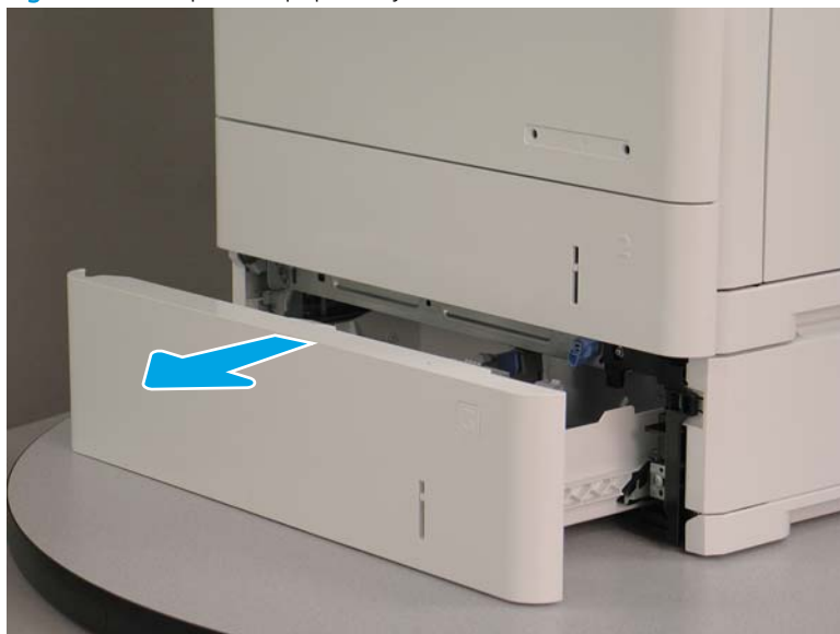
Figure 1-117 Open the paper tray to locate the rollers
