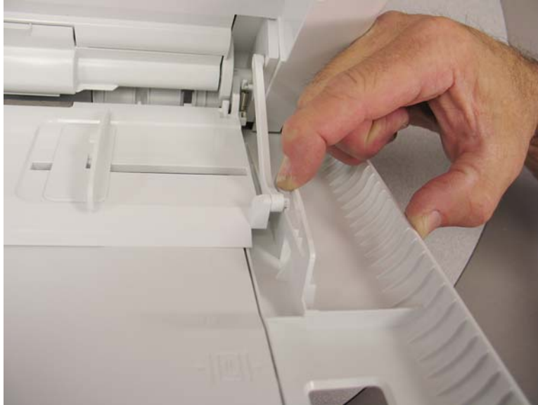
Figure 1-1886 Release the MP tray assembly lift arms from the MP cover
