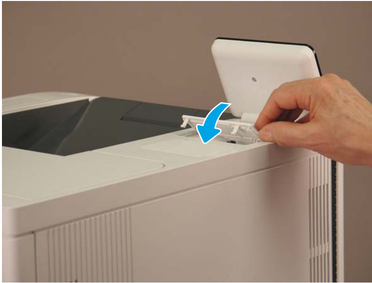
Figure 1-1699 Align the control panel cover and pivot down to install it
