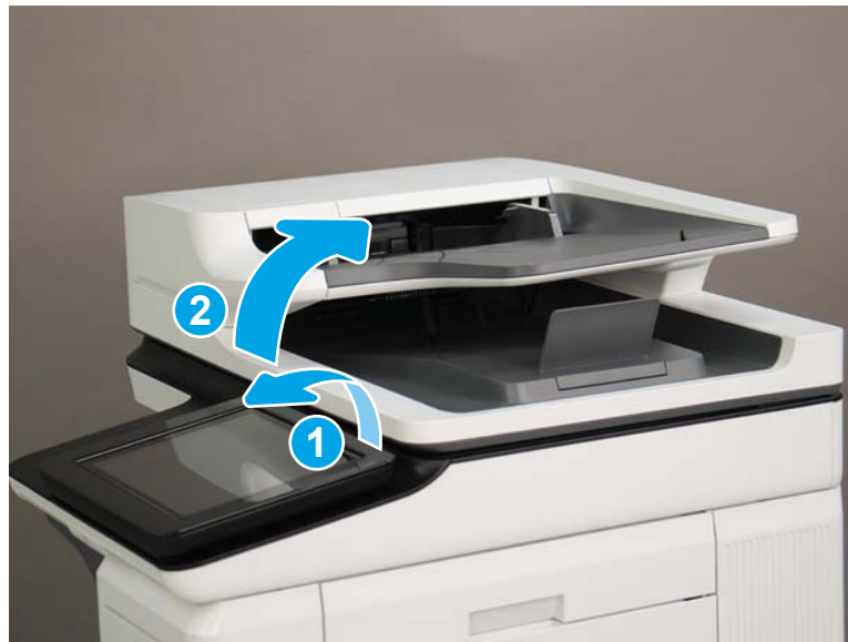
Figure 1-1082 Tilt the control panel and open the document feeder
