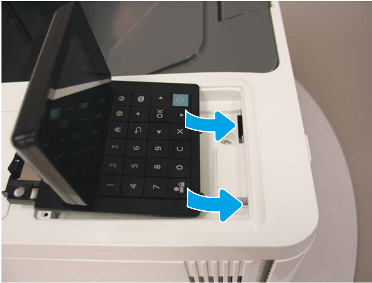
Figure 1-1707 Install the control panel tabs into the printer slots
