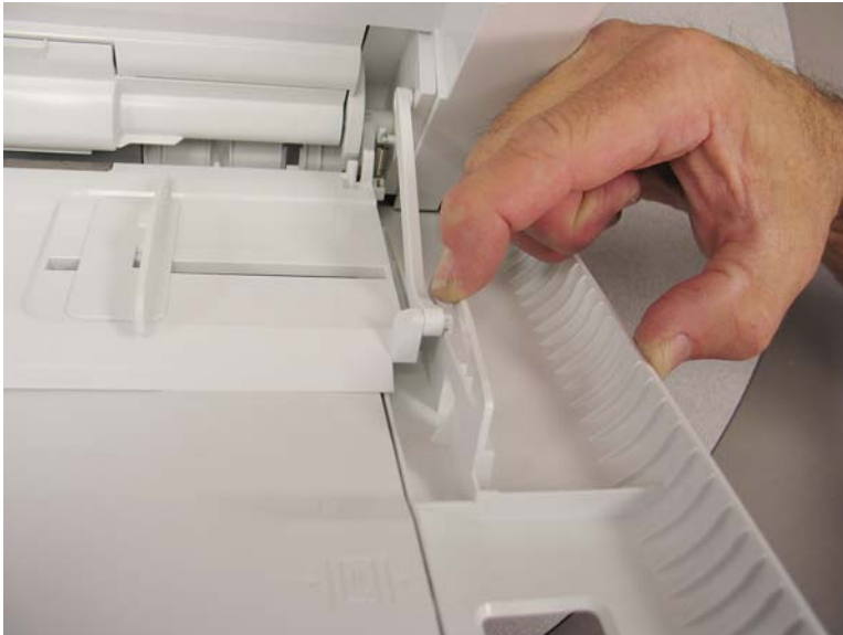
Figure 1-1870 Release the MP tray assembly lift arms from the MP cover
