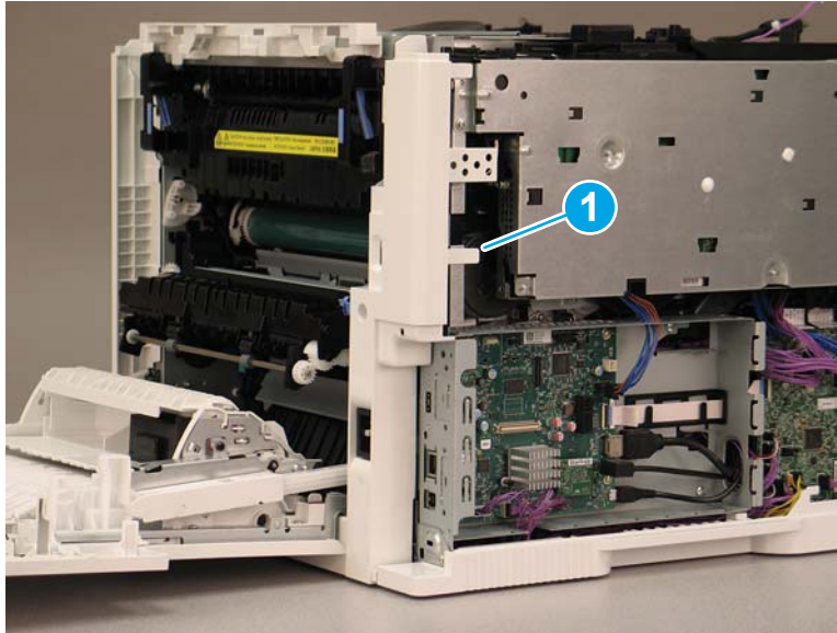
Figure 1-1846 Release the tab and remove the inlet cover
