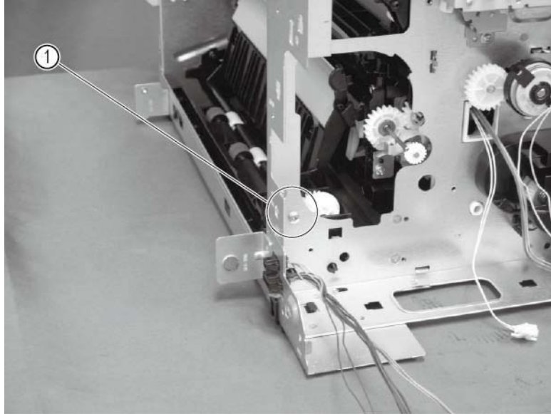
Figure 1-2367 Remove one screw
