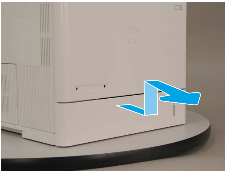
Figure 1-1816 Open and remove the cassette tray 2
