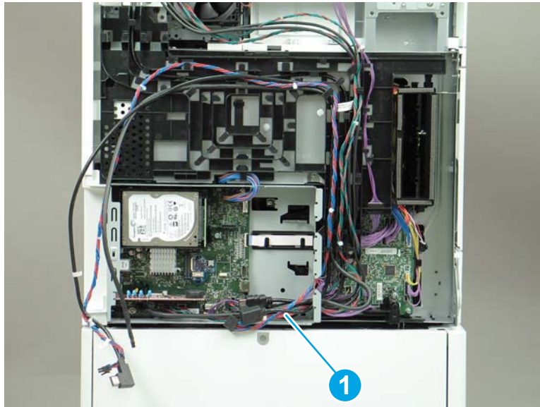
Figure 1-541 Thread the formatter cables through the formatter case
