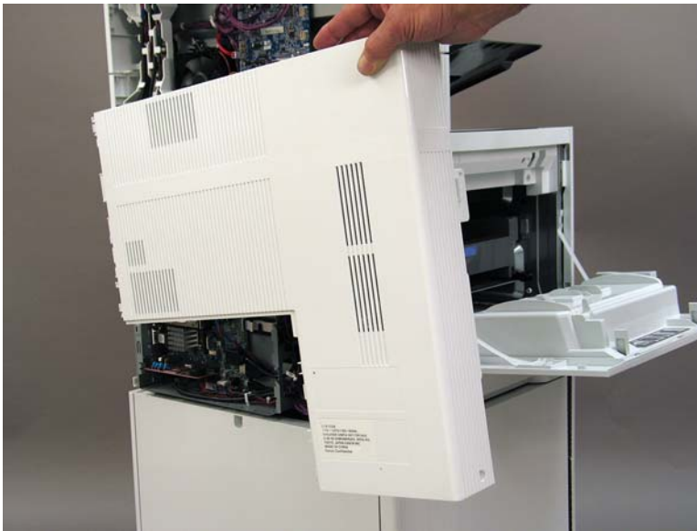
Figure 1-165 Remove the rear cover
