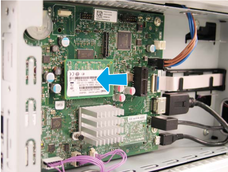
Figure 1-1749 Push the DIMM onto the formatter connector
