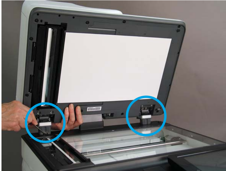
Figure 1-776 Release two tabs on the ADF
