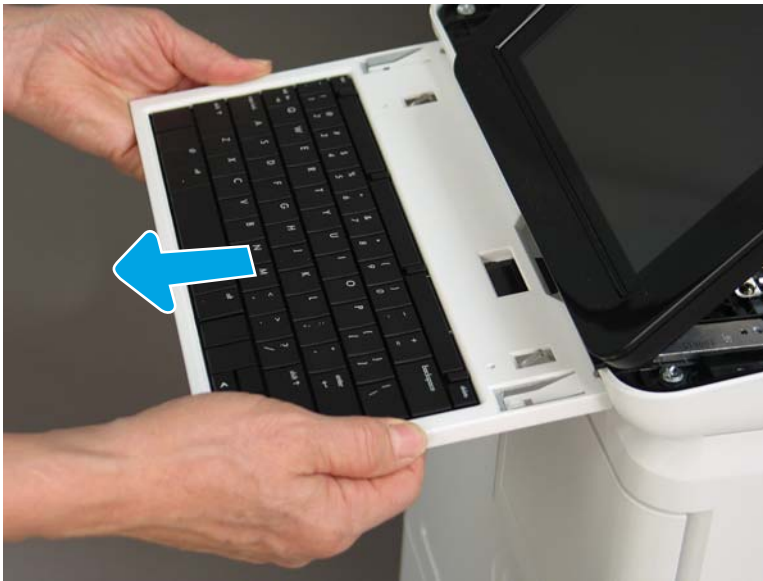
Figure 1-186 Remove the keyboard
