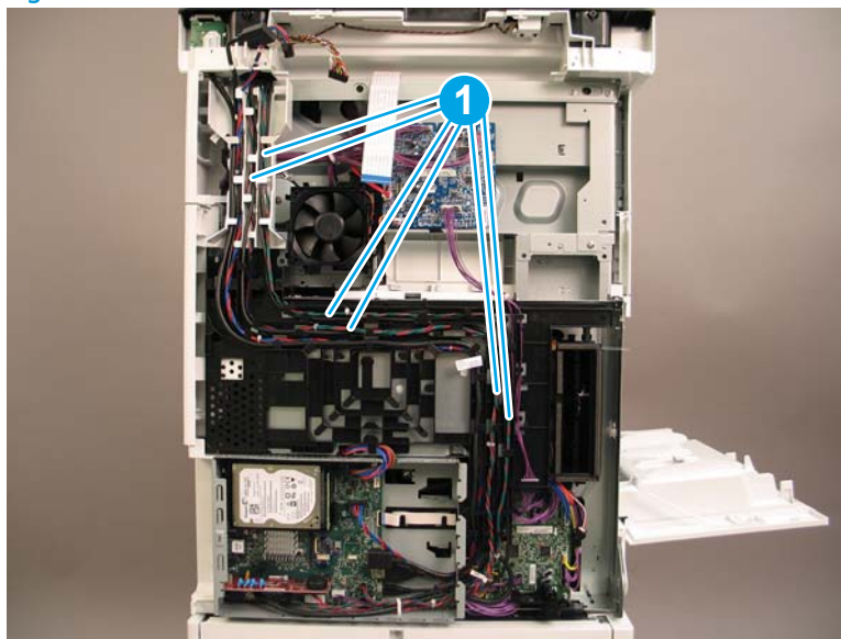
Figure 1-310 Release the formatter cables
