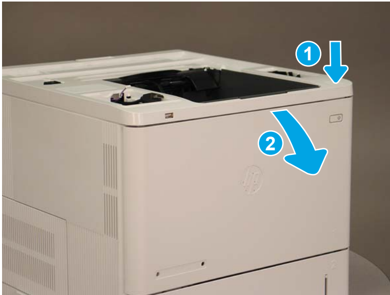
Figure 1-1907 Locate the tab and open the MP tray cover
