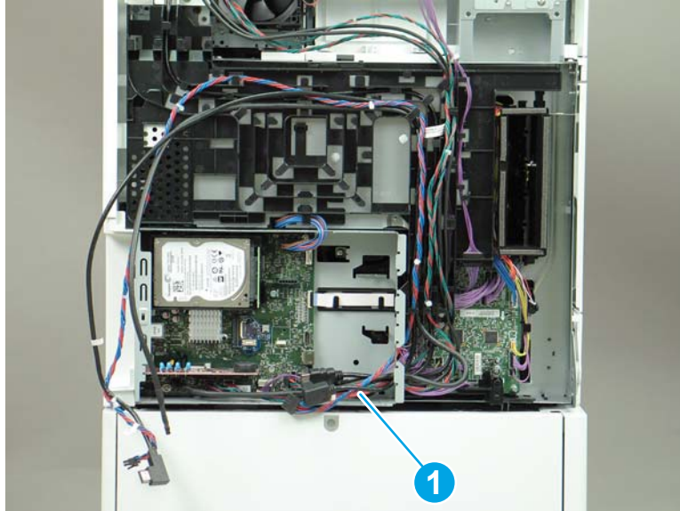
Figure 1-241 Thread the formatter cables through the formatter case
