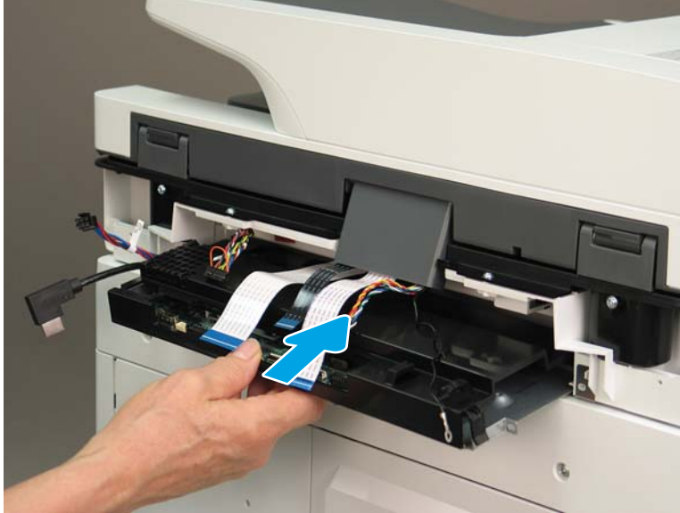
Figure 1-586 Check the cables when installing the SCB
