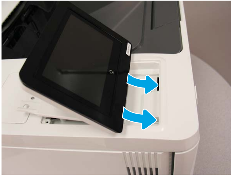
Figure 1-1697 Install the control panel tabs into the printer slots
