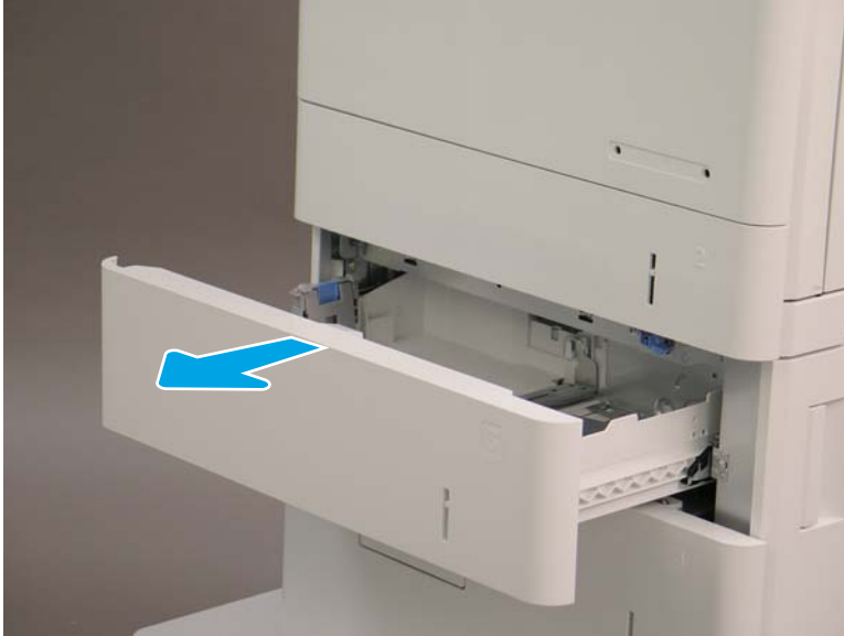
Figure 1-1765 Open the paper tray to locate the rollers
