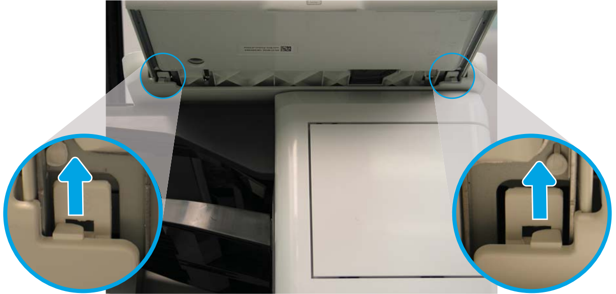
Figure 1-627 Release two tabs
