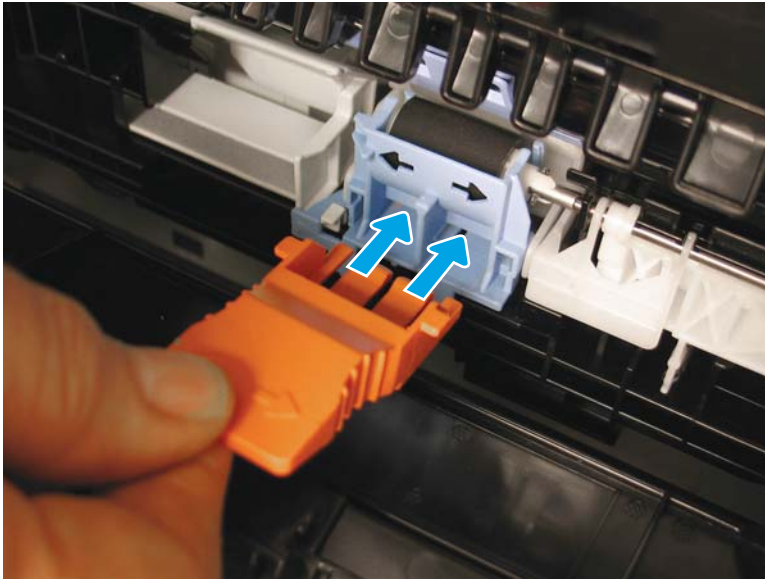
Figure 1-127 Install the orange tool in the separation roller
