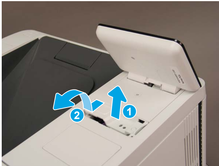
Figure 1-2472 Lift and release the control panel
