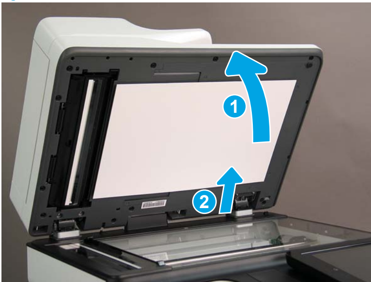
Figure 1-300 Tilt and lift the ADF
