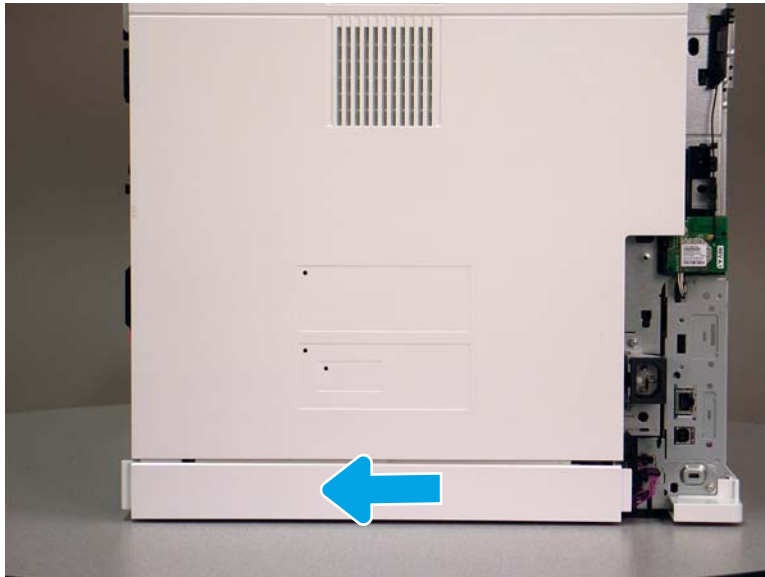
Figure 1-1942 Slide the rear lower cover
