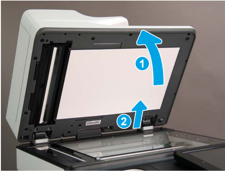
Figure 1-263 Tilt and lift the ADF
