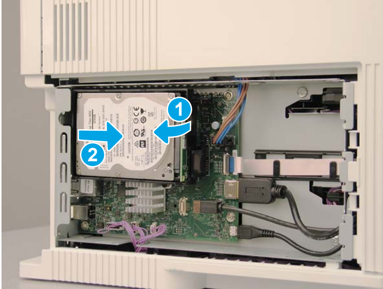
Figure 1-1746 Rotate the HDD away from the formatter and remove the HDD
