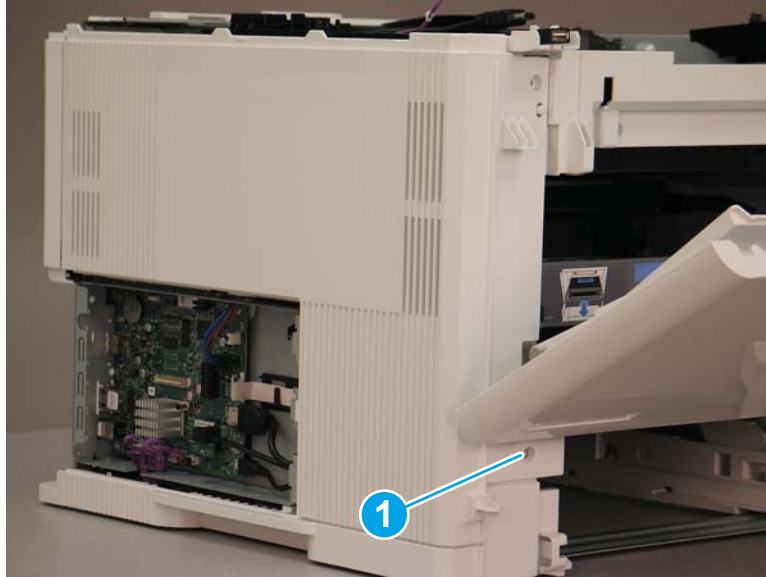
Figure 1-2121 Open the cartridge door and remove one screw
