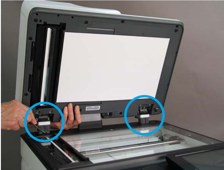
Figure 1-1021 Release two tabs on the ADF
