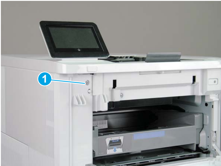
Figure 1-2080 Remove one screw
