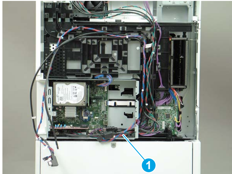
Figure 1-701 Thread the formatter cables through the formatter case
