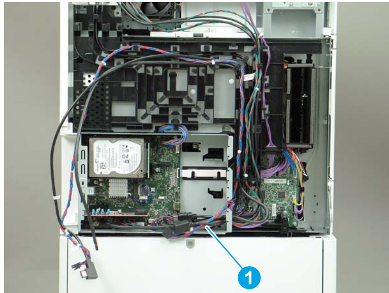
Figure 1-420 Thread the formatter cables through the formatter case
