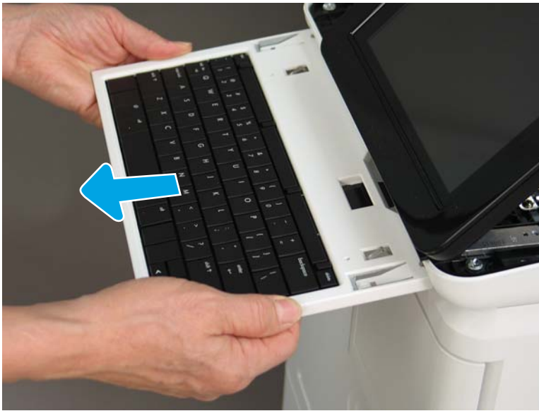
Figure 1-93 Remove the keyboard
