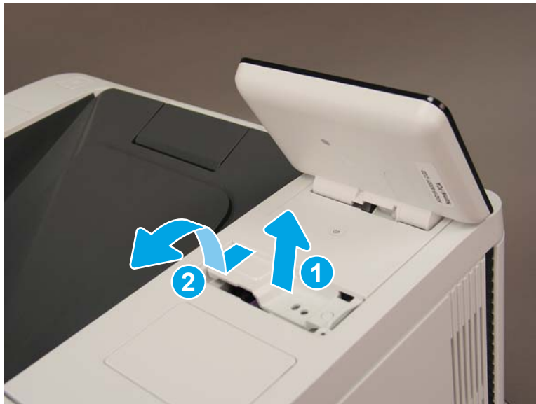
Figure 1-2384 Lift and release the control panel
