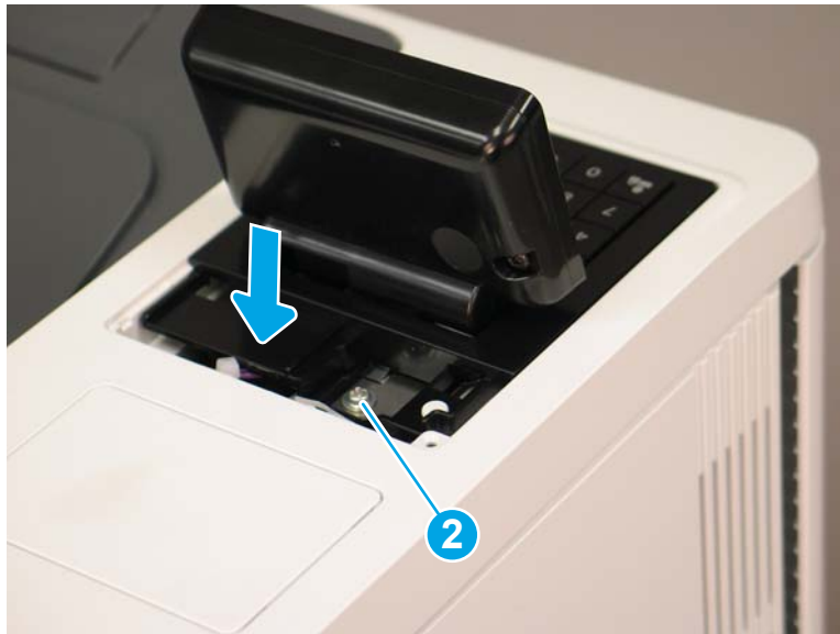
Figure 1-1708 Lower the control panel and install one thumbscrew
