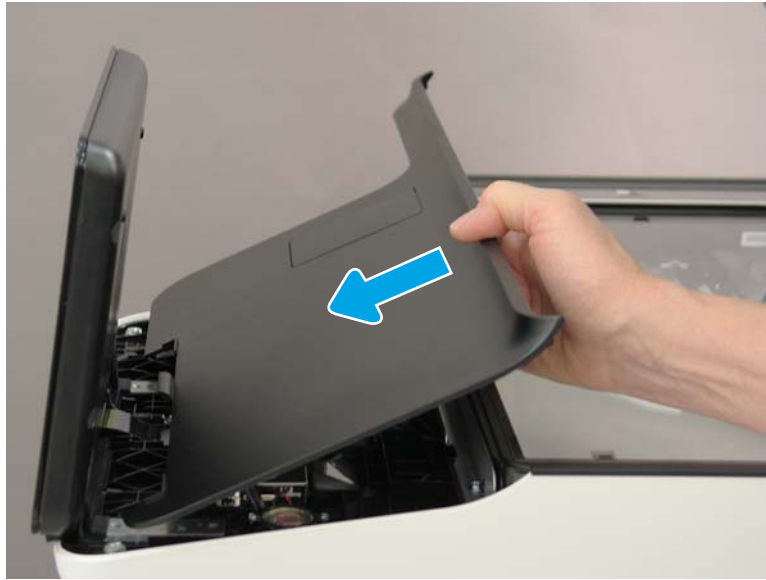
Figure 1-98 Install the cover
