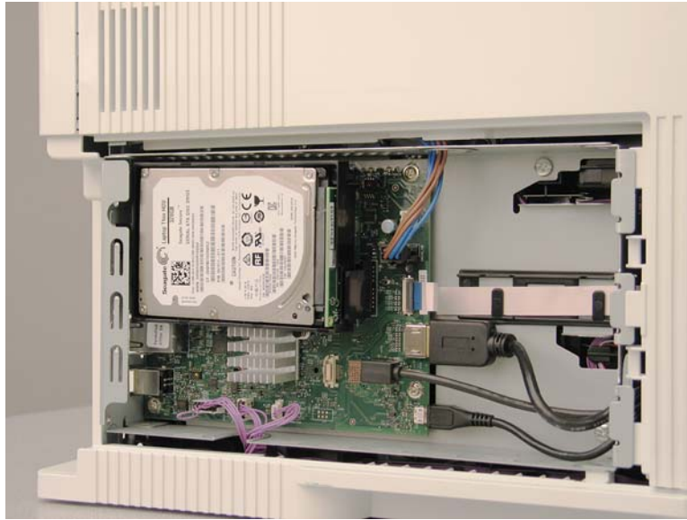
Figure 1-1756 Locate the space for installing the internal USB ports/AA module
