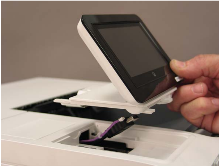
Figure 1-1902 Remove the control panel
