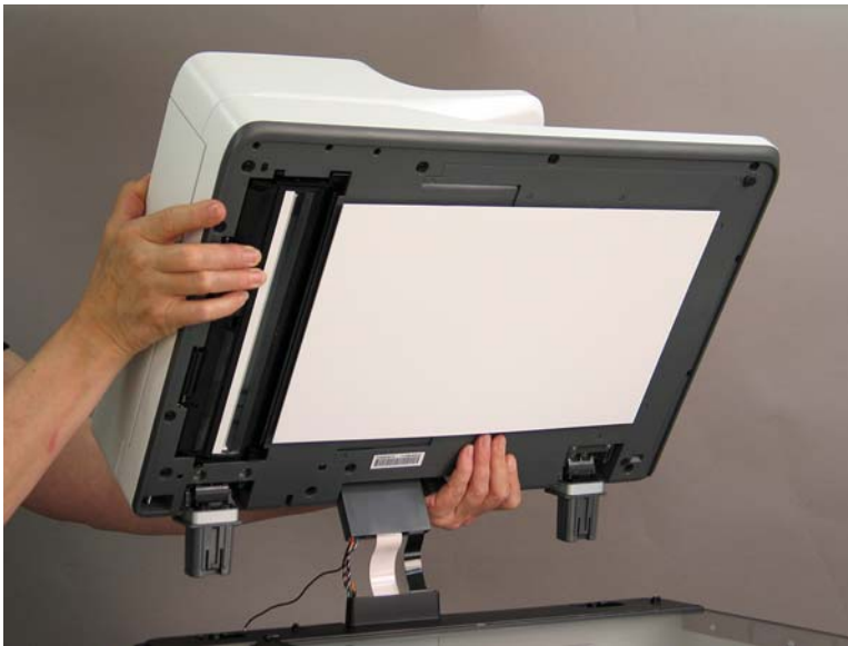
Figure 1-231 Lift and remove the ADF
