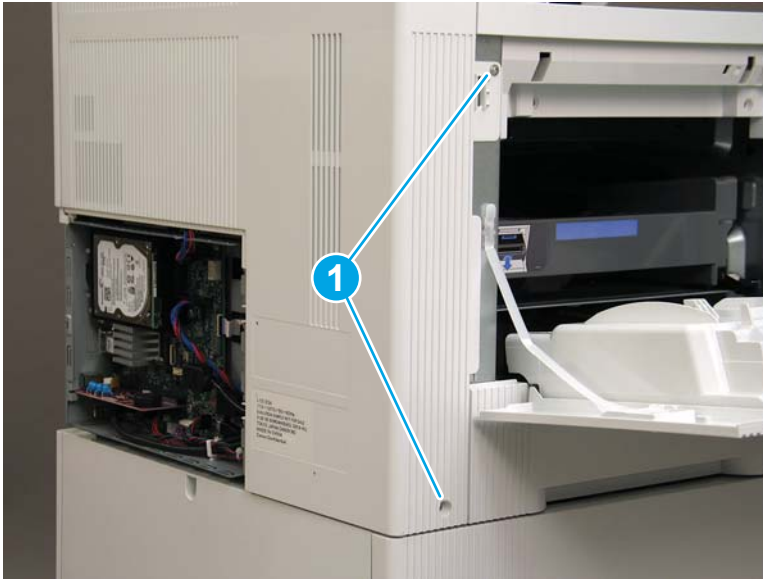
Figure 1-534 Remove two screws
