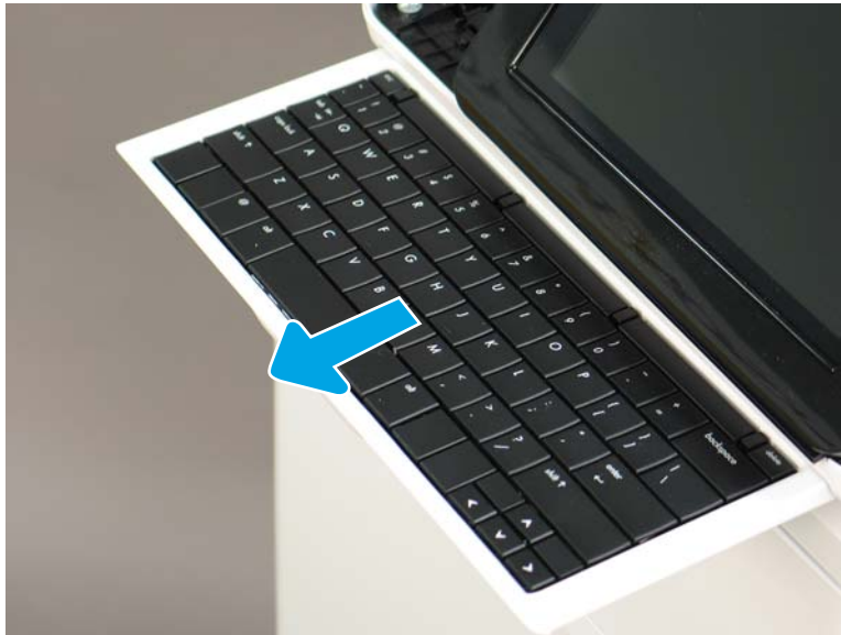
Figure 1-474 Slide the keyboard tray out
