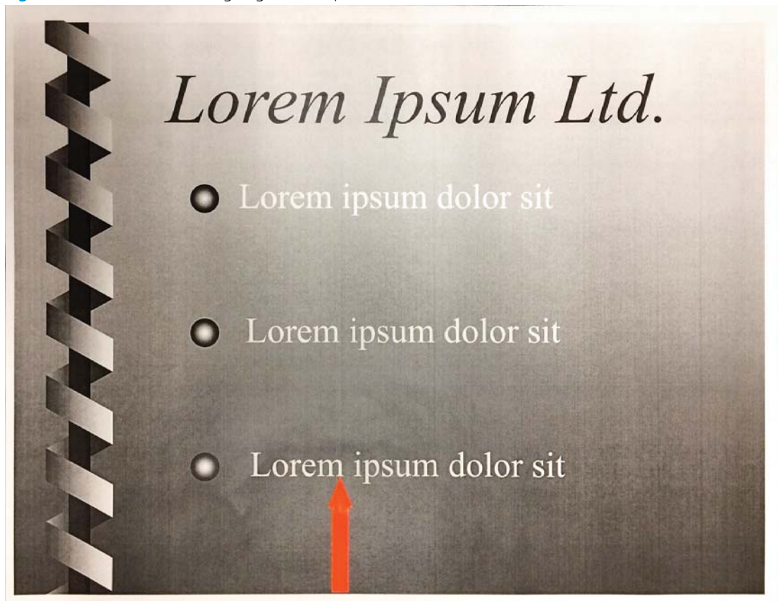
Figure 2-122 120 mm trailing edge blue duplex side
