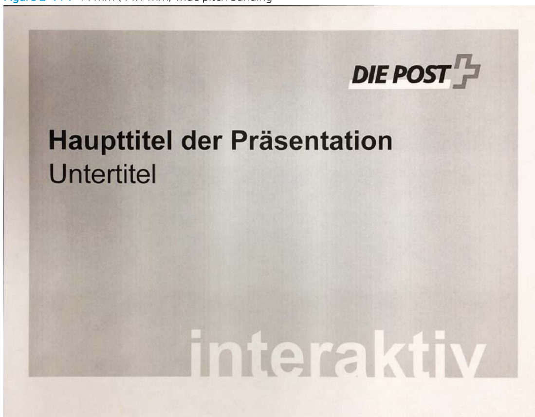
Figure 2-114 44 mm (44.1 mm) wide pitch banding
