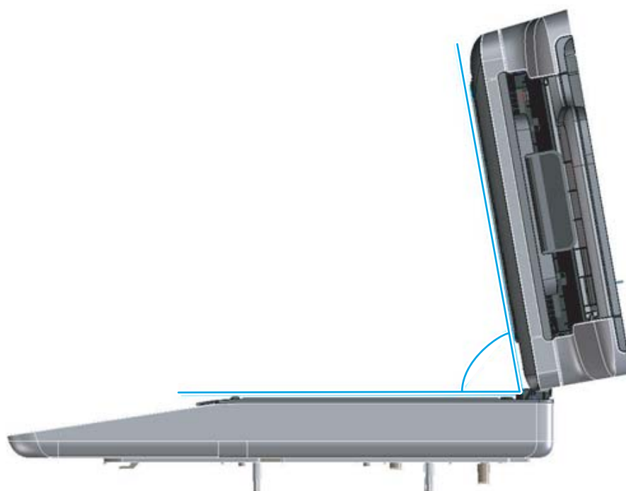
Figure 1-52 Document feeder open (60° to 80°)
