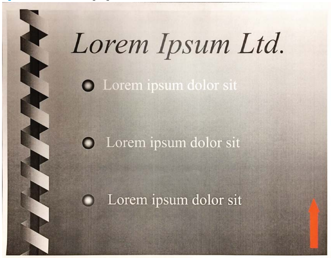
Figure 2-115 18 mm leading edge blur
