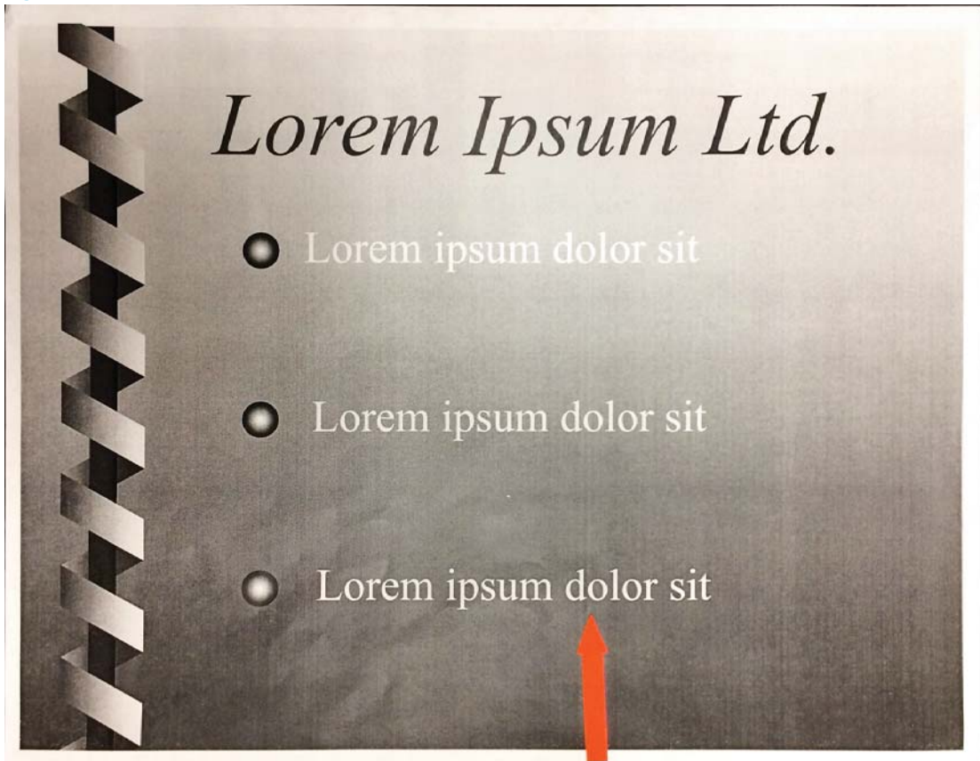
Figure 2-121 111 mm trailing edge blur
