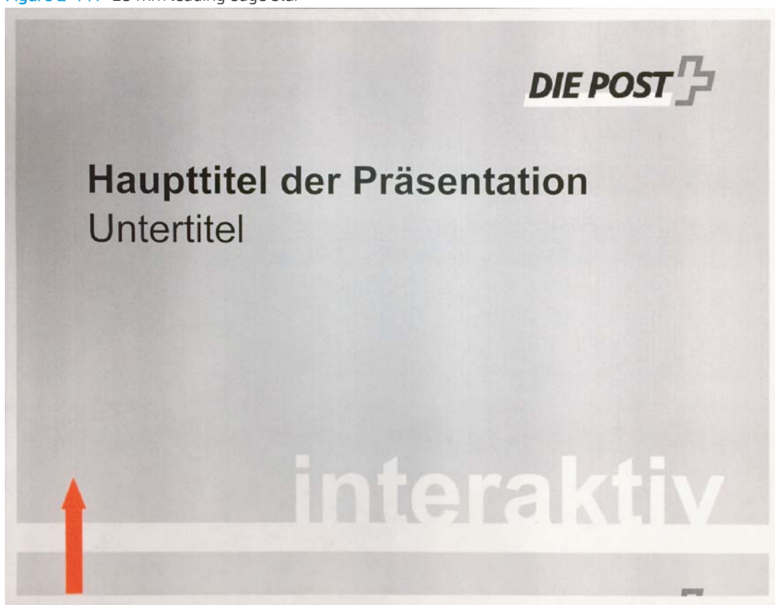
Figure 2-117 25 mm leading edge blur
