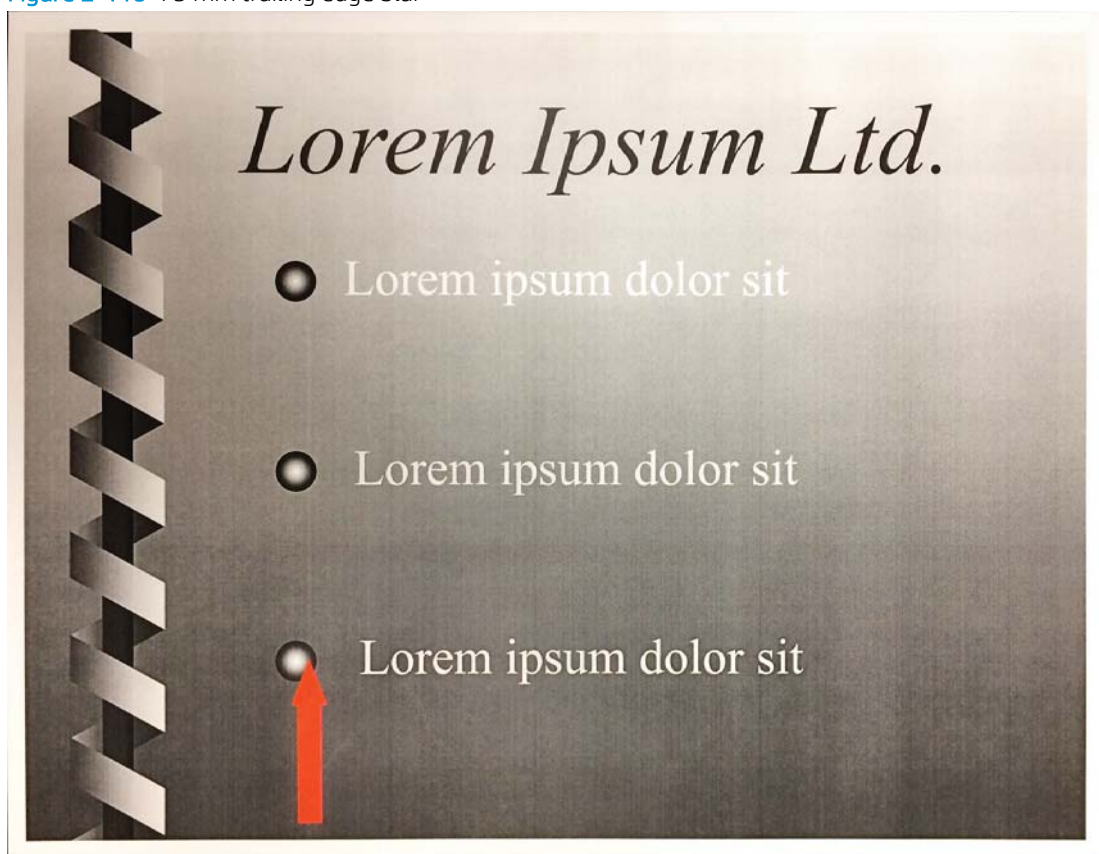
Figure 2-119 75 mm trailing edge blur
