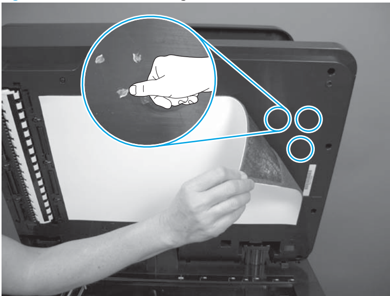
Figure 1-221 Remove remaining adhesive
