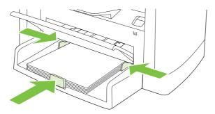
NOTE: When you add new media, make sure that you remove all of the media from the input tray and straighten the stack of new media. Do not fan the media. This reduces jams by preventing multiple sheets of media from feeding through the product at one time.
