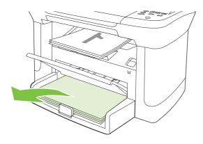
5. Without changing the orientation, remove the printed stack from the output bin, and then straighten the stack.
