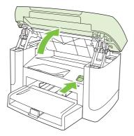
2. Grasp the handle on the print cartridge and then pull the cartridge straight out to remove it. See the recycling information inside the print cartridge box.
