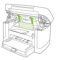
3. Replace the print cartridge and close the print-cartridge door.
