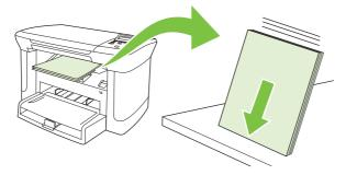
6. Maintaining the same orientation, place the stack of media in the input tray again. The printed side should be facing down with the top edge feeding into the product first.
