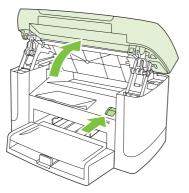
2. Grasp the handle on the print cartridge, and then pull the cartridge straight out to remove it.
