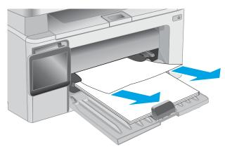
Remove any jammed paper from the toner-cartridge area. Use both hands to remove jammed paper to avoid tearing the paper.
