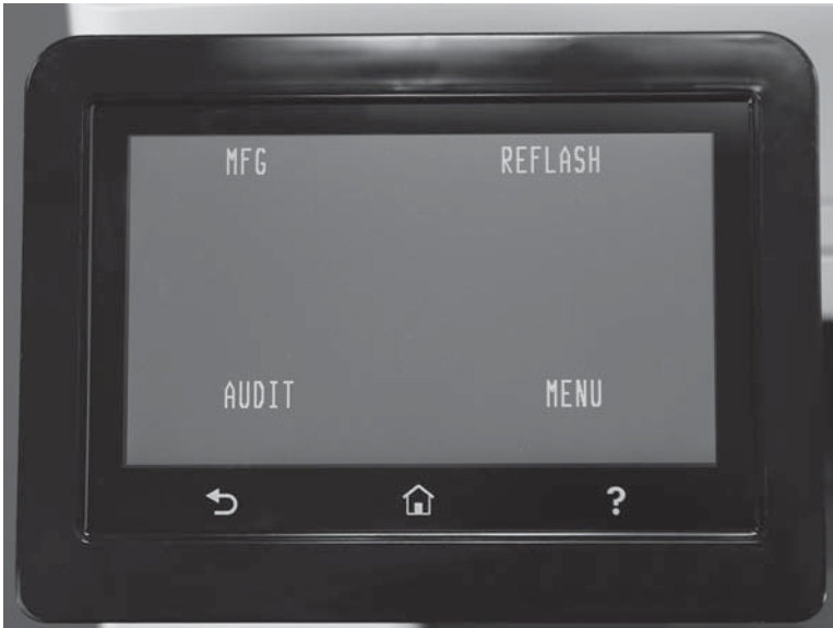
Figure 2-23 Touchscreen control panels boot screen
