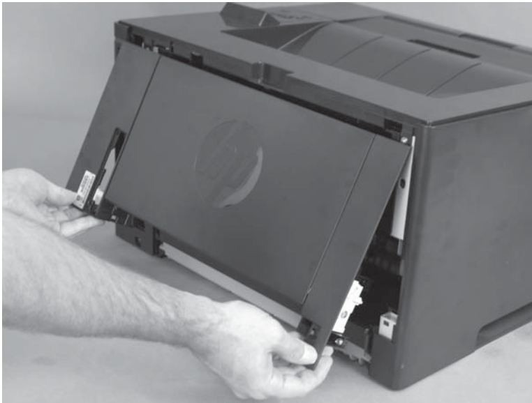
Figure 1-26 Remove the rear-cover assembly (2 of 2)
