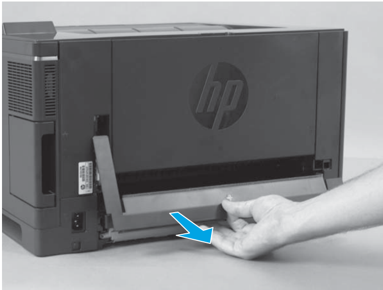
Figure 1-24 Remove the lower back cover
