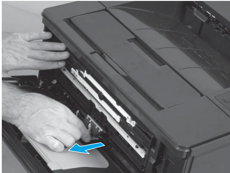
Figure 1-9 Remove the Tray 1 separation pad (4 of 4)
