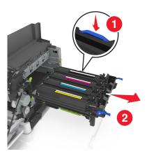
**8** Remove the used developer unit.
