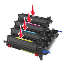
13 Remove the red packing strip from the imaging kit.
