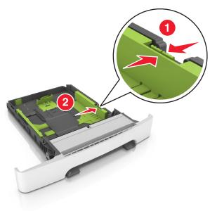
Note: Use the paper size indicators on the bottom of the tray to help position the guides.
