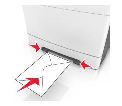
**2** Feed paper into the manual feeder only to the point where its leading edge can contact the paper guides.
