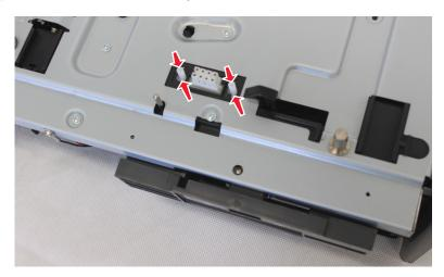
Squeeze, and then push the latches into the tray base to release the cable.
