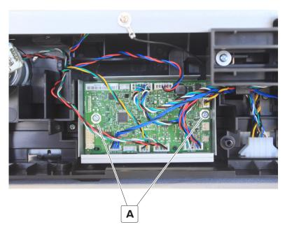
Remove the controller board assembly.
