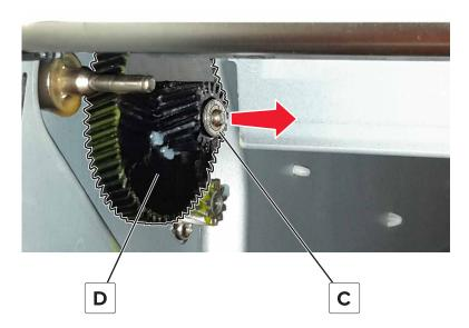
Installation note: Use the washer in the new gear.
