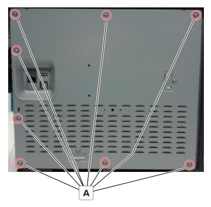
2 Remove the controller board shield.
