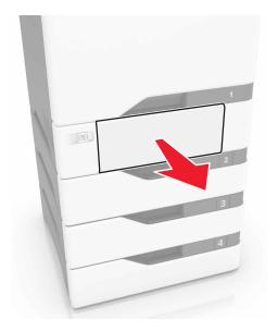
**Warning—Potential Damage:** A sensor inside the optional tray is easily damaged by static electricity. Touch a metal surface before removing the jammed paper in the tray.
