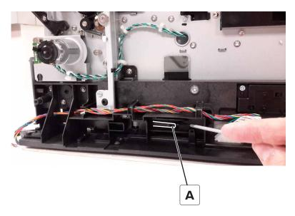
**6** Hold the tab in place, and then slide the rail toward the front of the printer to remove.
