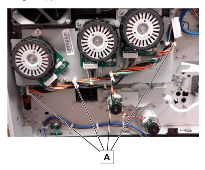
Disconnect the three motor cables (B).
