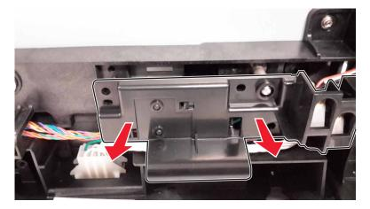
Disconnect the sensor cable (B).
