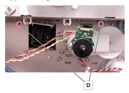
**6** Remove the two screws (E) from the top-left and top-right corners of the EP drive, and then remove the gear box.
