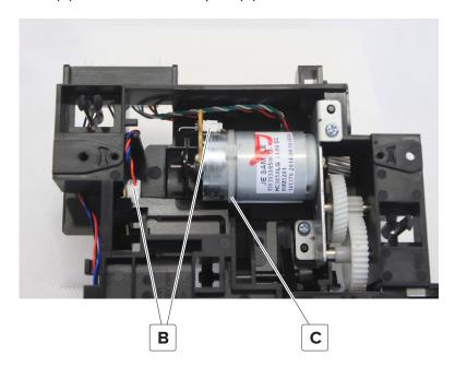
Squeeze, and then push the latches into the tray base to release the cable.
