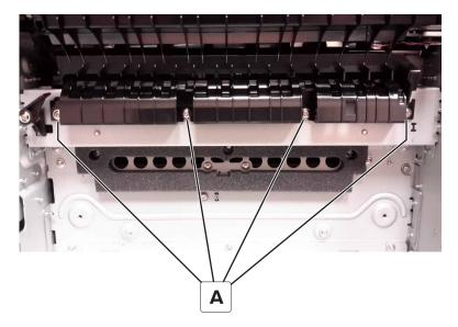
**3** Hold the redrive deflector up, and then remove the redrive guide.
