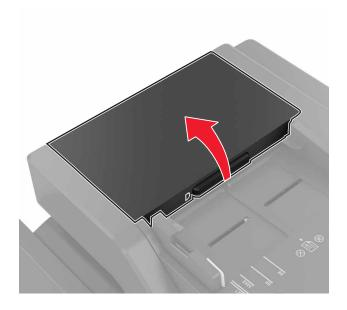
**3** Remove the ADF separator roller cover.
